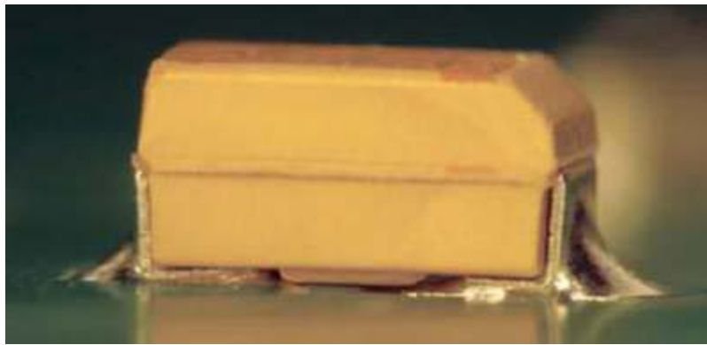
Figure 16-23: Acceptable, preferred solder joint
