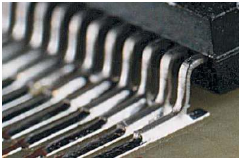
Figure 16-13: Examples of Gullwing leads: Acceptable
