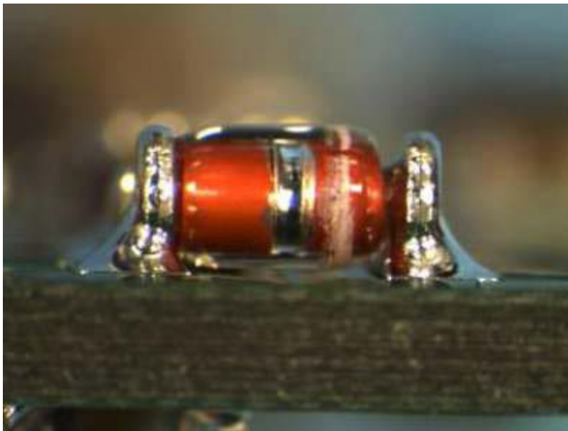
Figure 16-10: Acceptable maximum solder joint (see also Table 11-3)
