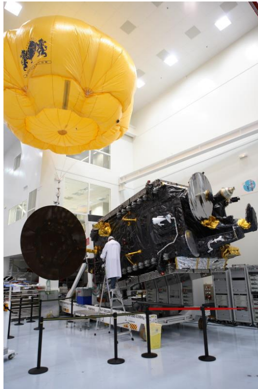
Figure 13-11: Example of release of reflectors
