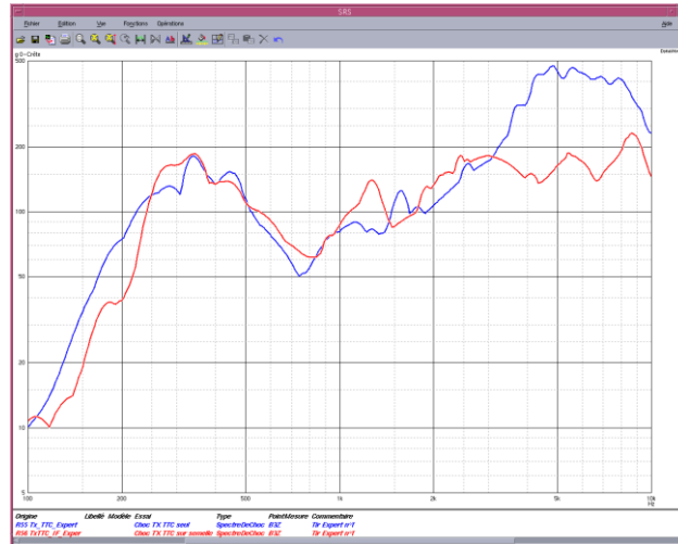
Figure 13-72: Top unit responses (X, Y, Z) with and without the load cells at the interface
