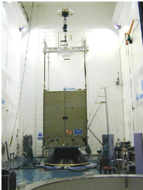
Figure 13-1: Examples of system test configuration and boundary conditions (clampband release on the left and Ariane 5 VEB separation on the right)
