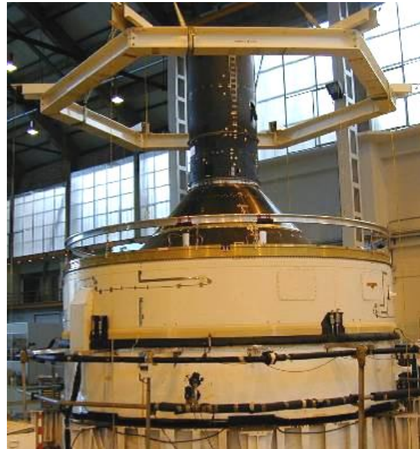
Figure 13-1: Examples of system test configuration and boundary conditions (clampband release on the left and Ariane 5 VEB separation on the right)
