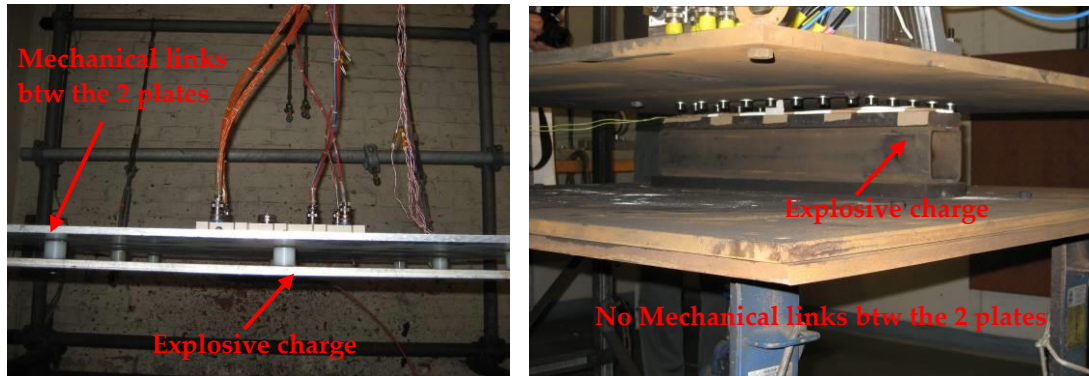
Figure 13-16: Excitation through direct contact (left) and pressure shock wave (right)
