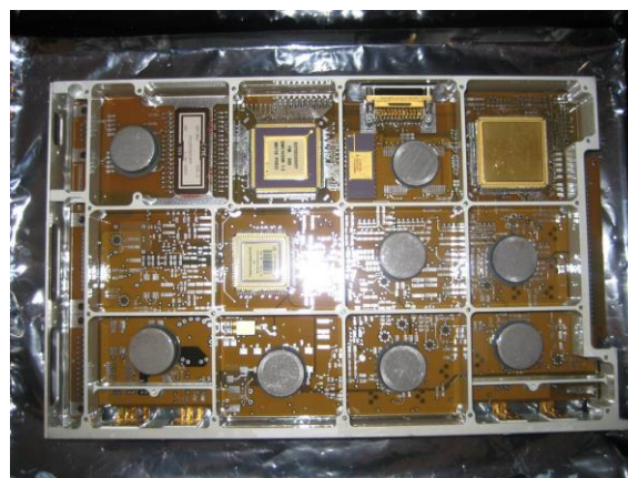
Figure 18-24: Module with critical components
