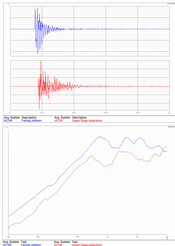
Figure 13-99: Example of UCTM shock measures with correct full scale value and relevant SRS
