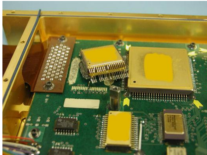
Figure 18-41: Pulled out component after a stringent shock test
