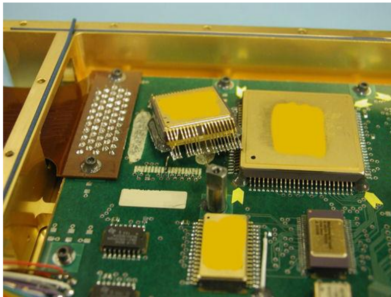
Figure 17-34: Adhesive failure and rupture of solder joint after a stringent shock test
