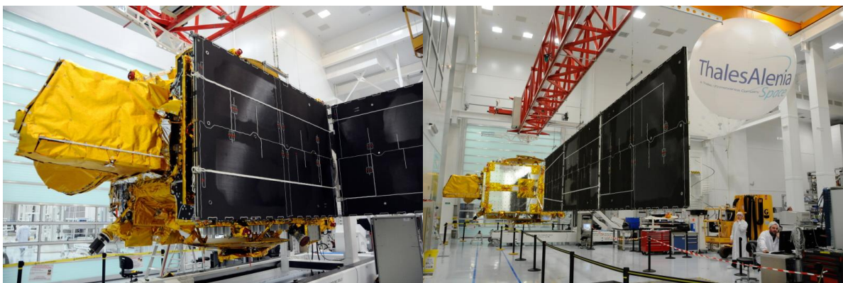
Figure 13-10: Example of release of solar arrays (left: intermediate position; right: final position)
