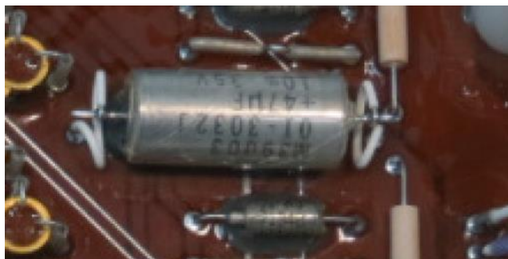
Figure 17-33: Heavy/large tantalum capacitor (secured with adhesive compound and with provision for stress relief)
