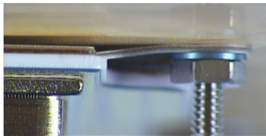
Figure 17-30: Deformed hybrid interface plate
