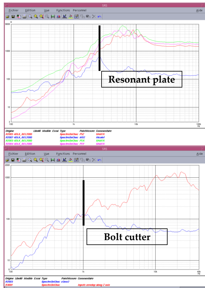
Figure 18-15: Equipment transition frequency (on a PCB) in various shock environments
