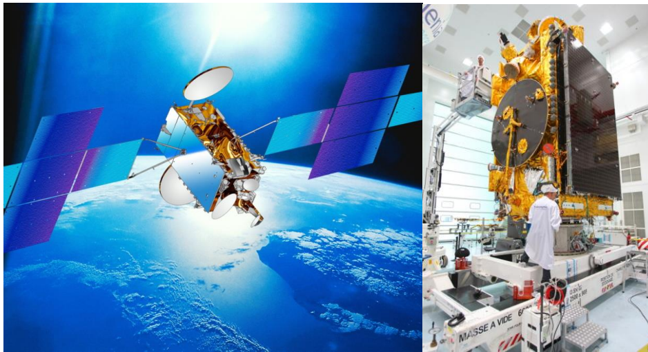
Figure 13-9: Example of a telecommunication spacecraft with deployed and stowed appendages (solar arrays and reflectors)
