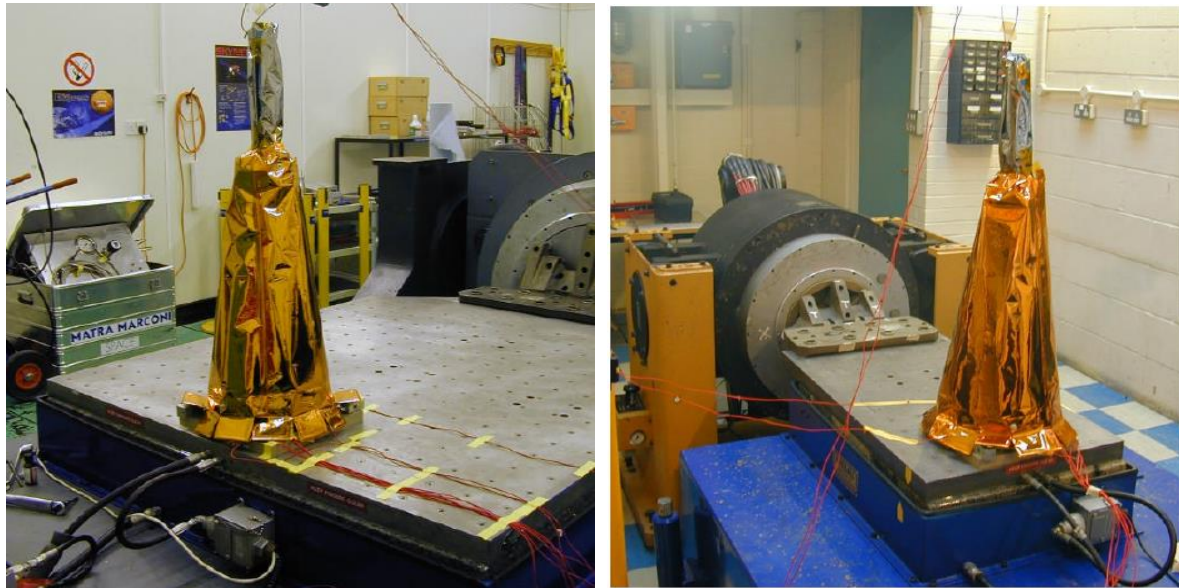
Figure 13-43: Metop DTA Lateral Test on the Ling C340 (left) and on the Ling V954 (right)
