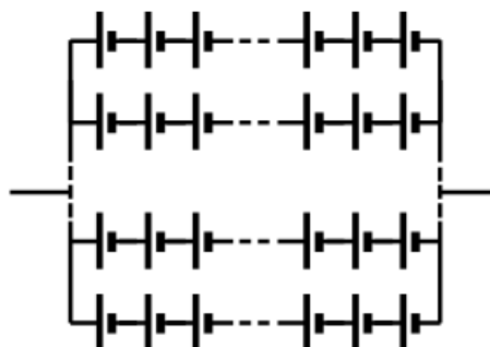
Figure 4-3: A module made of cells connected in series and parallel ( n s m p module)
