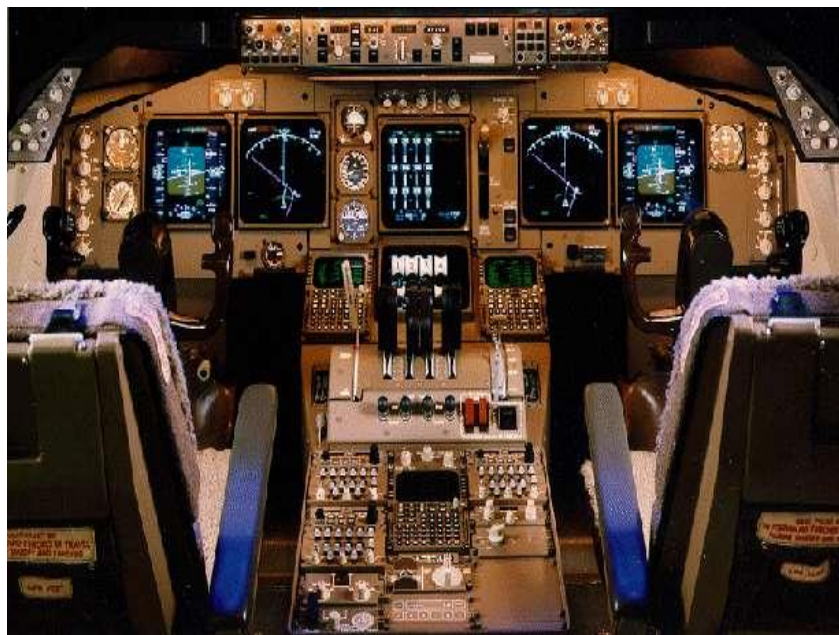
Figure 5-9. Example of a computer-based, concentrated user interface – the glass cockpit (transition to glass cockpit for the Boeing 747)
