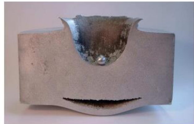
Al sphere, 12 mm diameter, Impact velocity: 6.8 km/s
