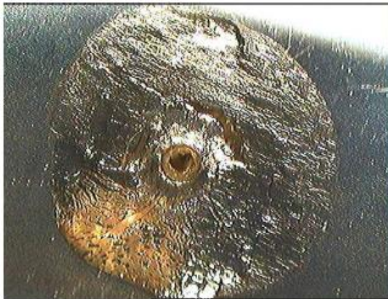
Impact on HST MLI Outer damage size: 5 mm; Hole size: 464 \mu\text{m}
