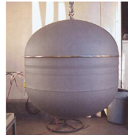
Hydrazine tank used on USA-193
