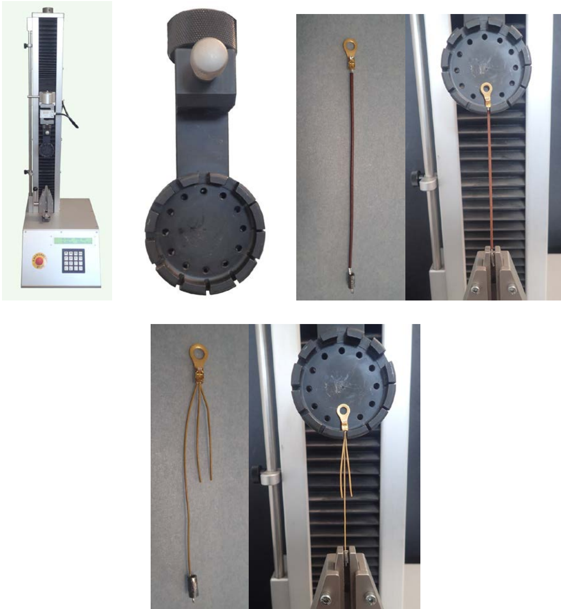
Figure A-6: Typical test fixture for testing lug and splice crimps
