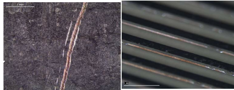
Figure 10-64: Example of visible copper on top surface (left) and on side of track (right)
