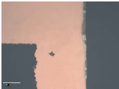
Figure 10-33: Example of voids – top image shows etch-out and bottom image shows an encapsulated void or inclusion
