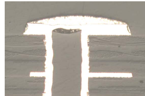
Figure 10-30: example of non-acceptable bulging
