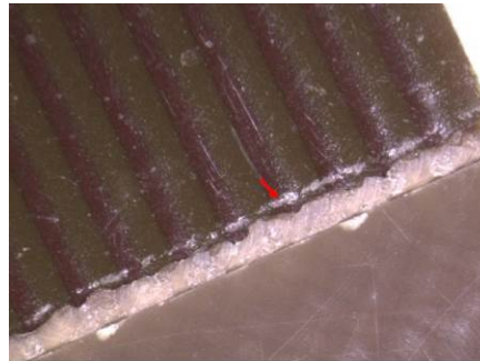
Figure 10-78: Example of an acceptable superficial scratch
