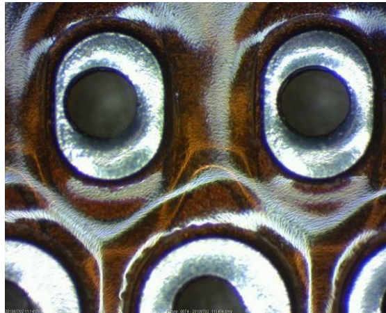
Figure 10-94: Hole misregistration causing reduced annular ring
