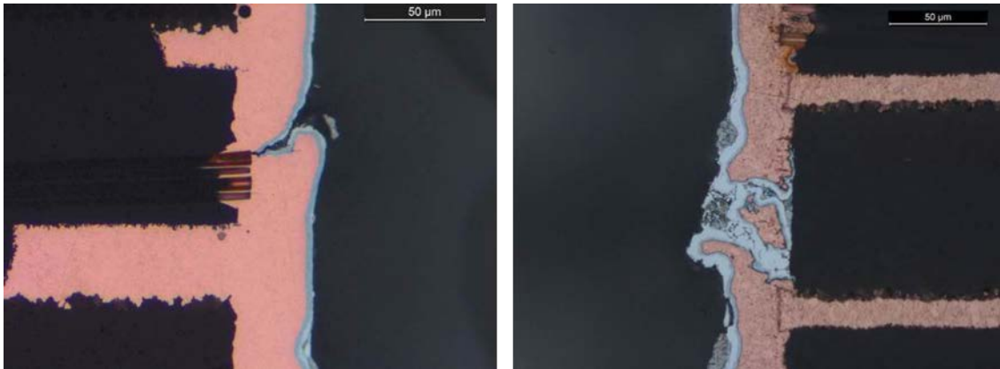
Figure 9-9: Examples of barrel cracks after IST testing showing a nominal crack size (left) and a large crack filled with SnPb (right)
