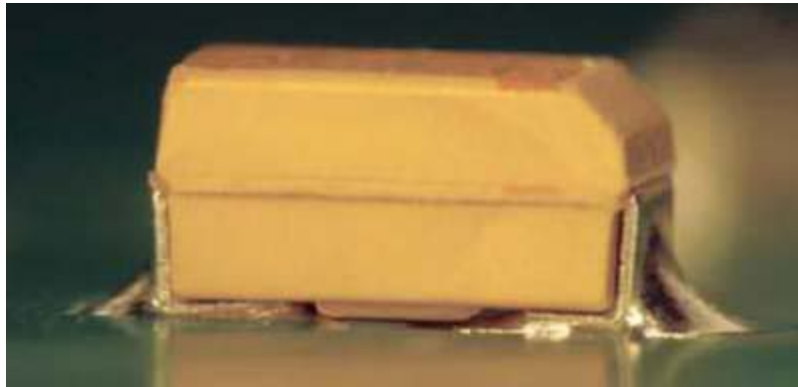
Figure I-23: Acceptable, preferred solder joint
