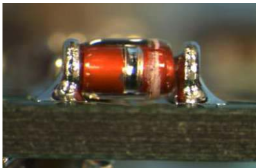
Figure I-10: Acceptable, maximum solder joint (see also Table 11-3)
