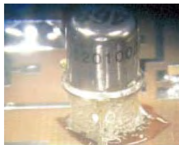
Figure 8-2: Staking of TO package with underfill
