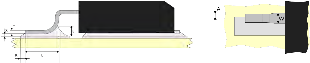
Figure 10-12: Mounting of leaded components with leads with plane termination
