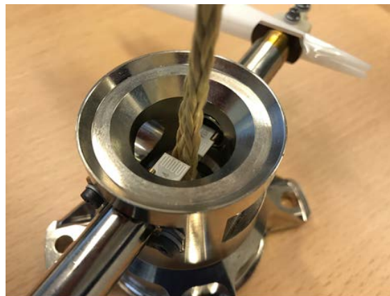
Figure 5-5: Thermal knife (with thermal heads visible)
