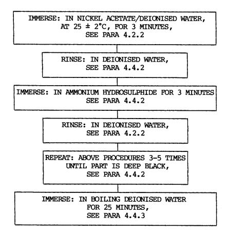
FLOW DIAGRAM OF DYEING PROCESSES
