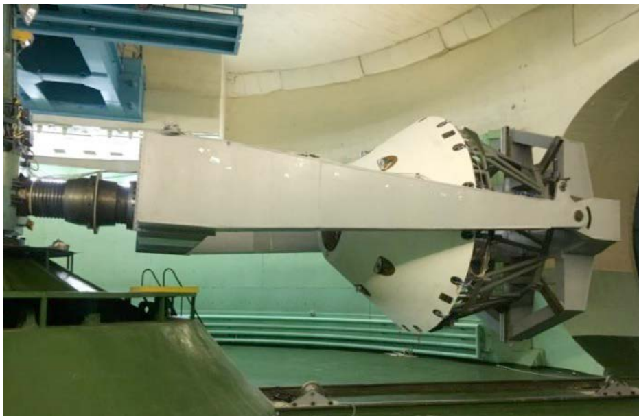
Figure A-21: Centrifuge test of ExoMars Descent Module (courtesy of Lavoshkin)
