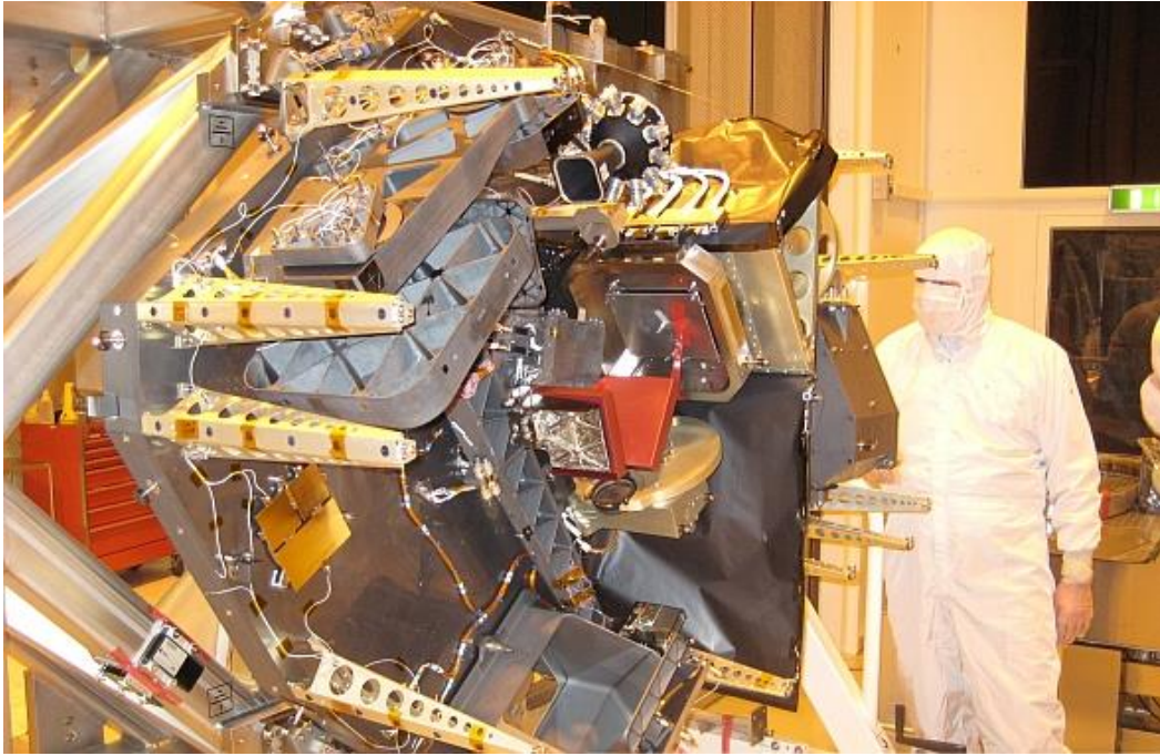
Figure A-34: NIRSpec engineering test unit (ETU) during gravity-release test (courtesy: EADS Astrium)
