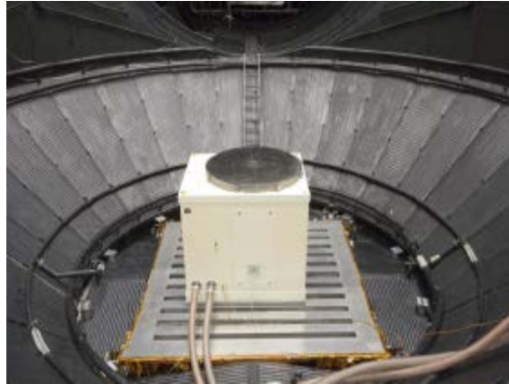
Figure A-18: Dynamic balancing facility installed in a vacuum chamber (Large Space Simulator at ESTEC)
