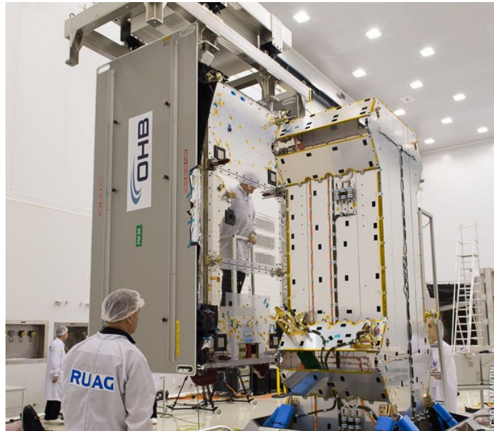
Figure 6-9: Fit check of Galileo Spacecraft with the launch dispenser
