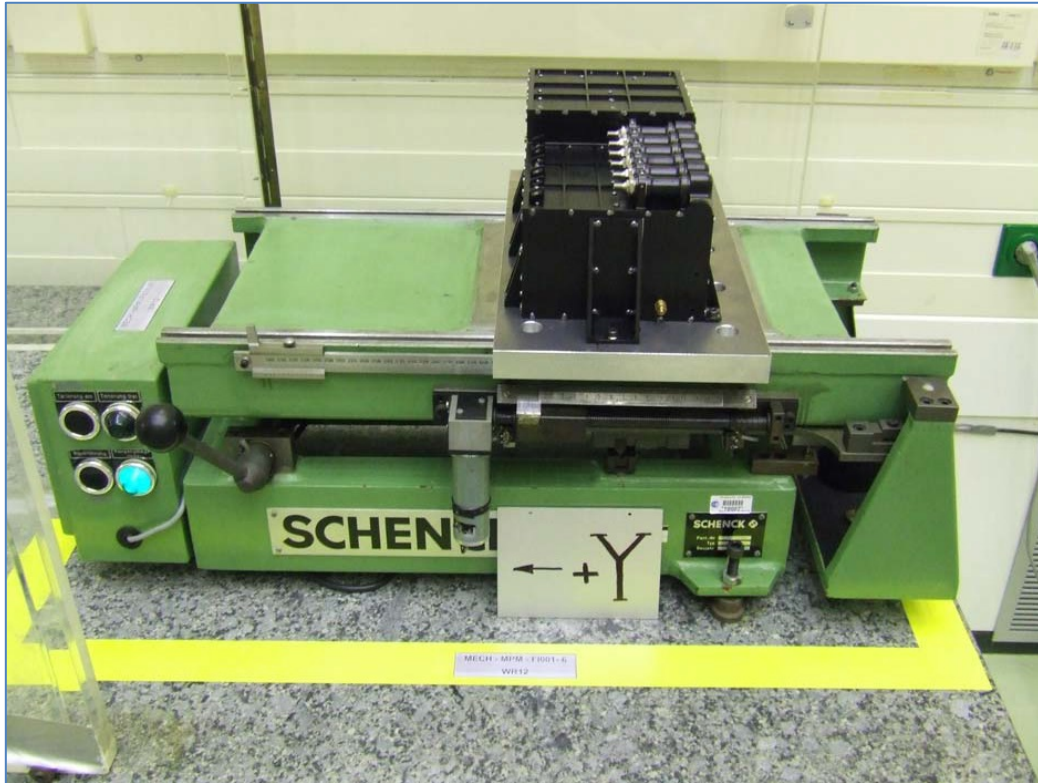
Figure A-2: CoG measurement along 2nd lateral axis
