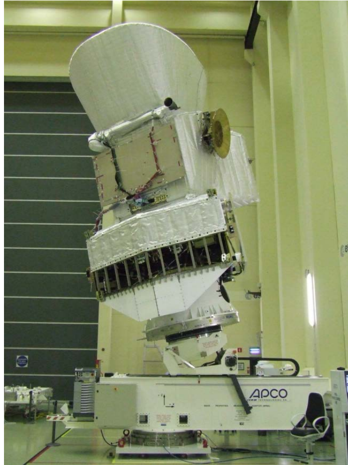
Figure A-4: M80 physical properties measurement machine with Bepi-Colombo MCS at ESTEC
