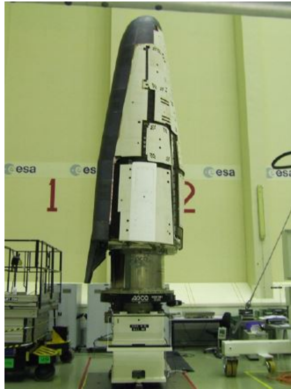
Figure A-5: WM50/6 combined CoG and MoI measurement machine with IXV STM
