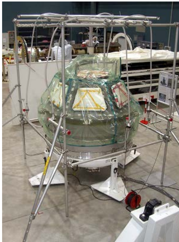
Figure B-4: Cupola Accumulation leak test overview
