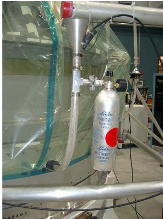
Figure B-5: Cupola Accumulation Leak Test He capillary leak source
