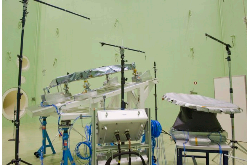
Figure A-26 Antenna reflector acoustic test in ESTEC acoustic facility
