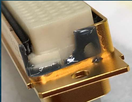
Wrong connector selection and "repair"
