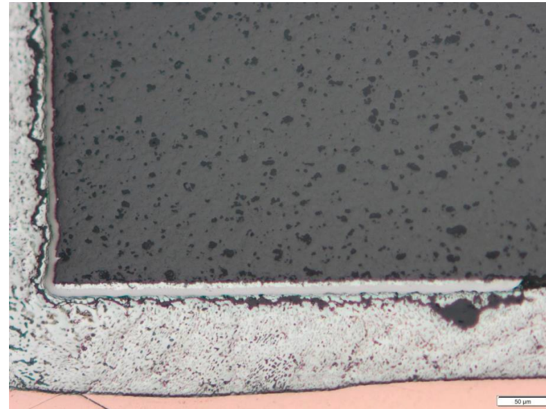
Crack in solder joint
