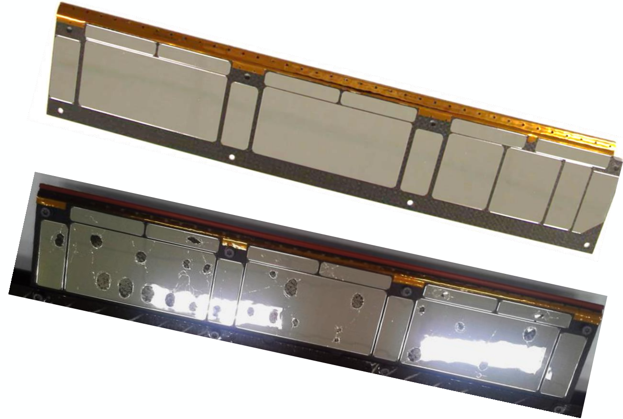
Fracture of glass solar reflectors during thermal vacuum cycling
