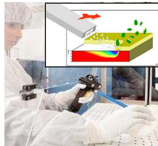
CO 2 spray cleaning
