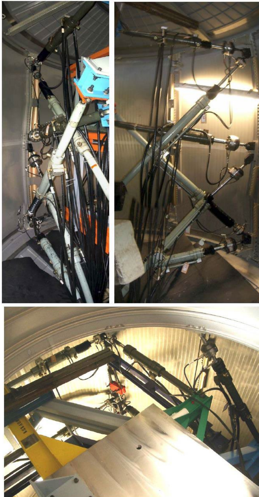
Figure A-15: ATV static test: internal loading jacks details
