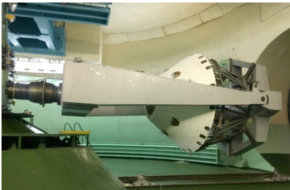
Figure A-21: Centrifuge test of ExoMars Descent Module (courtesy of Lavoshkin)
