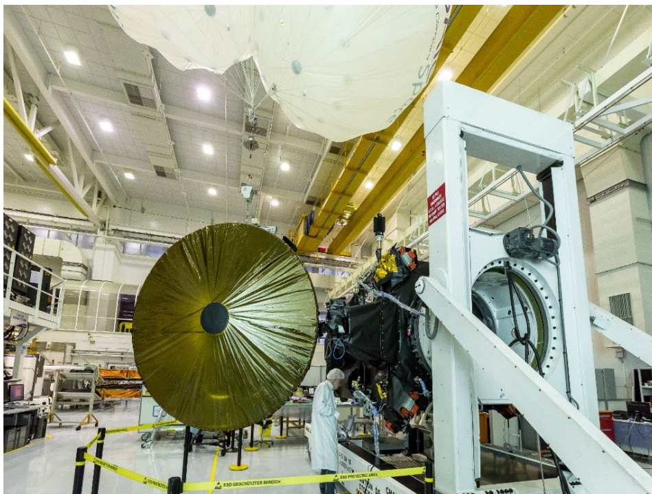
Figure 6-7: Exomars TGO antenna offloading device
