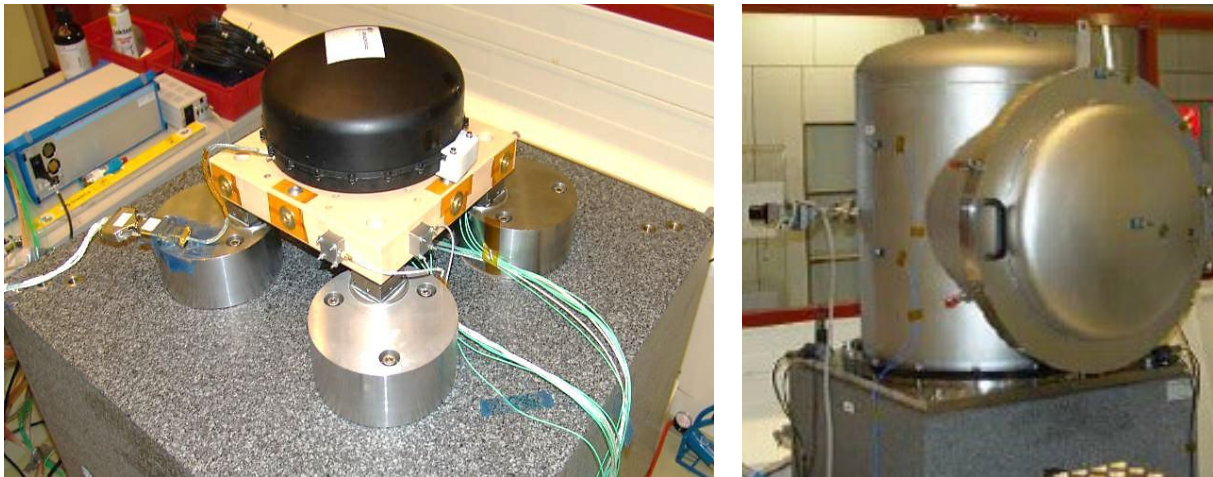
Figure A-39: ESA reaction wheel characterisation facility in room conditions and in with vacuum bell (mN range frequency band up to 1 kHz )
