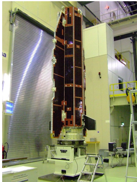
Figure A-6: WM50/6 combined CoG and MoI measurement machine with Goce PFM
