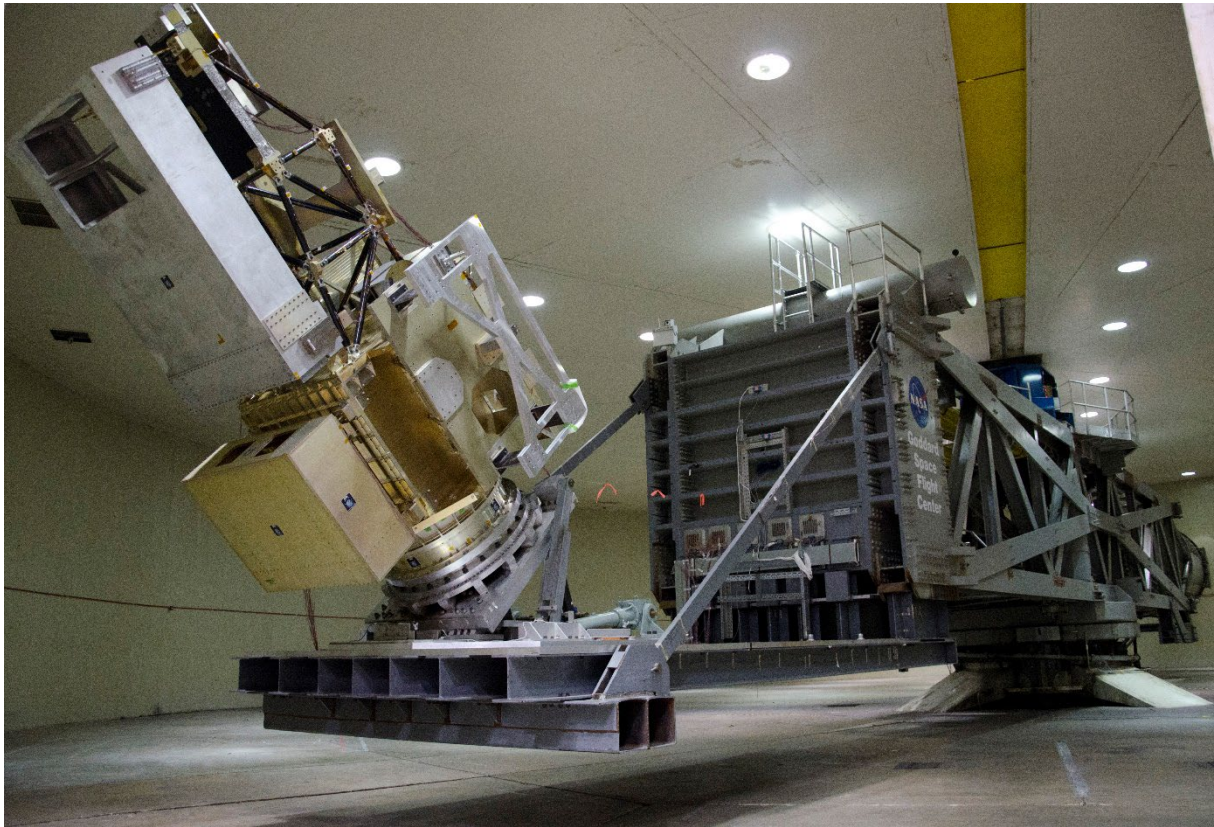
Figure A-20: GPM spacecraft undertakes centrifuge test at Goddard (courtesy of NASA)
