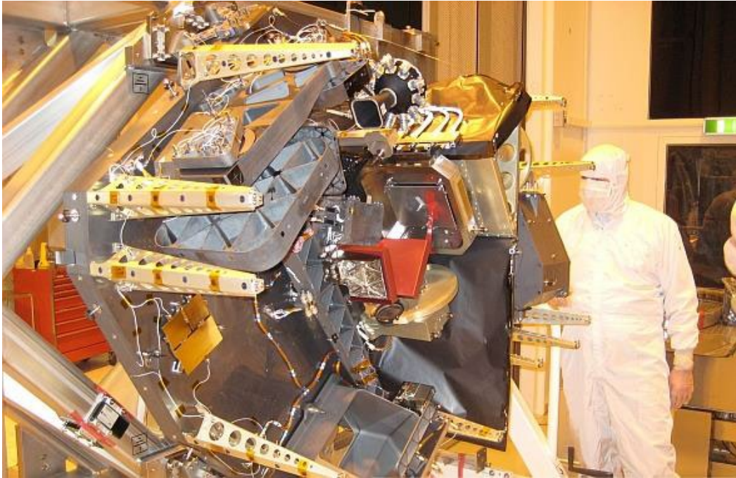
Figure A-37: NIRSpec engineering test unit (ETU) during gravity-release test (courtesy: EADS Astrium)
