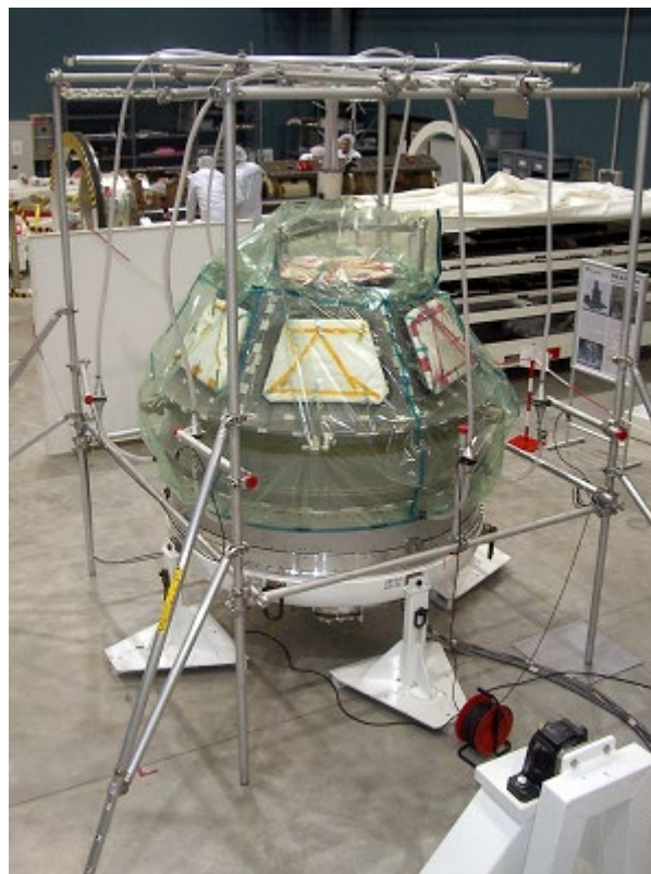
Figure B-4: Cupola Accumulation leak test overview
