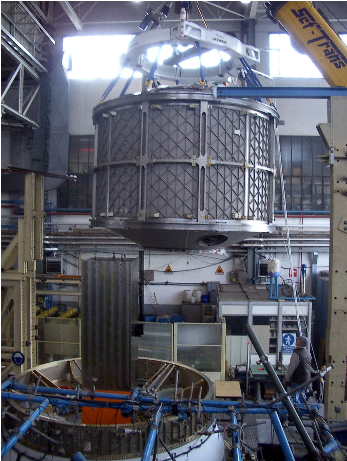
Figure A-12: Setting of ATV primary structure static test
