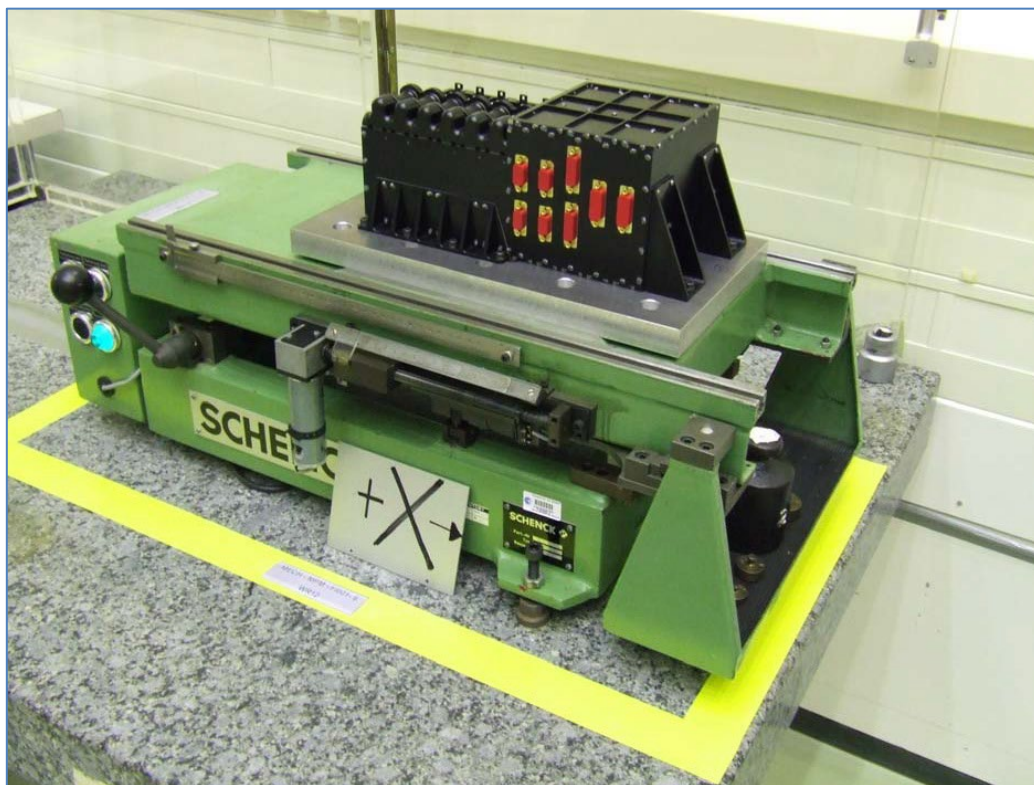
Figure A-1: CoG measurement along 1st lateral axis
