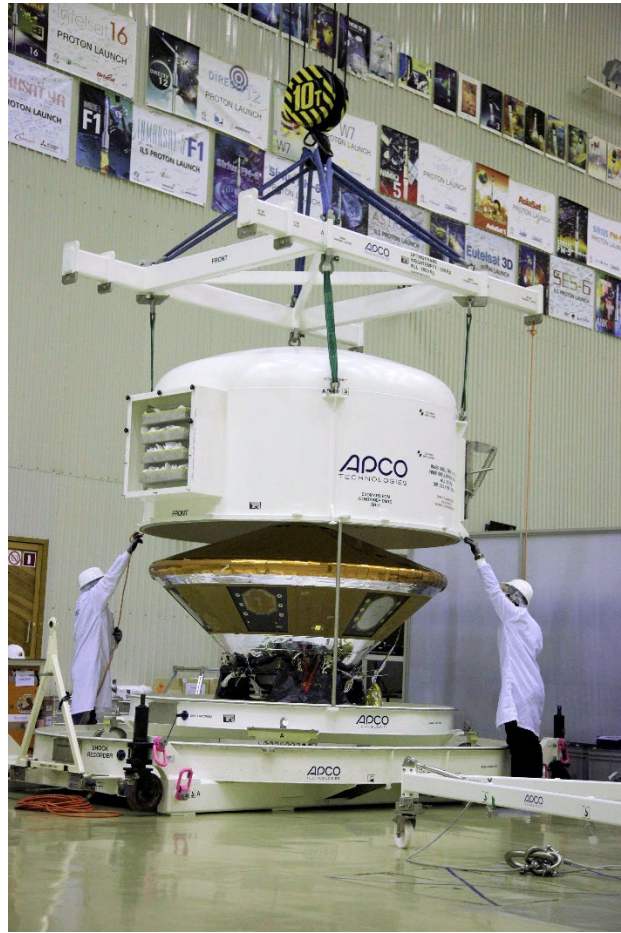
Figure 4-3: Exomars Schiaparelli Descent Module Container
