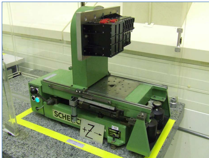
Figure A-3: CoG measurement along vertical axis
