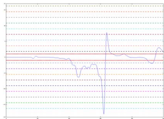
Figure 7-1: Curve scanning principle with threshold values
