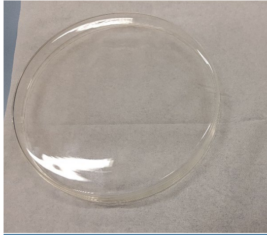
Figure K-6: Example of a dummy surface which can be used to prepare a sample for transfer efficiency measurements
