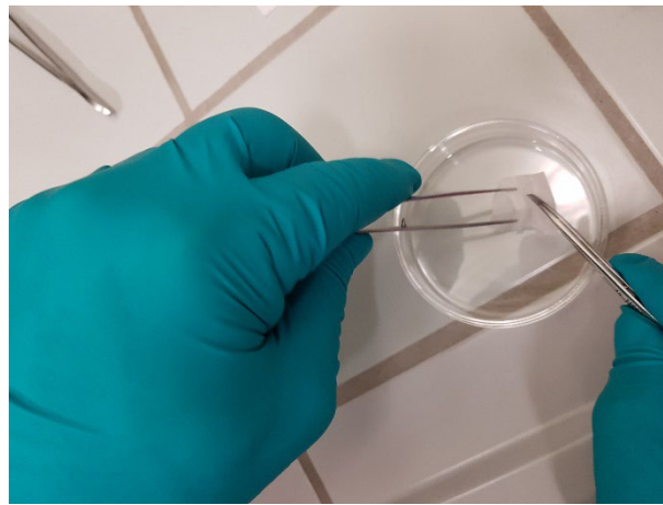
Step 2: Unfolding a wetted tissue over a clean Petri dish. This manual process is repeated five times for five independent wipes, in line with 5.4.3.7.2e.
