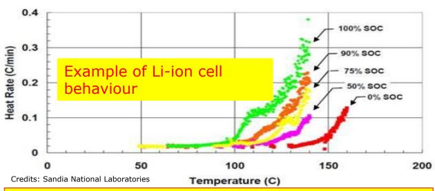
The onset temperature of self-generating heating (thermal runaway) decreases with increasing State of Charge (SoC)
