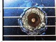
Impact on HST MLI Outer damage size: 5 mm; Hole size: 464 um
