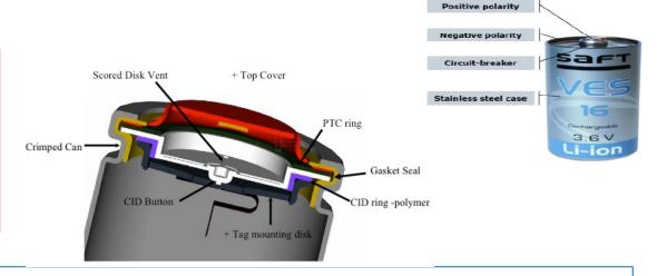
Typical safety devices that can be found in a battery cells (cylindrical cells 18650):
