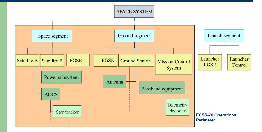
This is the architecture of a traditional ESA mission. Boundaries do vary e.g. In some cases EGSE is shared, in some Ground Station are 3<sup>rd</sup> party and effectively external. Mission control is also sometime separate for Space and Ground
