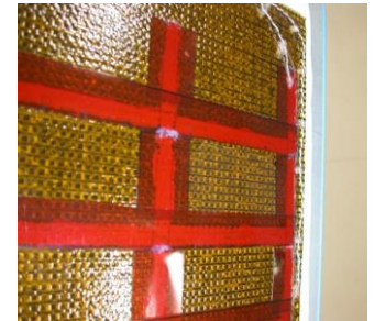
Coverglass ready for thermal cycling test
