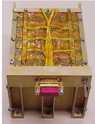
PROBA1 6S6P 18650HC ABSL battery module
