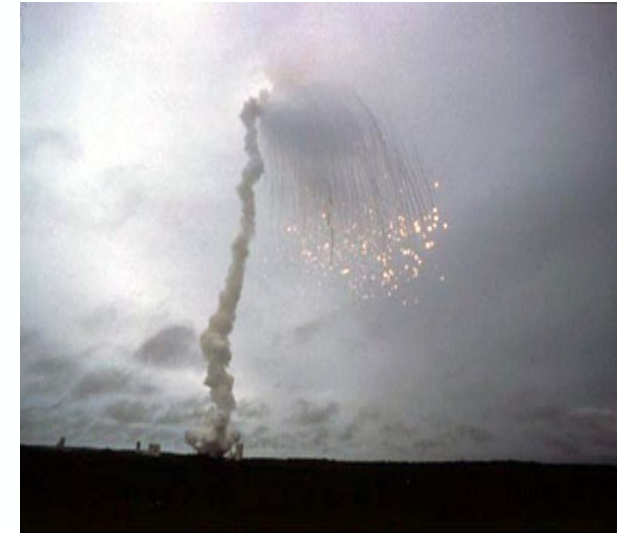
Ariane 501 failure. Since this failure ESA has put a number of measures in place for development, verification and validation of flight and ground software such as ISVV and Spice4Space
