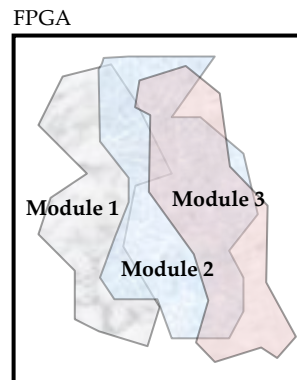
Figure 13-6: Physical implementation of global TMR inside an FPGA
