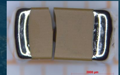
Figure 10: Optical micrograph of flex crack in MLCC
