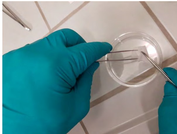
Step 2: Unfolding a wetted tissue over a clean Petri dish. This manual process is repeated five times for five independent wipes, in line with 5.4.3.7.2e.
