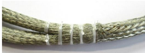
Figure 7-10: Secured braid along the breakout
