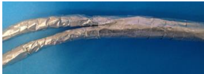
Figure 7-13: Example of acceptable foil shielding
