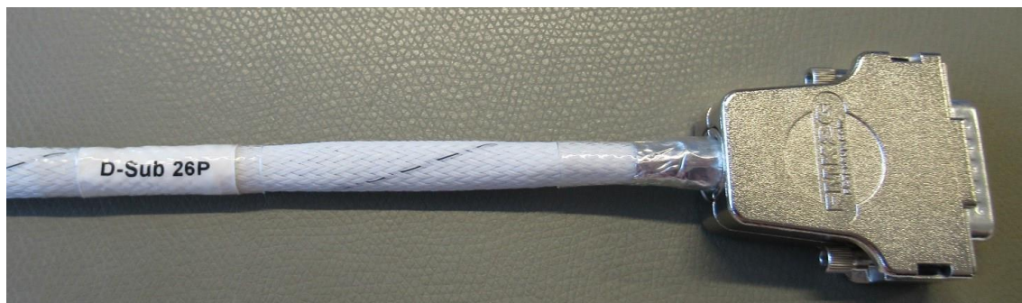
Figure 7-7: Connector label applied onto harness bundle
