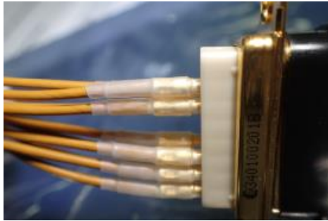
Figure 7-1: Double sleeving on D-Sub contacts
