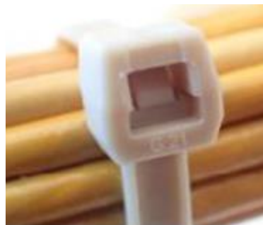
Figure 6-4: Tie-wrap – receded tail
