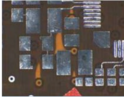
Figure 10-79: Examples of unacceptable discoloured copper oxide originating from a via
