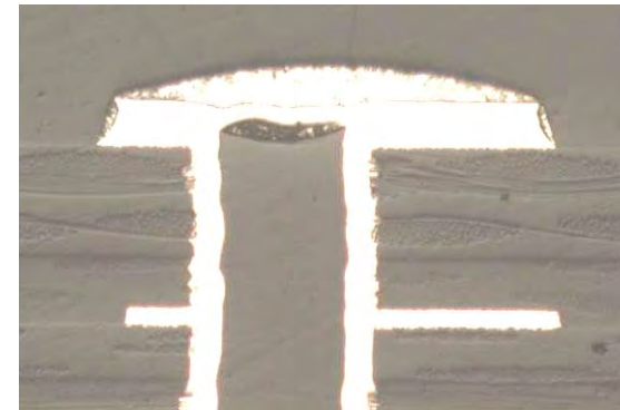
Figure 10-33: Example of non-acceptable bulging
