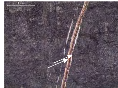
Figure 10-75: Example of visible copper on top surface (left) and on side of track (right)
