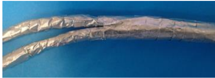
Figure 7-13: Example of acceptable foil shielding
