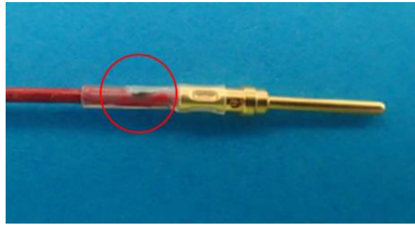
Figure 7-5: Example of foreign particles entrapped under shrinking sleeve
