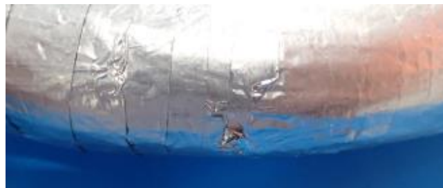
Figure 7-15: Example of not acceptable foil shielding
