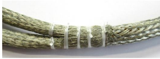
Figure 7-10: Secured braid along the breakout
