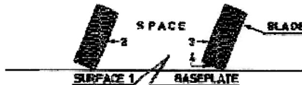
Figure 7-7: Schematic blade geometry for diffuse body radiation analysis. Louvers of the control subsystem. NIMBUS spacecraft. From London (1967) [20].
