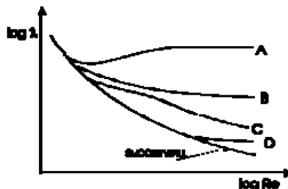
Figure 7-1: Friction characteristics associated with four types of roughness geometry. Notice that the equivalent roughness is different in every case. From Reynolds (1974).
