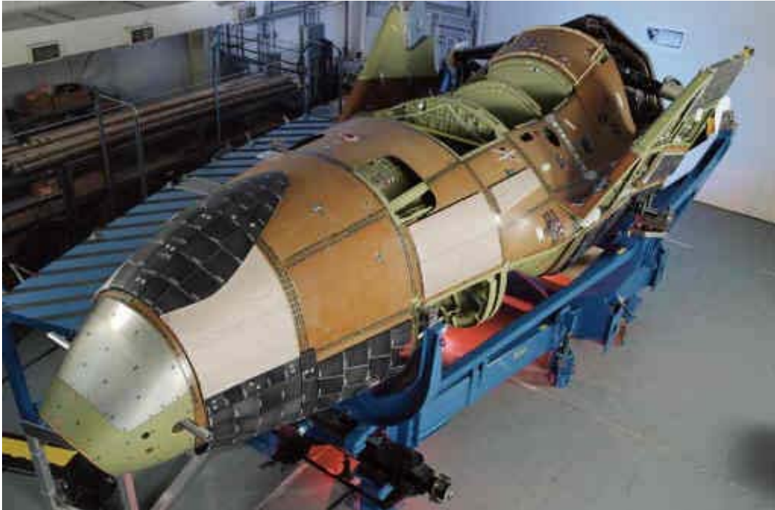
Figure 6-41: FEI Blankets Integrated on the X-38 V-201
