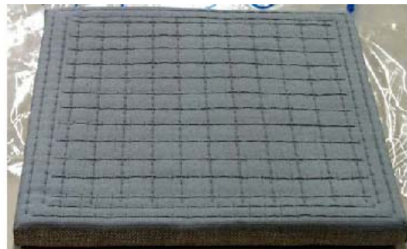
Figure 6-35: Typical look of FEI-650 and Blanket with Gray High Emittance
