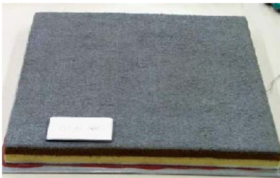
Figure 6-34: FEI-450 Blanket equipped with Gray FEI-1000 High Emittance Coating
