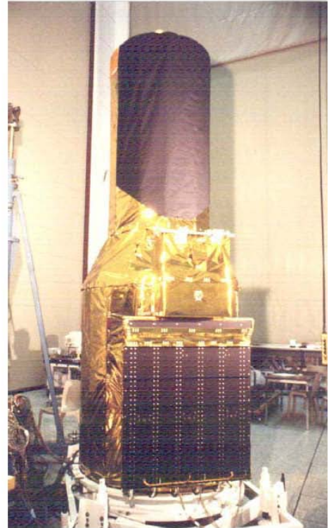
Figure 9-25: “Thank to 40 state-of-the art variable conductance heat pipes located in the avionics bay the ATV is able to carry away the heat and release the energy directly into space or, otherwise, to warm up other parts in a very economic fashion” Astrium – ESA “Jules Verne goes hot and cold” – Successful achievement of the Qualification Thermal Test campaign – 14 Dec 2006.
