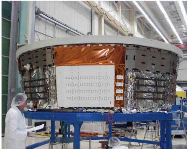
Figure 9-25: “Thank to 40 state-of-the art variable conductance heat pipes located in the avionics bay the ATV is able to carry away the heat and release the energy directly into space or, otherwise, to warm up other parts in a very economic fashion” Astrium – ESA “Jules Verne goes hot and cold” – Successful achievement of the Qualification Thermal Test campaign – 14 Dec 2006.
