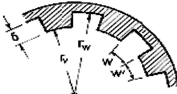
Figure 7-1: Sketch illustrating design variables in grooved heat pipes. From Frank et al. (1967) [27], quoted by Winter & Barsch (1971) [96].
