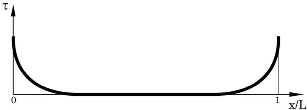
Figure 21.9-8 - Shear stress distribution for large overlap lengths
