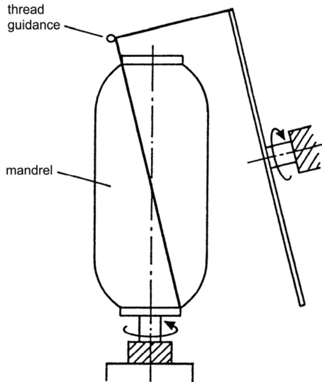
Figure 38.6-1 - Filament winding: Polar vertical
