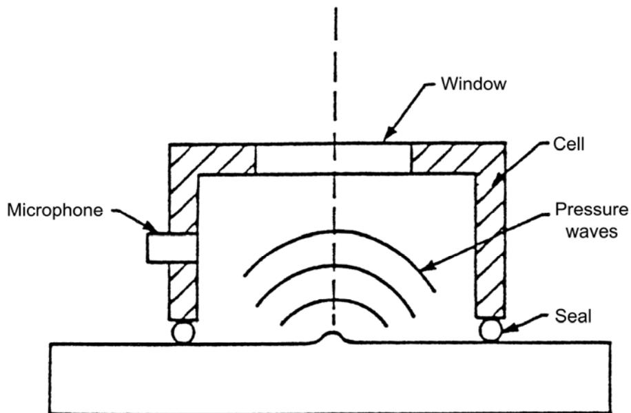
**Figure 34.15-4 - Thermal-wave imaging: Photoacoustic gas cell**
