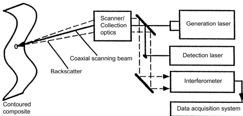
**Figure 34.12-1 - Laser ultrasonic test system: Diagrammatic representation**
