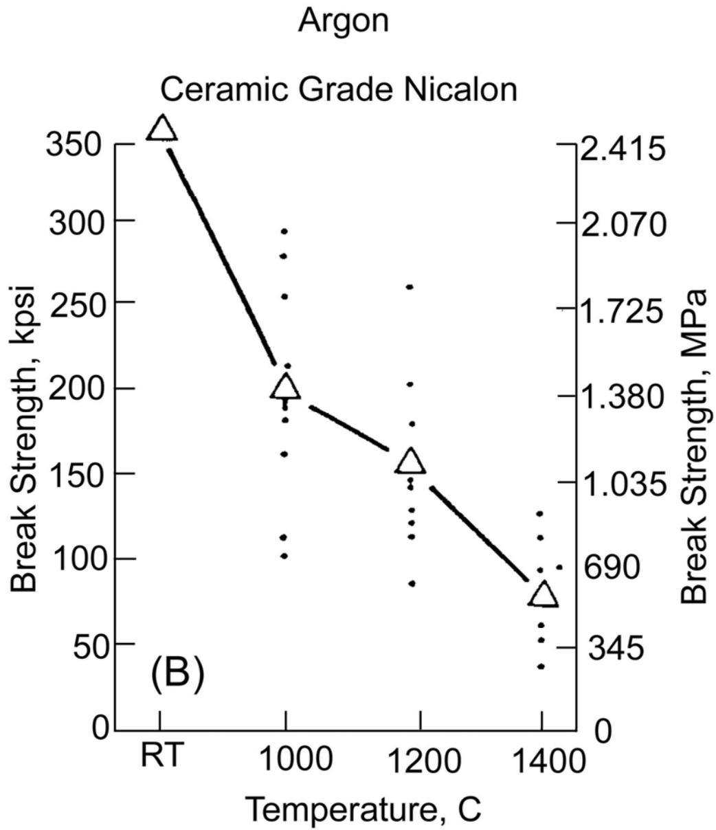
After 12 hour furnace soak in flowing argon
