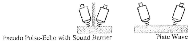
**Figure 34.10-5 - Non-contact ultrasonics: Air-coupled sensor configurations**
