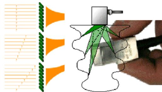
**Figure 34.10-4 – Phased-array transducers: Functionality**
