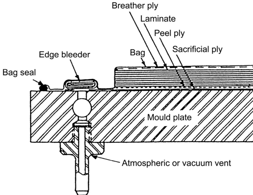
Figure 38.4-5 - Bag moulding: Edge bleed out system
