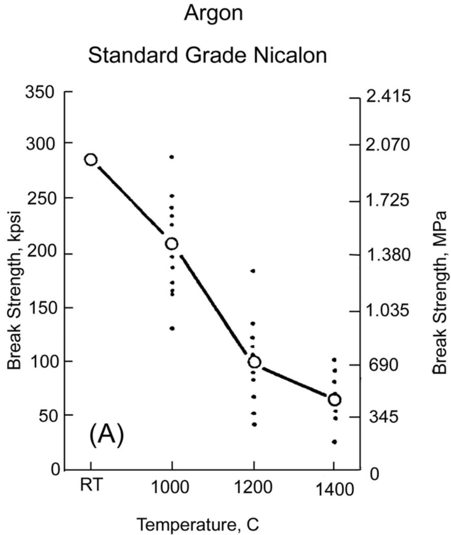
After heat treatment in flowing argon furnace environment (12 hour soak)
