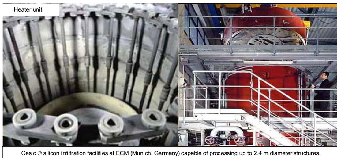
**Figure 43.12-2 – Cesic®: Silicon-infiltration processing equipment**
