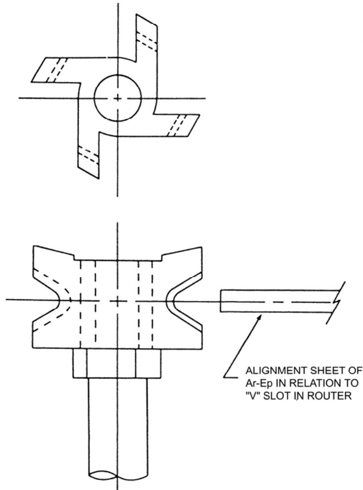
Figure 39.3-2 - Router for trimming aramid/epoxy composites
