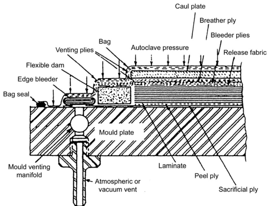
Figure 38.4-4 - Autoclave moulding method, with vertical bleeder
