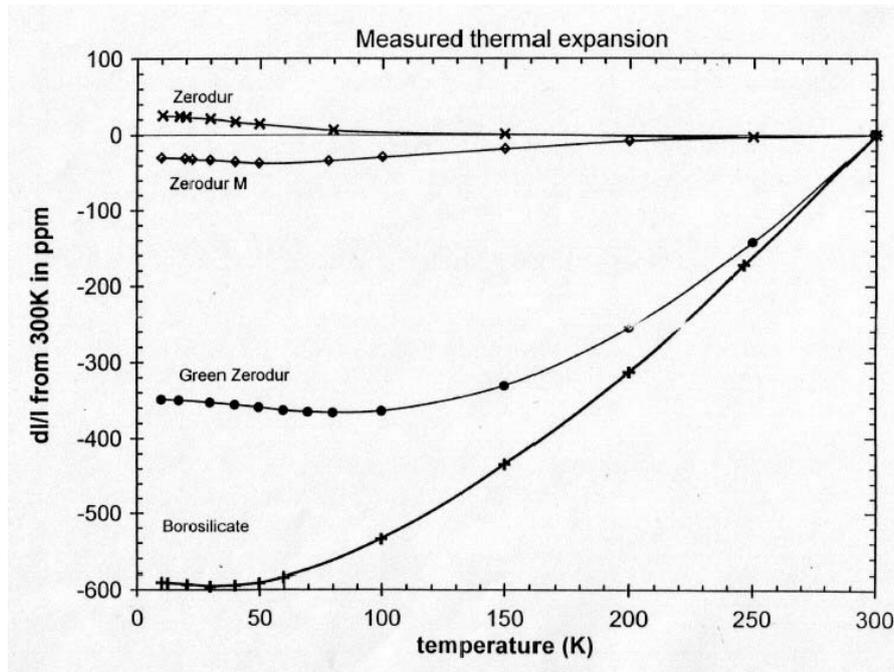
Figure 43.15-8 - Zerodur®: Thermal expansion of different glass ceramics
