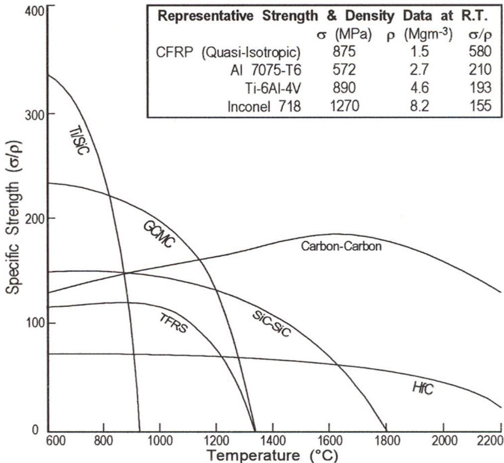
Figure 42.2-2 - Specific strength against temperature for advanced materials
