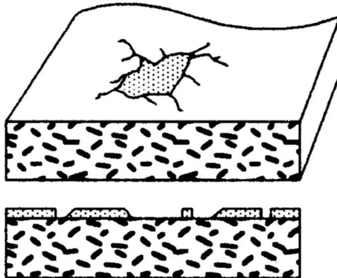
Figure 41.3-3 - Damage categories: Chipping
