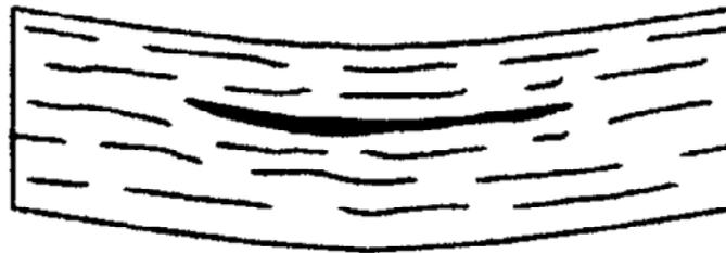
Figure 41.3-5 - Damage categories: Delamination
