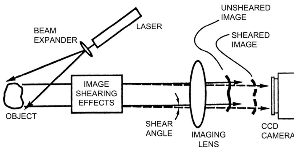
Figure 34.14-1 - Electronic shearographic system: Schematic diagram
