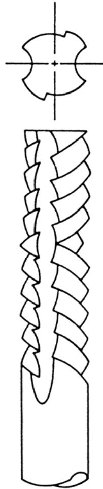
Figure 39.3-1 - Router: Opposed helix for aramid/epoxy
