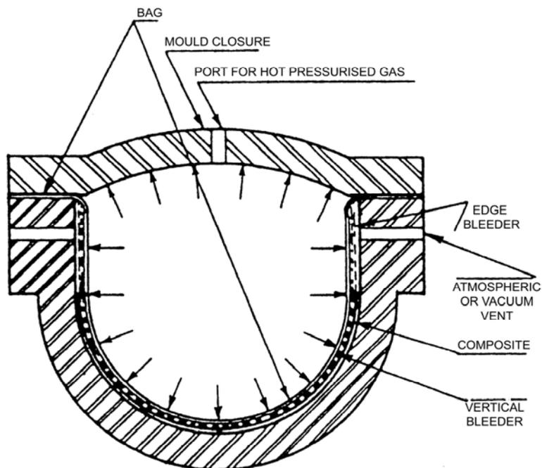
Figure 38.4-2 - Pressure bag moulding
