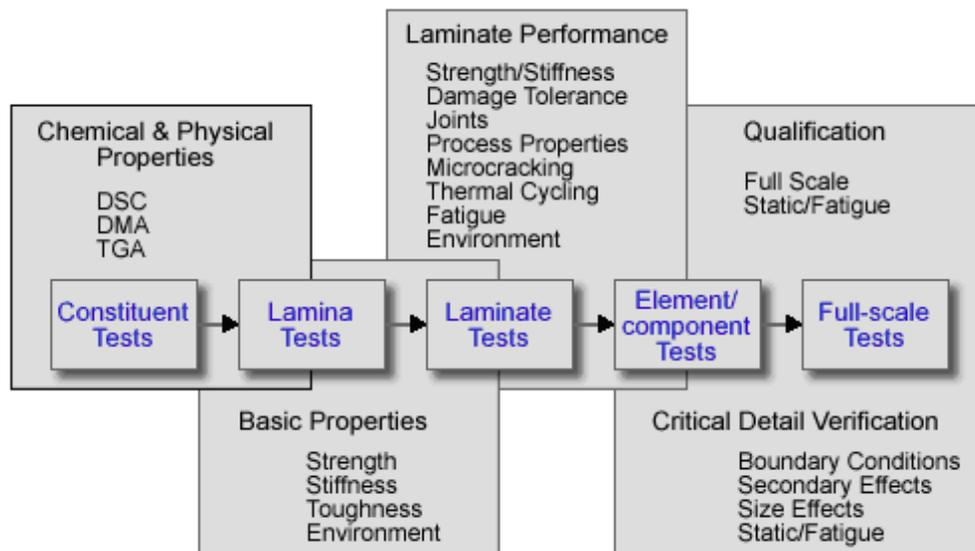
Figure 33.6-2 - Building block approach: Composite materials
