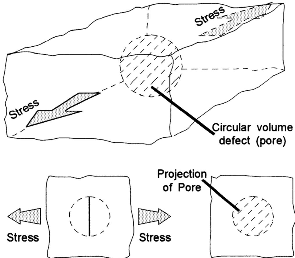
**Figure 33.4-1 - Metal structures: Idealisation of a volumetric defect**
