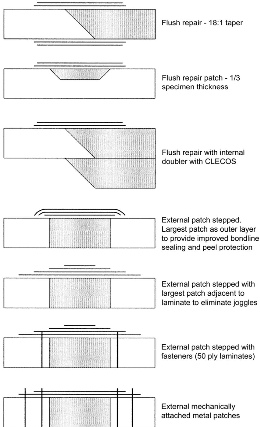
**Figure 41.4-1 - Basic repair concepts**
