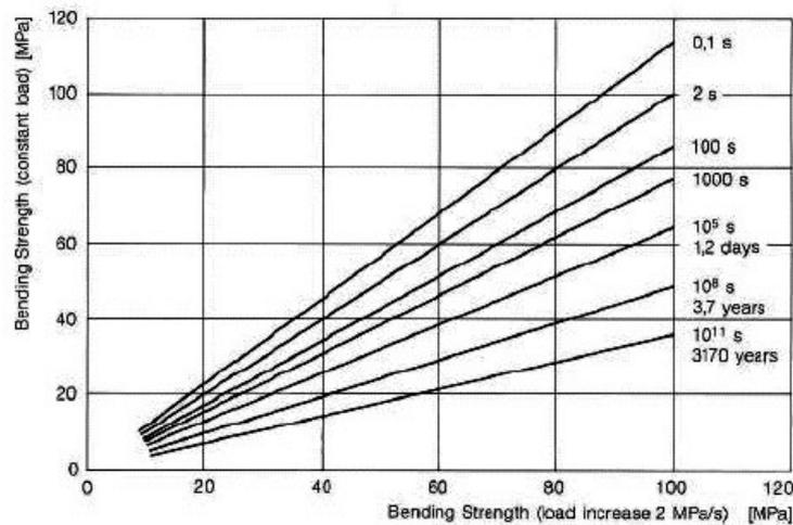
**Figure 43.15-13 - Zerodur®: Bending strength under constant load**
