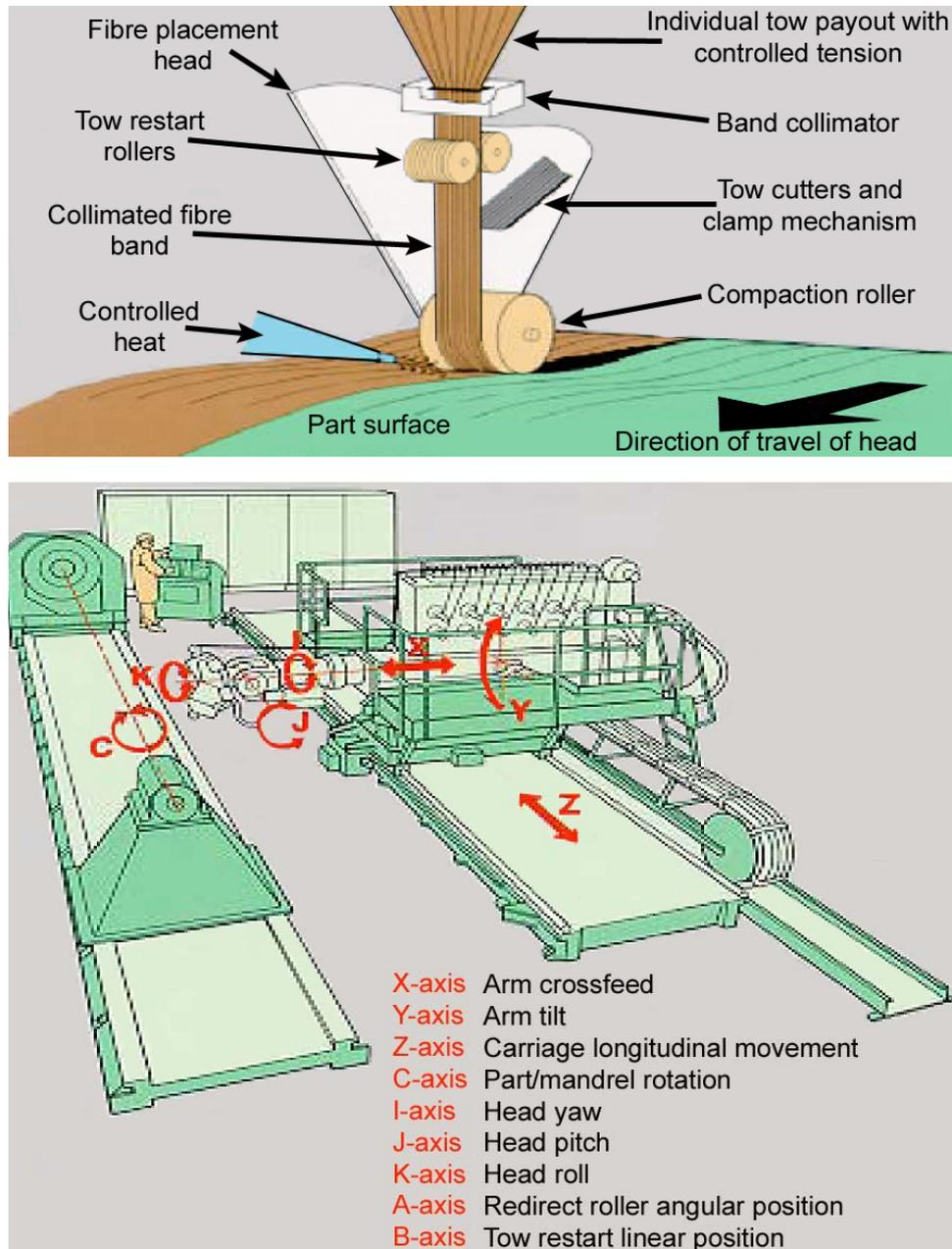
**Figure 38.14-1 – Fibre placement: Schematic view of the system**
