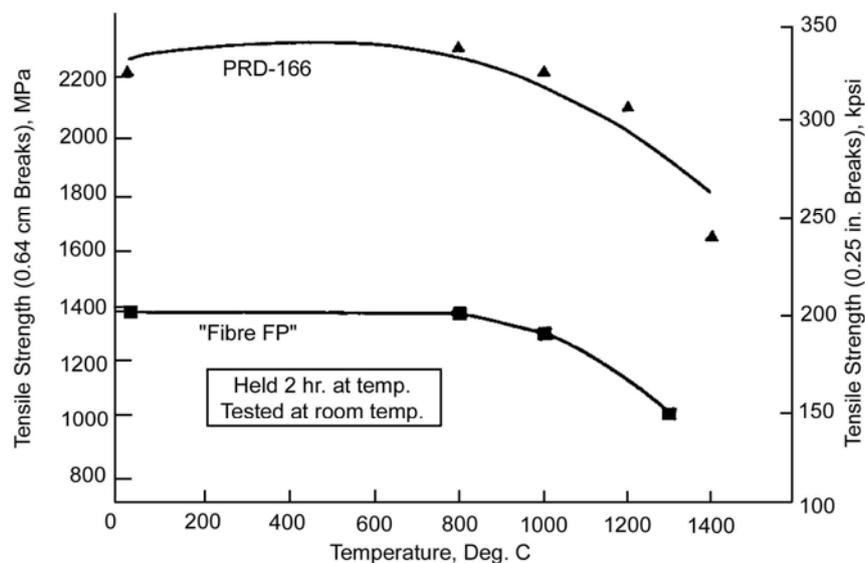
Figure 42.6-10 - Alumina fibres: tensile strength against exposure to elevated temperature
