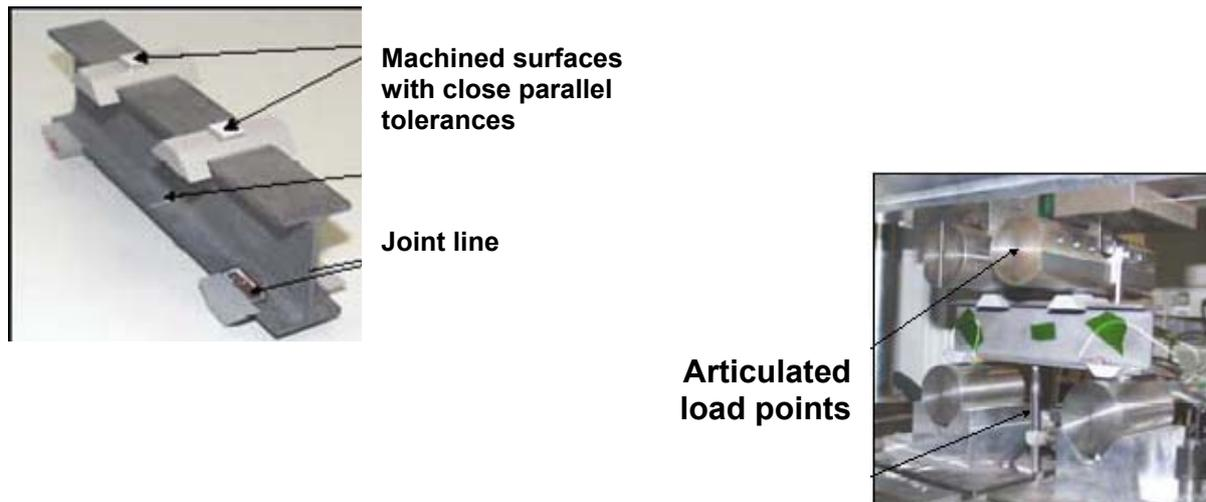
**Figure 43.18-2 – NIRSpec optical bench development: Test set-up and I-beam sample with joint line**
