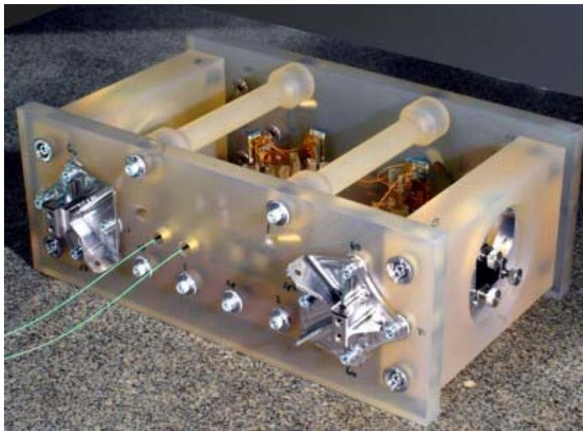
**Figure 43.19-1 – Zerodur®: Optical bench for LISA pathfinder mission**
