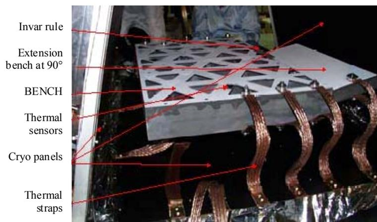
**Figure 43.18-5 – NIRSspec optical bench development: Test set-up for cryogenic temperature test**
