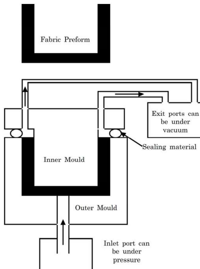
Figure 38.7-1 - Resin transfer moulding (RTM): Process
