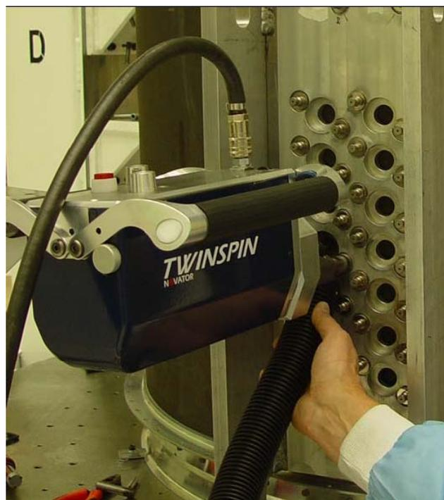
Figure 39.10-2 – Orbital drilling: Equipment mounted on a jig
