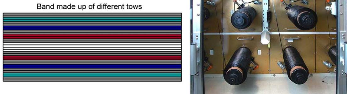
Figure 38.14-8 – Fibre placement: Mixed-material lay-up
