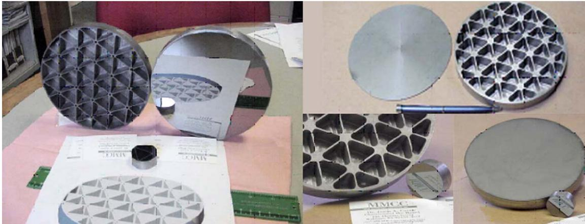
Pre-polished Si membrane bonded to lightweight substrate.
