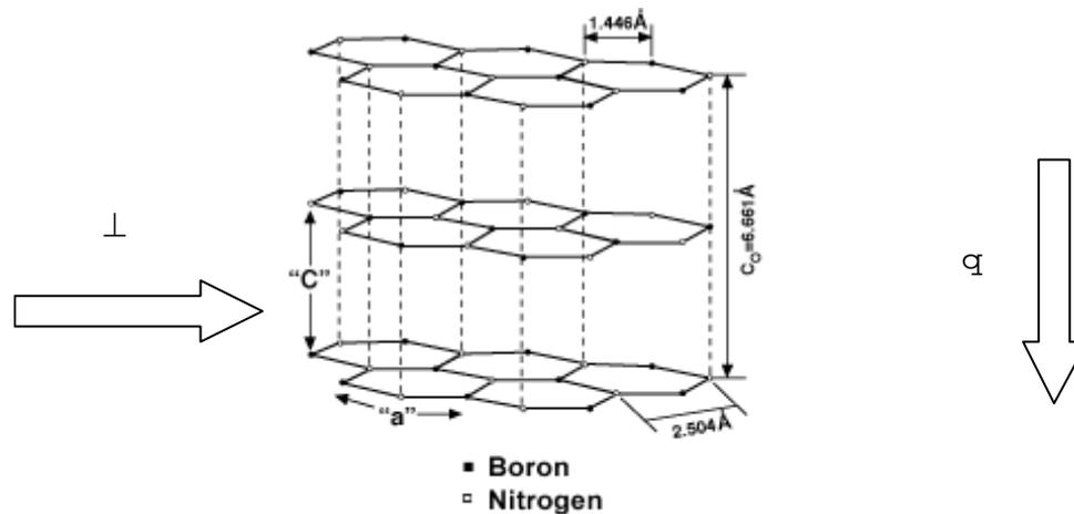
**Figure 43.9-1 – Technical ceramics: pyrolytic boron nitride – structure**
