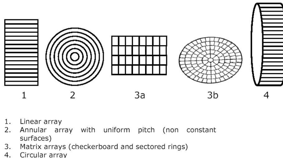
**Figure 34.10-3 – Phased-array transducers: Element configurations**
