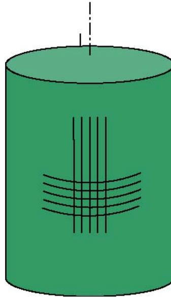
Fibre placement enables the incorporation of purely axial plies
