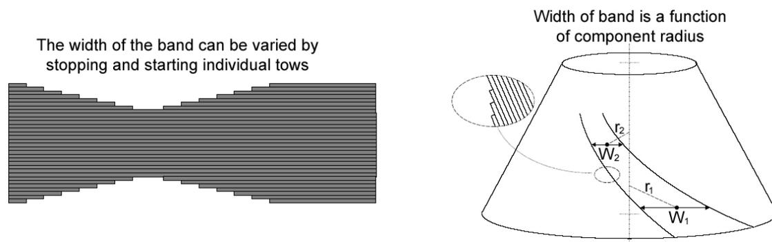
**Figure 38.14-7 – Fibre placement: Variation of band width**
