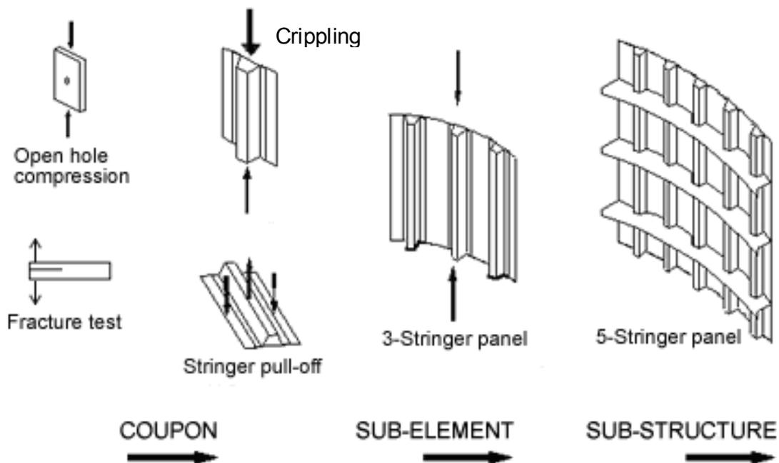
Figure 33.6-1 - Building block approach: Test programme development
