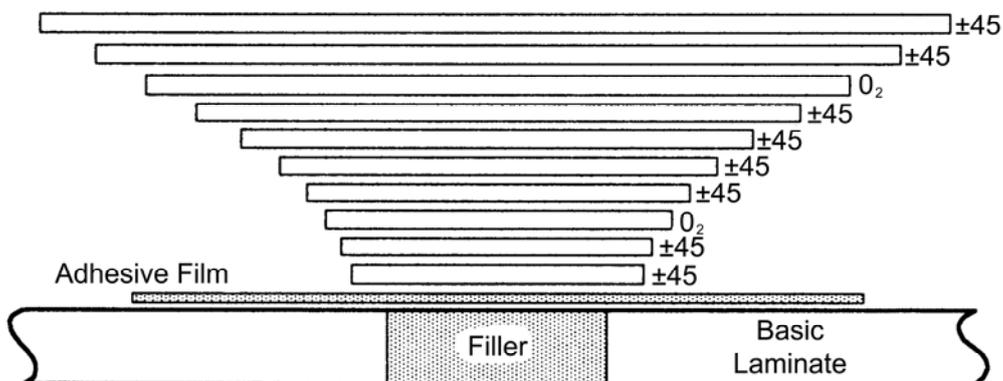
Figure 41.6-2 - External repair: Cured in place
