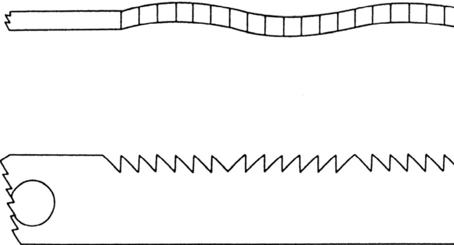
Figure 39.5-3 - Sabre sawing: Alternating tooth blade for aramid/epoxy
