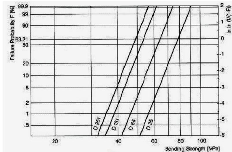
**Figure 43.15-10 - Zerodur®: Failure probability for test surfaces processed with bonded grit of different sizes**
