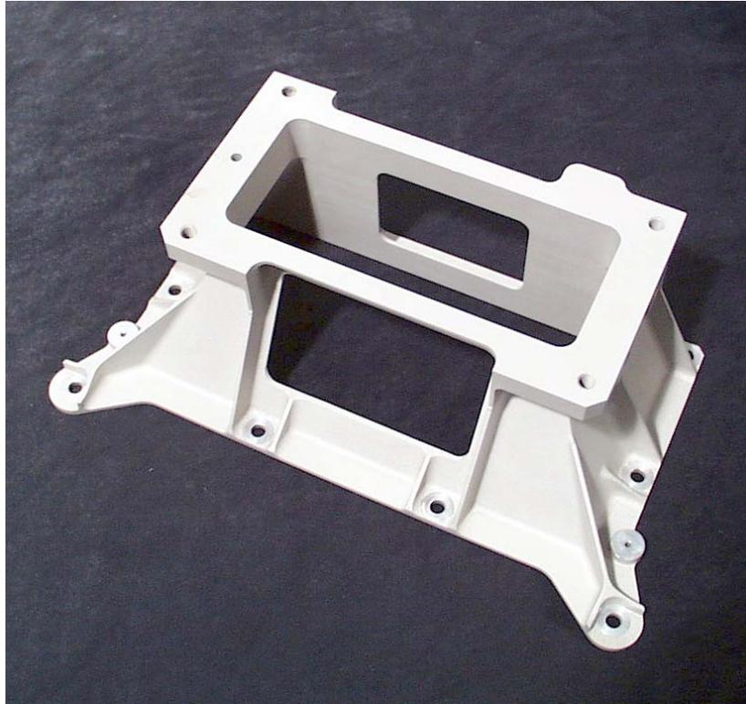
This item is 250 mm × 150 mm × 80 mm and was machined from ZK60A-T5 extruded bar and treated with ALGAN 2 plus OXSILAN® MG 0611, Ref. [\[44-22\]](#).
