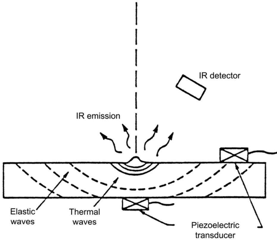
**Figure 34.15-3 - Thermal-wave imaging: Photothermal and piezoelectric detection**
