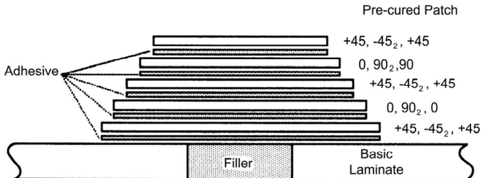
Figure 41.6-1 - External repair: Pre-cured patches
