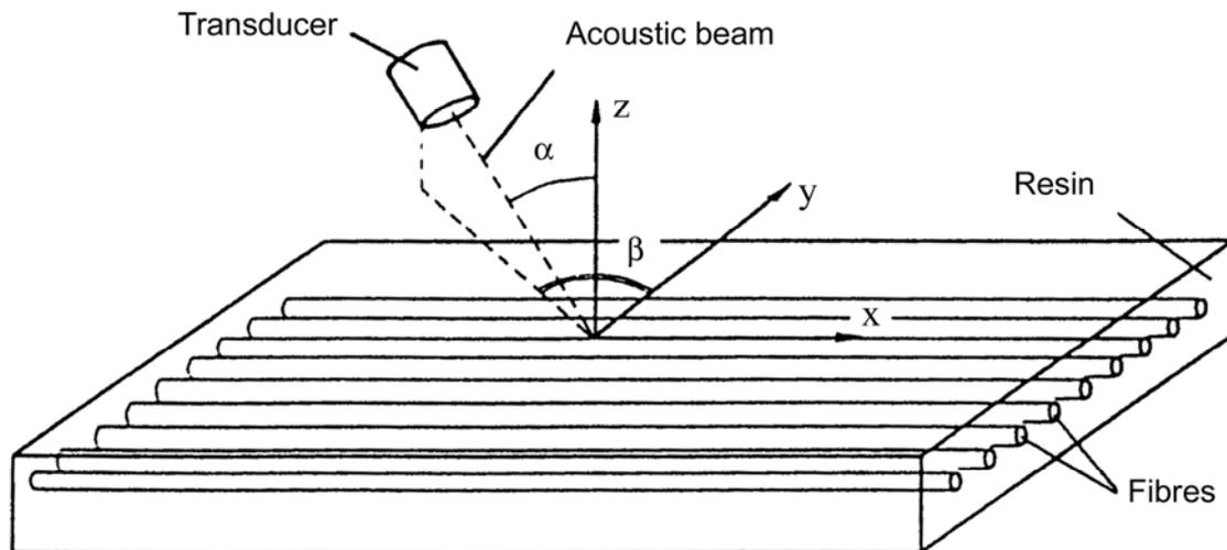
Figure 34.10-2 - Detection of fibre orientation by backscattering measurement
