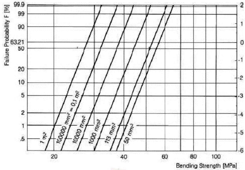
The values for the test surface area  $SL = 113 \text{ mm}^2$  are measured by test. Test conditions: Rate of stress increase  $2 \text{ MPa/s}$ ; test surface processed with D 151, air as surrounding medium. The values for the other test surfaces are calculated. □
