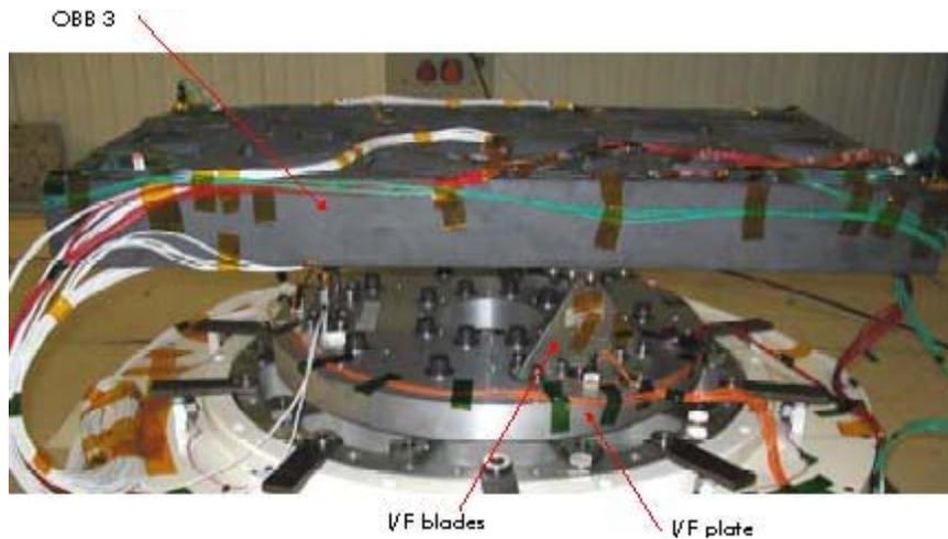
**Figure 43.18-4 – NIRSspec optical bench development: Test set-up for ‘shaker’ vibration tests**
