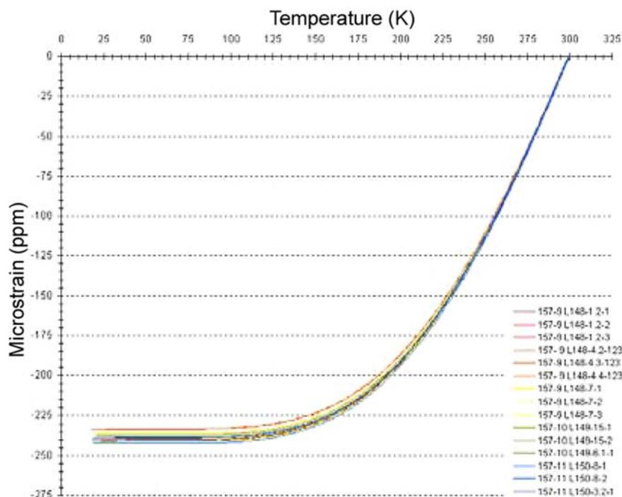
CTE measurement on 15 samples from 3 batches of materials tested in x-, y- and z-directions, where z-direction samples contained joints made prior to silicon infiltration.
