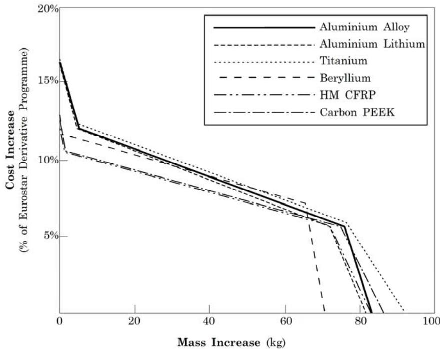
**Figure 40.3-2 - Mass/cost sensitivity for complete structure**
