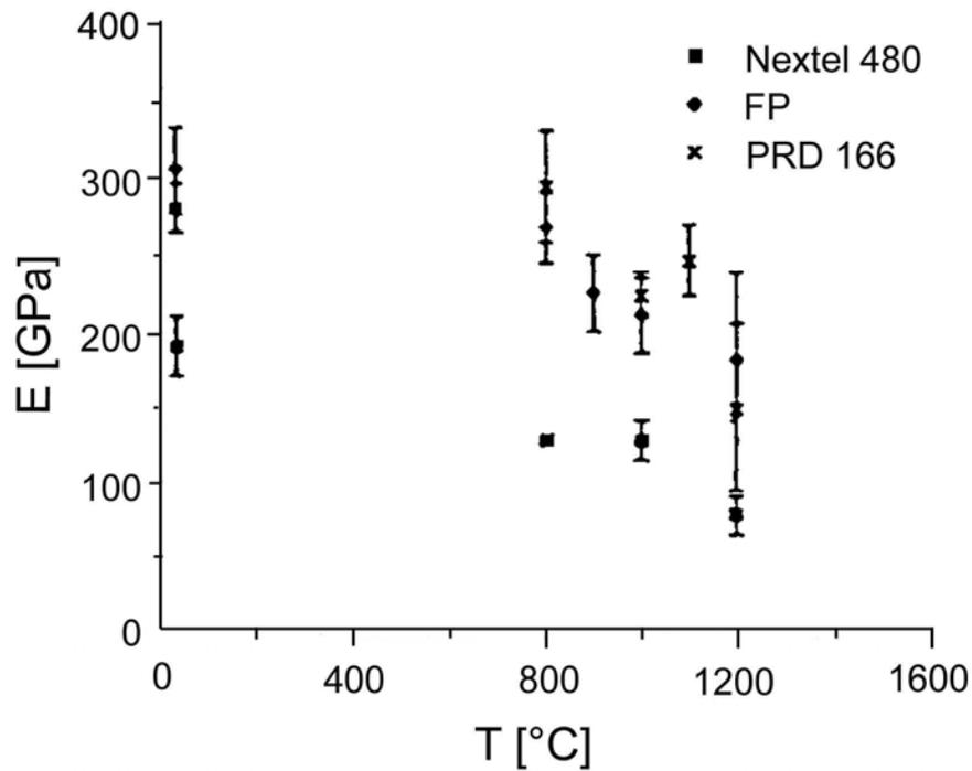
Figure 42.6-9 - Alumina fibres: modulus at elevated temperature
