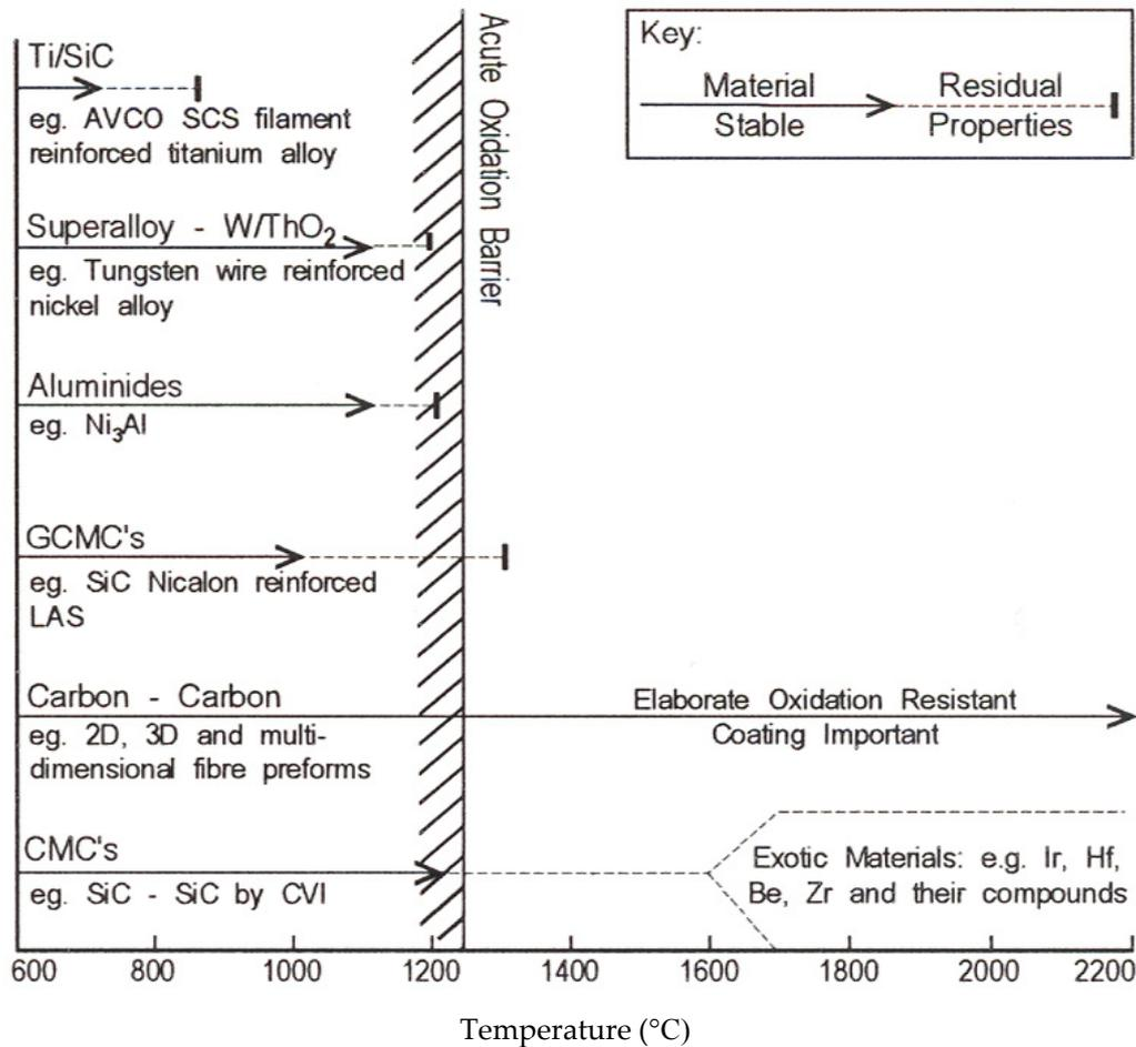
**Figure 42.2-1 - Classification of advanced metallic and ceramic materials with temperature**
