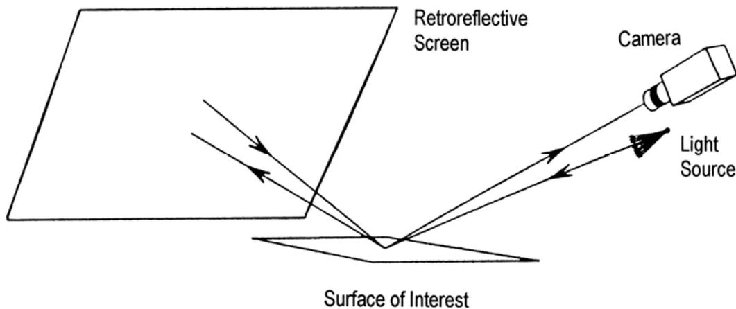
**Figure 34.19-1 - D sight - Diffracto sight schematic**
