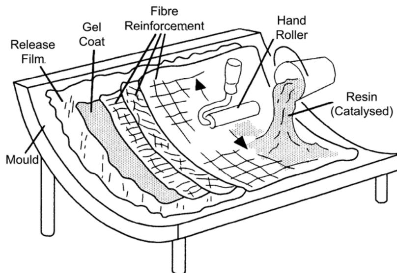
**Figure 38.3-1 - Hand lay-up process for mat or cloth**
