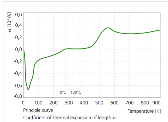
Figure 43.15-6 - Zerodur®: Thermal expansion – cryogenic behaviour
