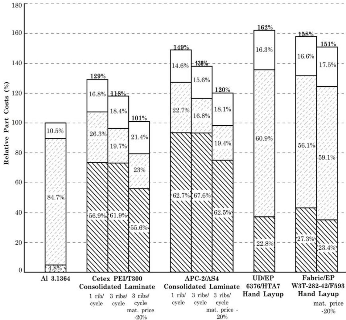
Key: Calculation basis: Landing flap rib thickness: 1.25 mm in CFRP, 1.0 mm in Al.
