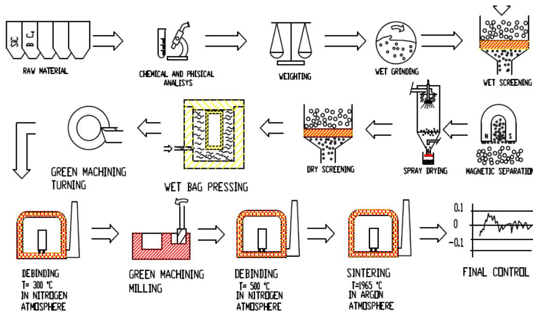
Figure 43.12-5 – SiC 54S® ceramic: Process sequence
