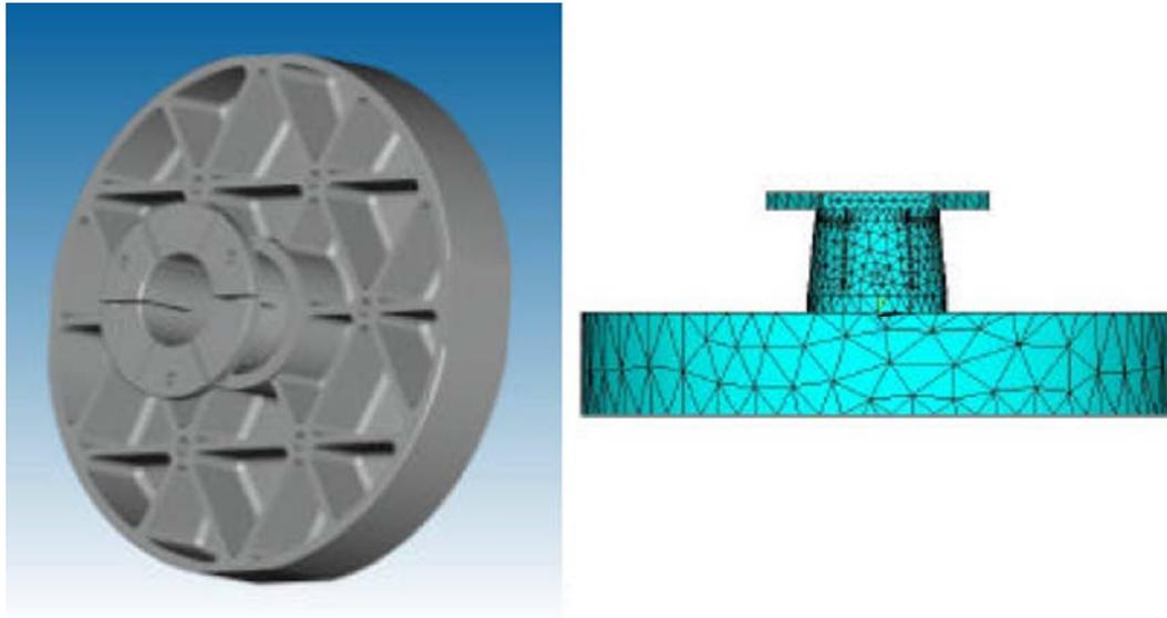
Figure 43.12-6 – SiC 54S®: NIRSpec prototype mirror
