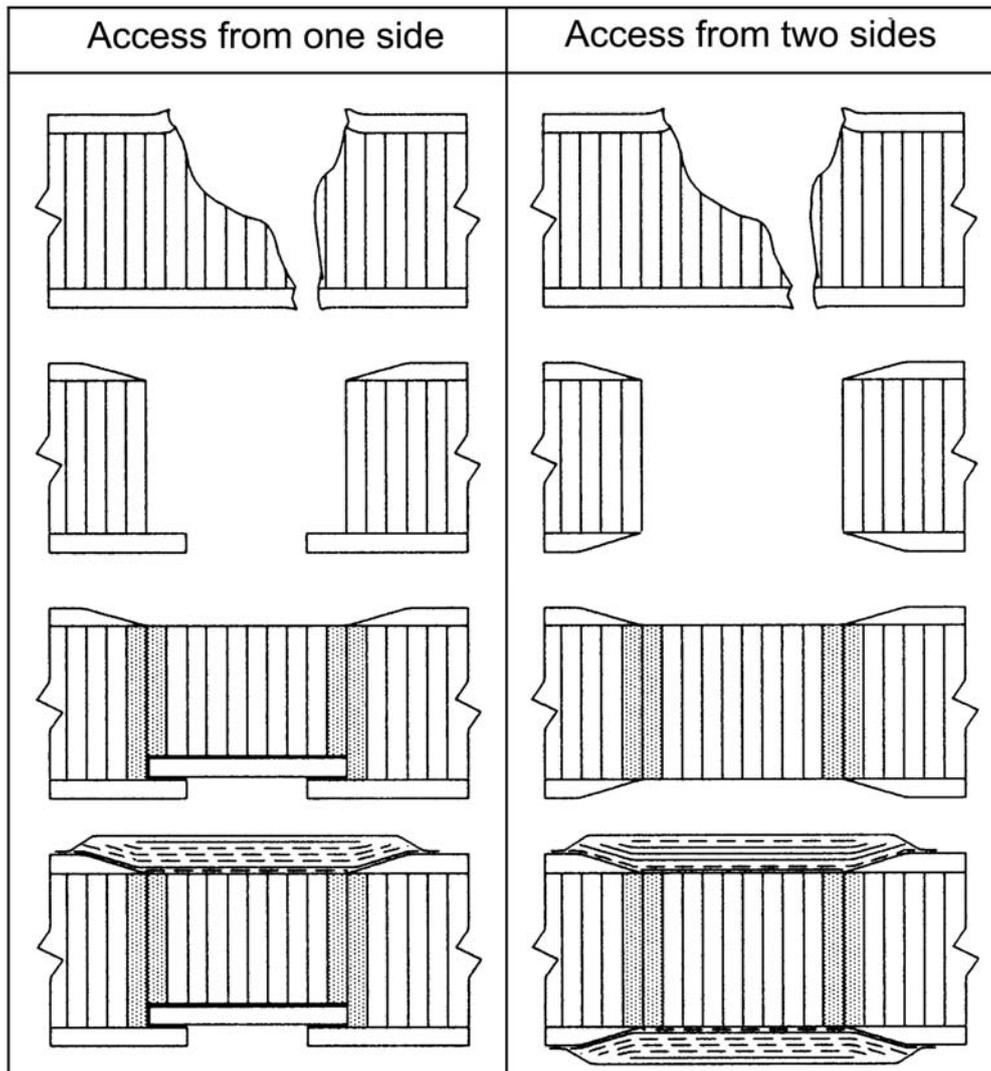
Figure 41.8-1 - Sandwich repair
