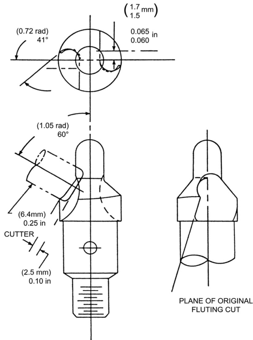
Figure 39.6-1 - Countersink for aramid/epoxy composite
