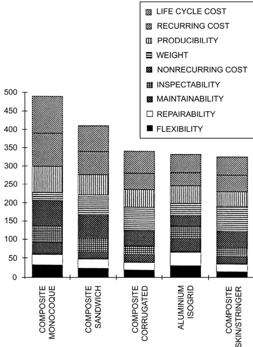
Figure 40.6-3 - Launcher fairing cylinder: Kepner-Tregoe evaluation scores for the section designs
