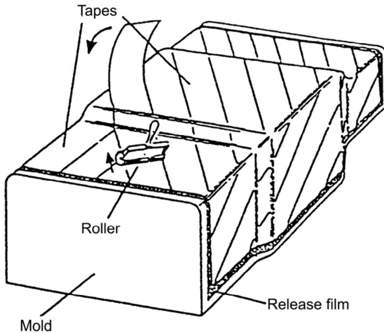
**Figure 38.3-2 - Prepreg: Direct lay-up**
