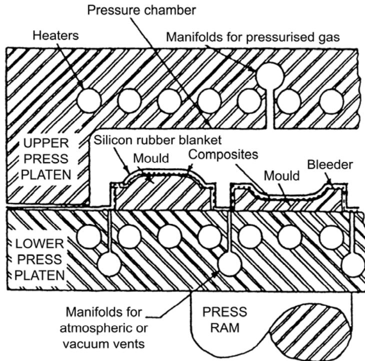
Figure 38.4-3 - Pressure bag moulding: Press modifications
