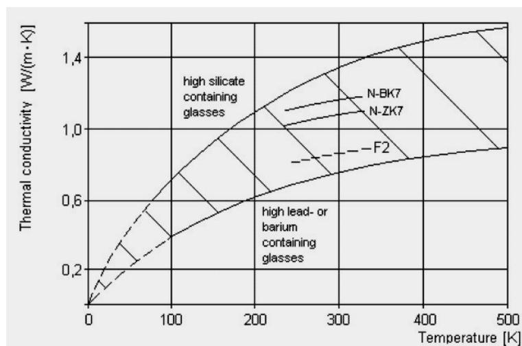
In [Figure 43.15.9](#), the thermal conductivity is plotted as function of temperature for different glasses, Ref. [\[43-94\]](#). The values of thermal conductivity for Zerodur are located between the two limiting curves in the diagram.
