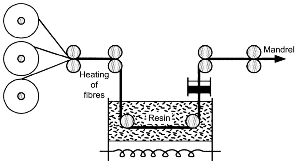
Figure 38.5-1 - Filament winding: Impregnation of fibres
