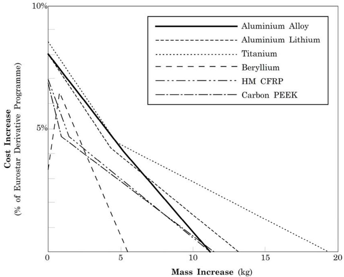
**Figure 40.3-1 - Mass/cost sensitivity for central thrust structure**
