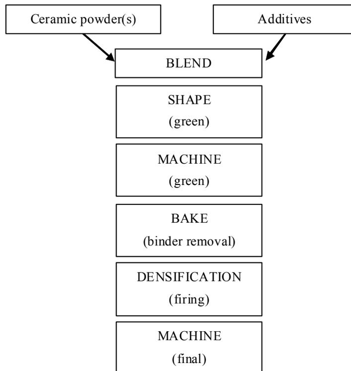
**Figure 43.4-1 – Technical ceramics: Manufacturing processes**
