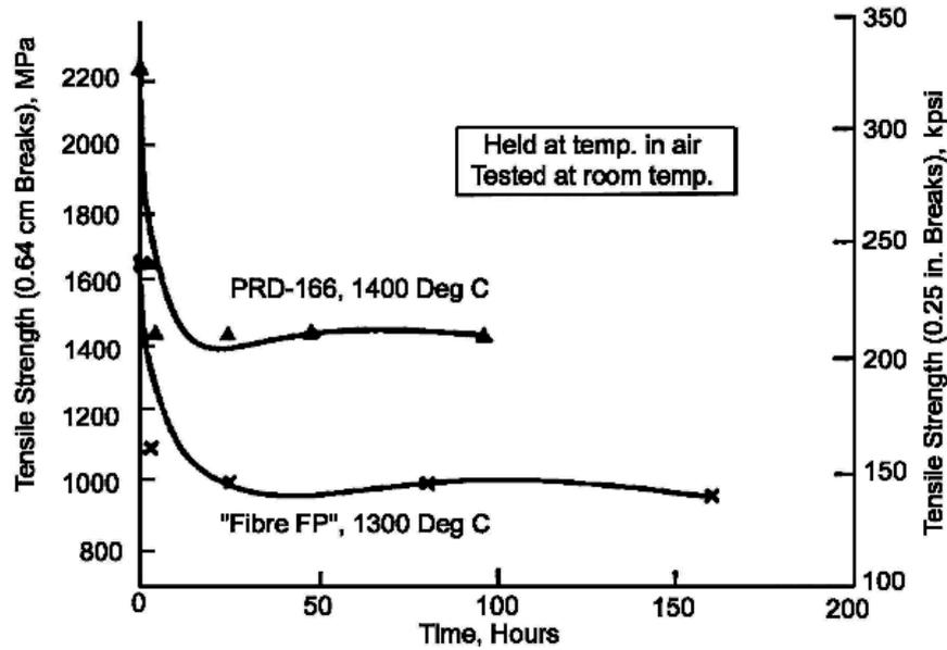
Figure 42.6-11 - Alumina fibres: tensile strength against exposure time
