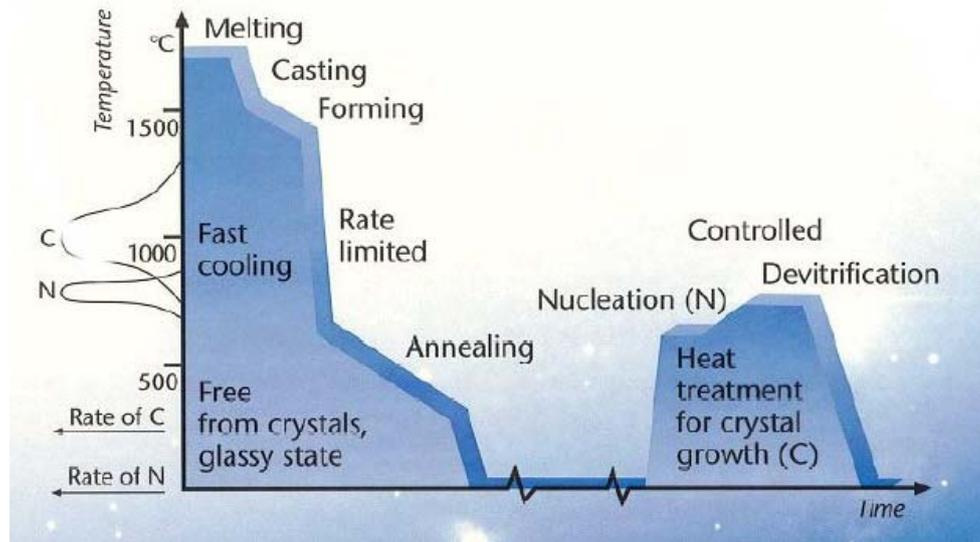
**Figure 43.15-3 - Zerodur®: Annealing process**
