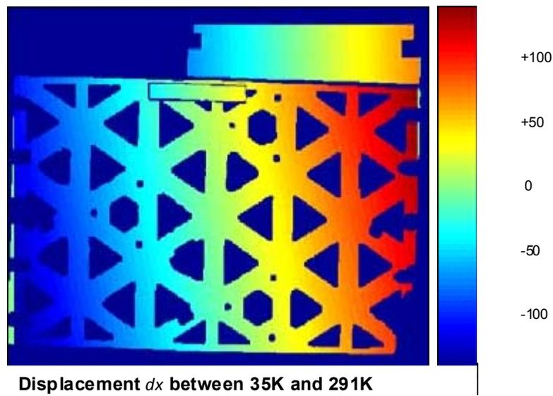
Figure 43.18-6 – NIRSpec optical bench development: Thermal contraction under cryogenic test
