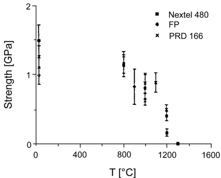
Figure 42.6-8 - Alumina fibres: tensile strength at elevated temperature
