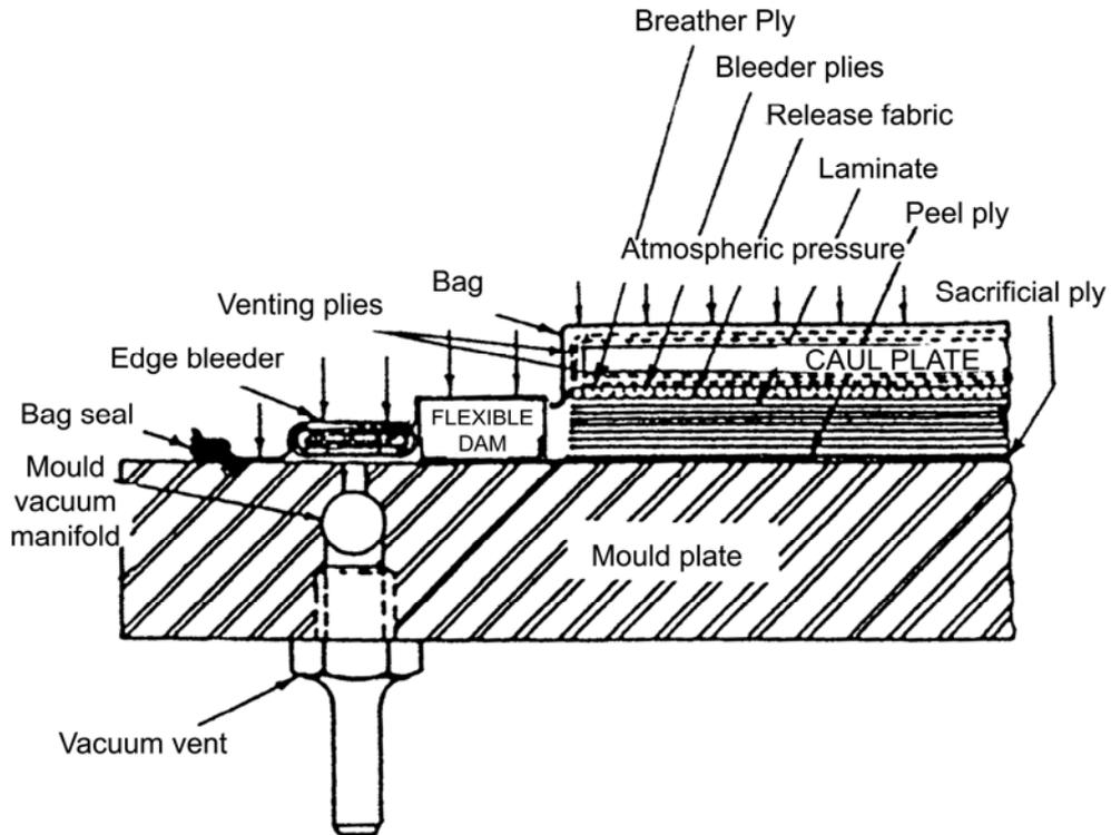
Figure 38.4-1 - Vacuum bag moulding method, with vertical bleeder
