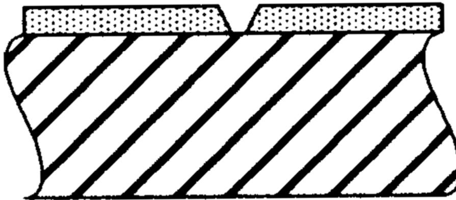
Figure 41.3-1 - Damage categories: Scratch
