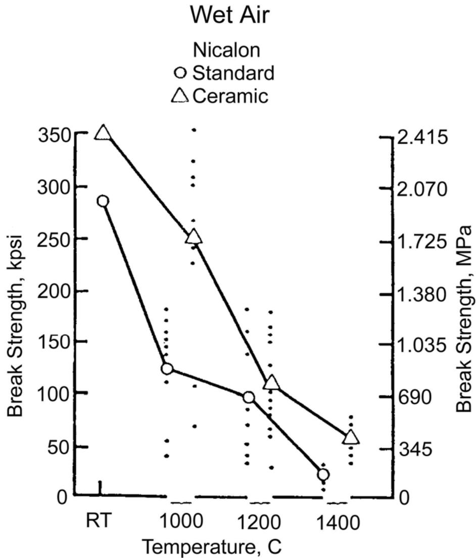
After heat treatments in flowing wet air furnace environment (12 hour soak)
