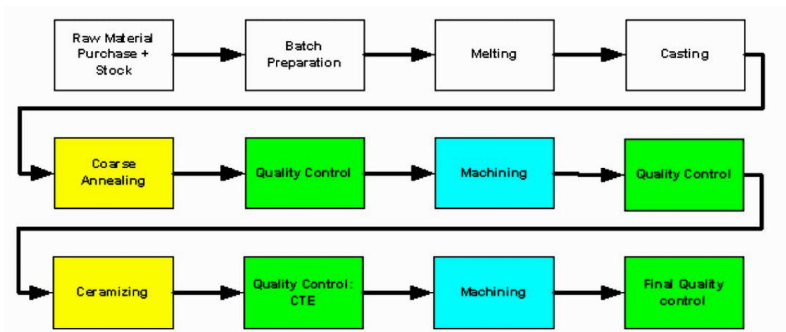
**Figure 43.15-2 - Zerodur®: Production process schematic**
