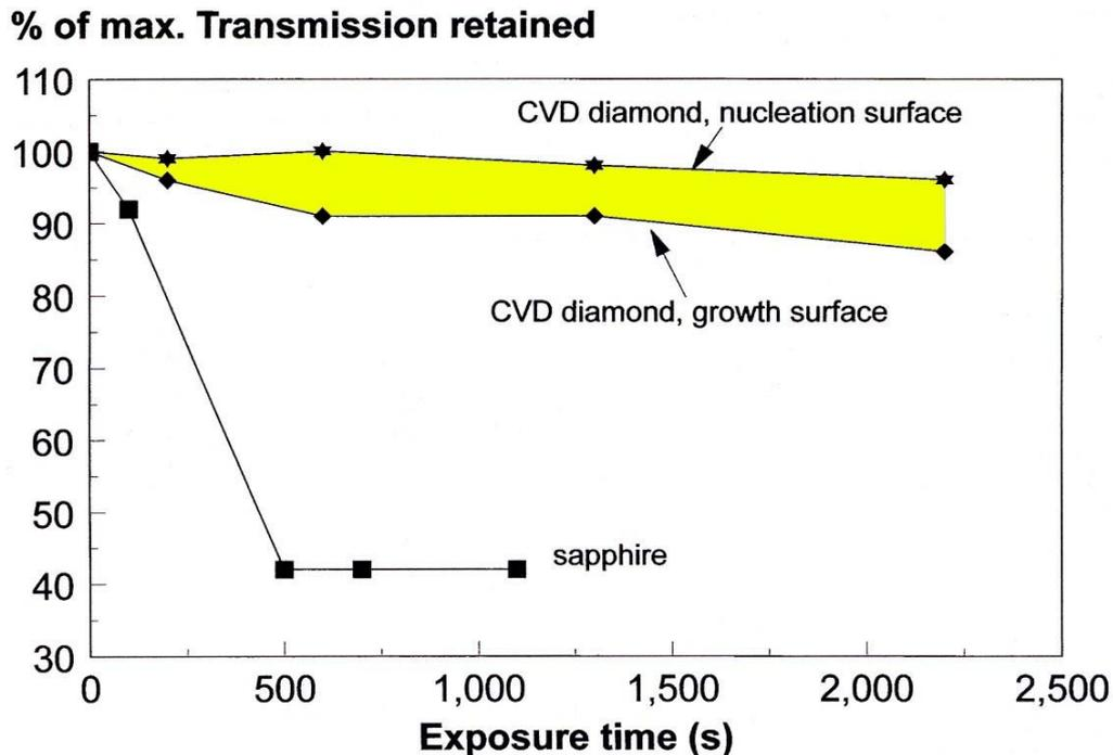
Retained transmission for CVD diamond is different depending on which production surface is exposed to sand erosion, i.e. upper bound is 'nucleation surface'; lower bound is 'growth surface'.
