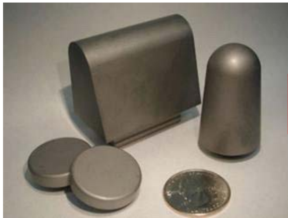
Figure 106.5-3 – CNT-modified ceramics: Potential application – NASA Ames HfB 2 -SiC arc-jet models of hypersonic vehicle components
