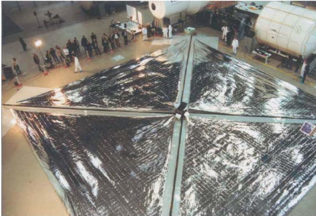
Figure 92.7-2 – Solar sail: CFRP deployable boom
