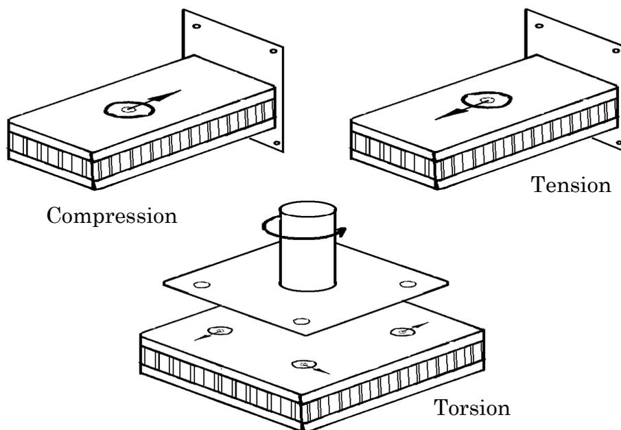
Figure 10-19: Failure modes: In-plane and torsion loads
