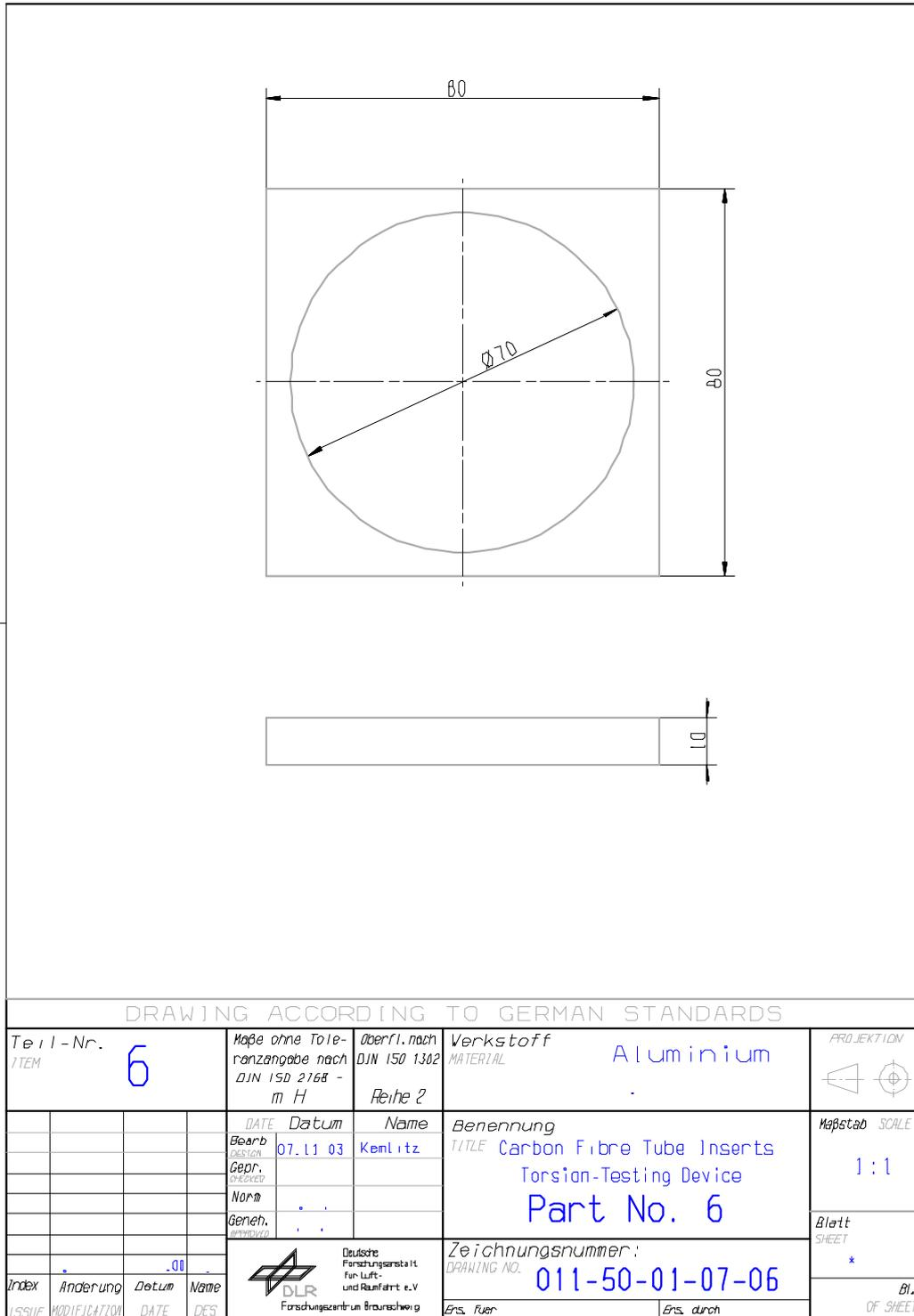
Figure H-37: Test fixture: Torsion – part 6
