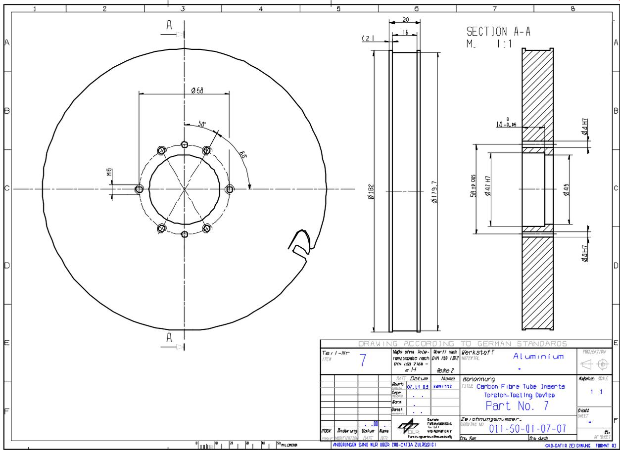
Figure H-38: Test fixture: Torsion – part 7
