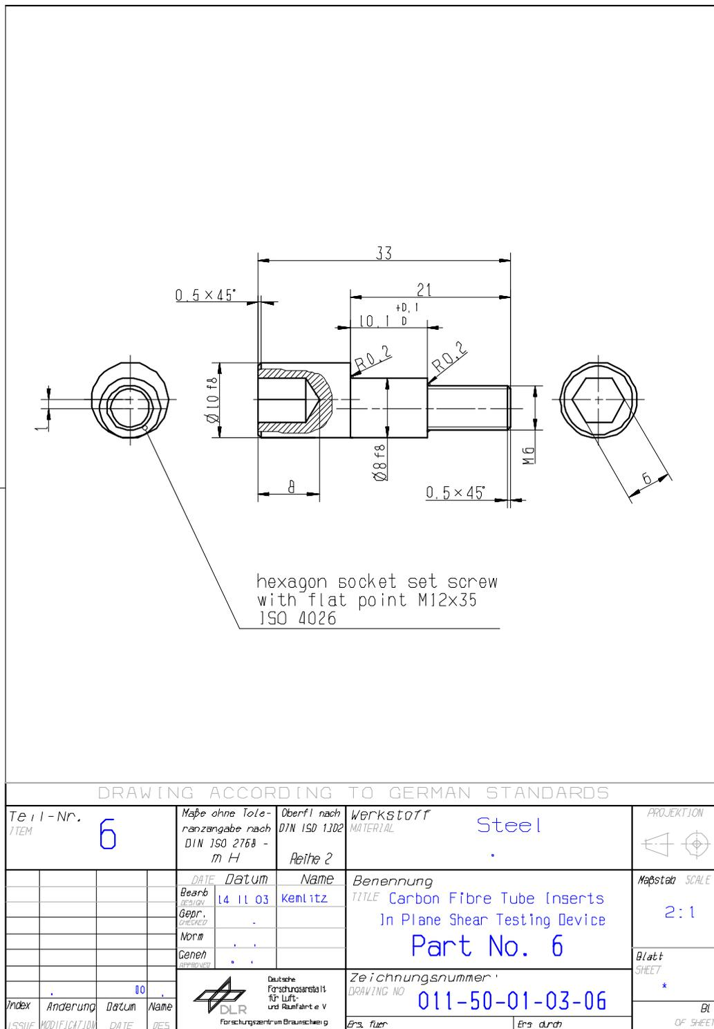
Figure H-15: Test fixture: In-plane shear load – part 6
