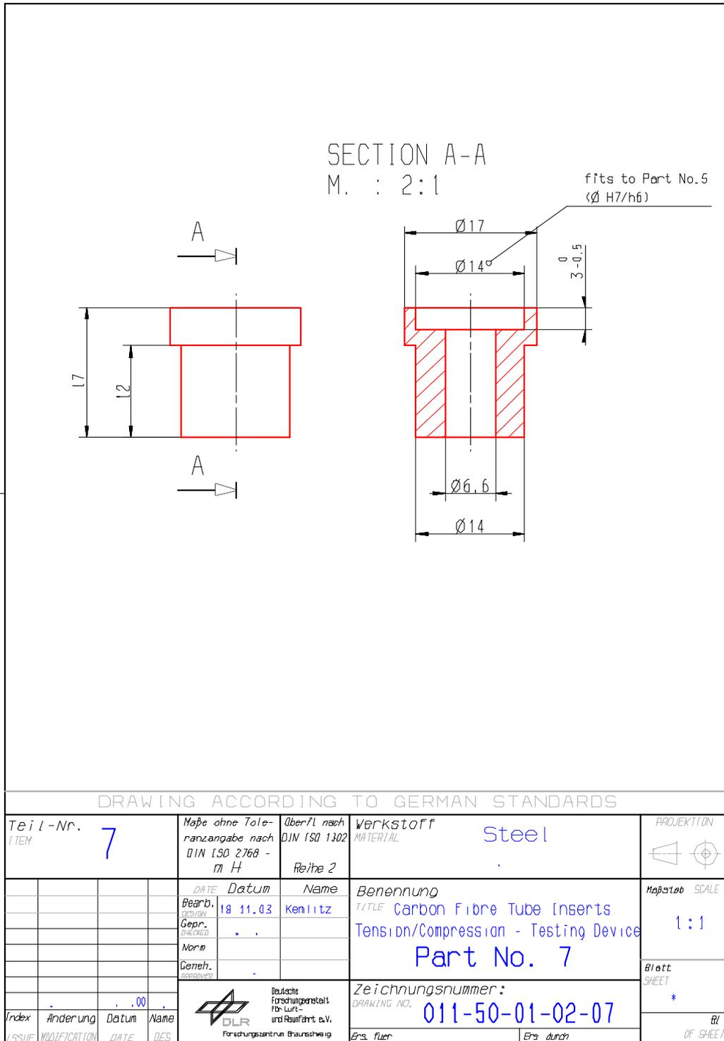
Figure H-8: Test fixture: Tension-compression load – part 7
