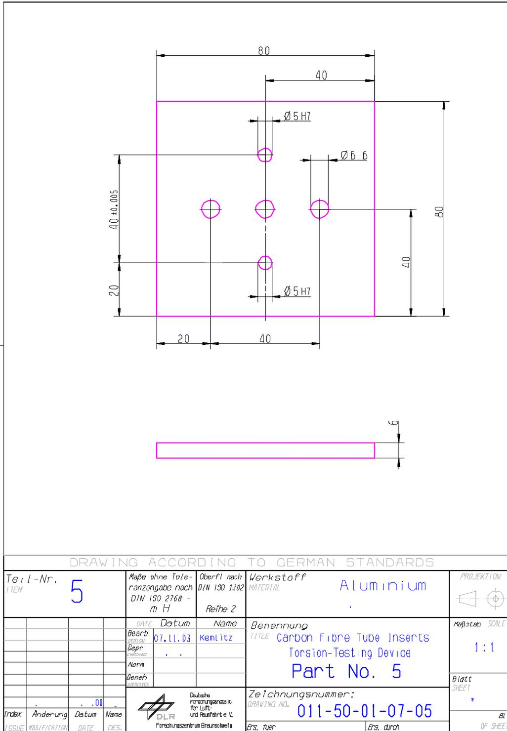
Figure H-36: Test fixture: Torsion – part 5
