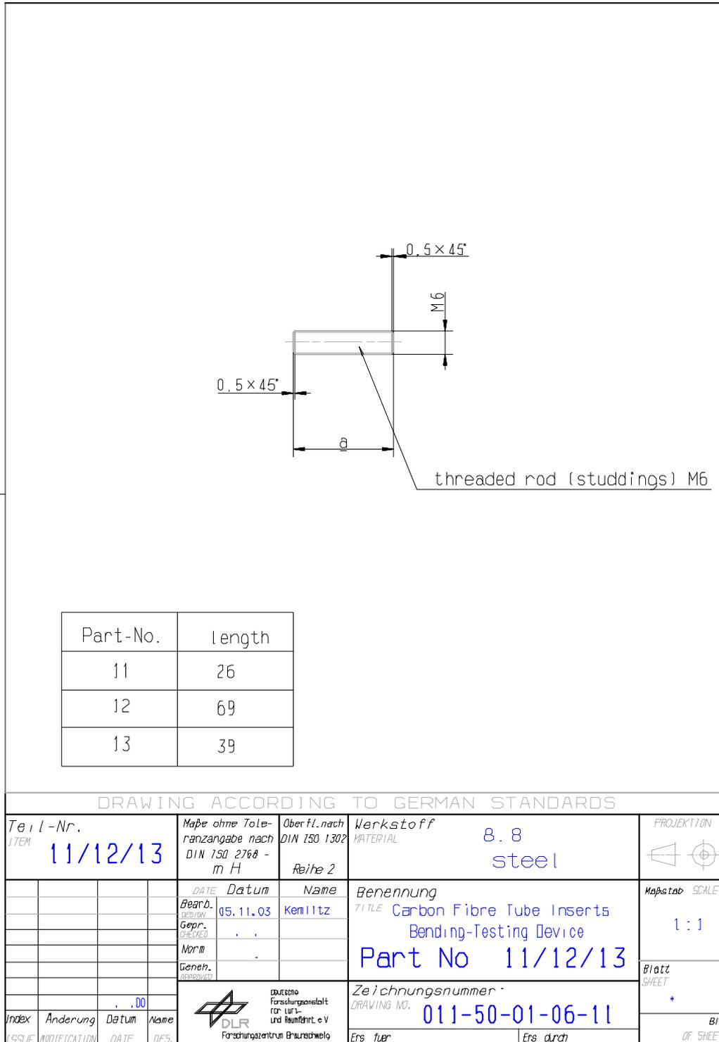
**Figure H-29: Test fixture: Bending – parts 11, 12 and 13**
