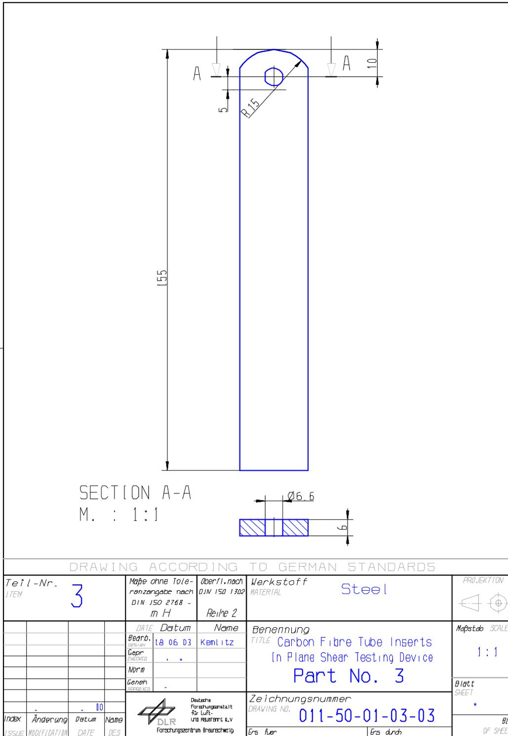
Figure H-12: Test fixture: In-plane shear load – part 3
