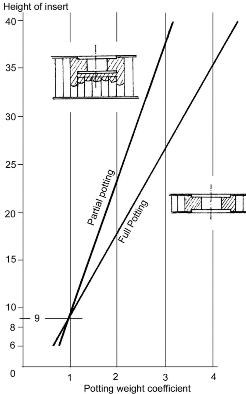
Figure 7-6: Correction coefficient for weight of insert heights
