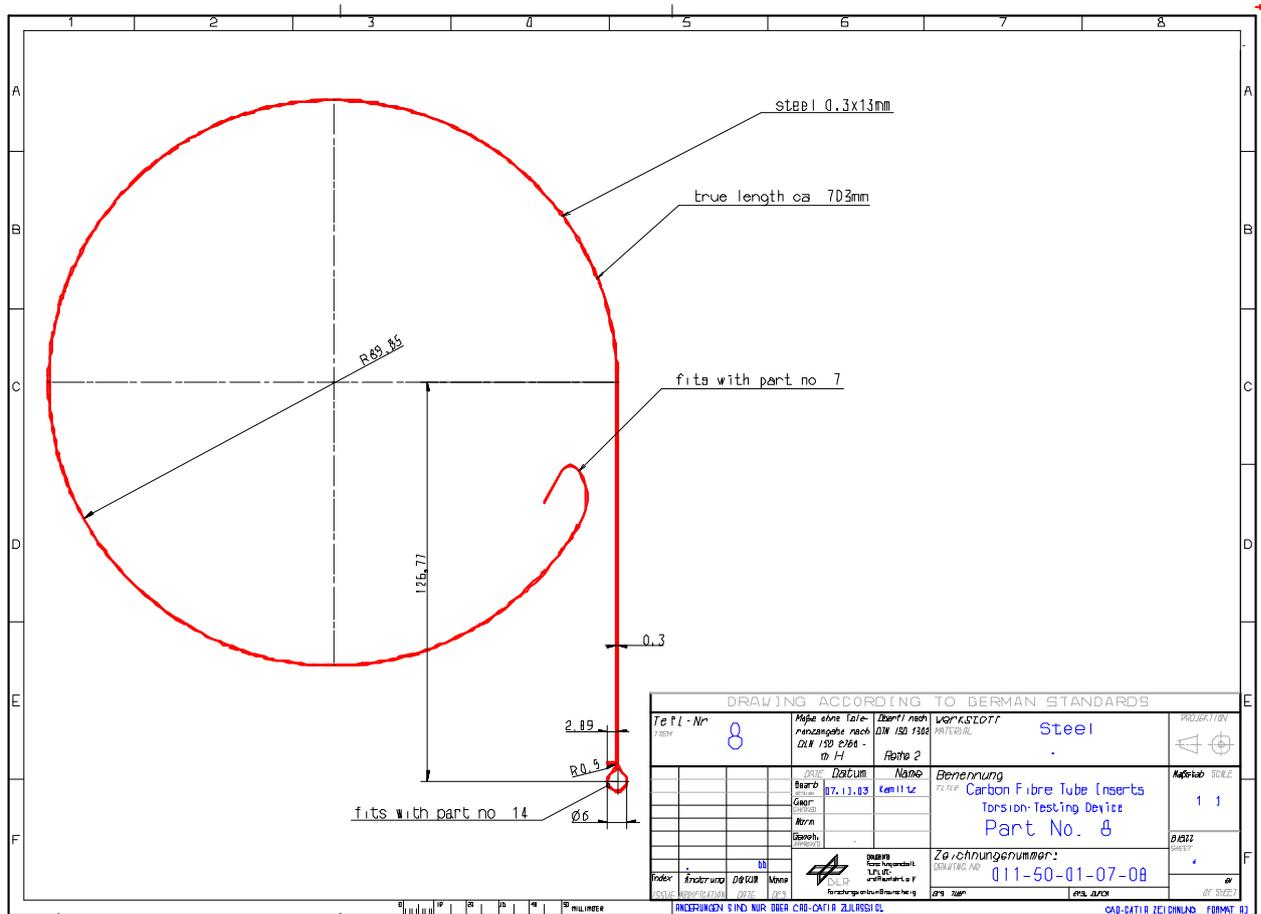
Figure H-39: Test fixture: Torsion – part 8
