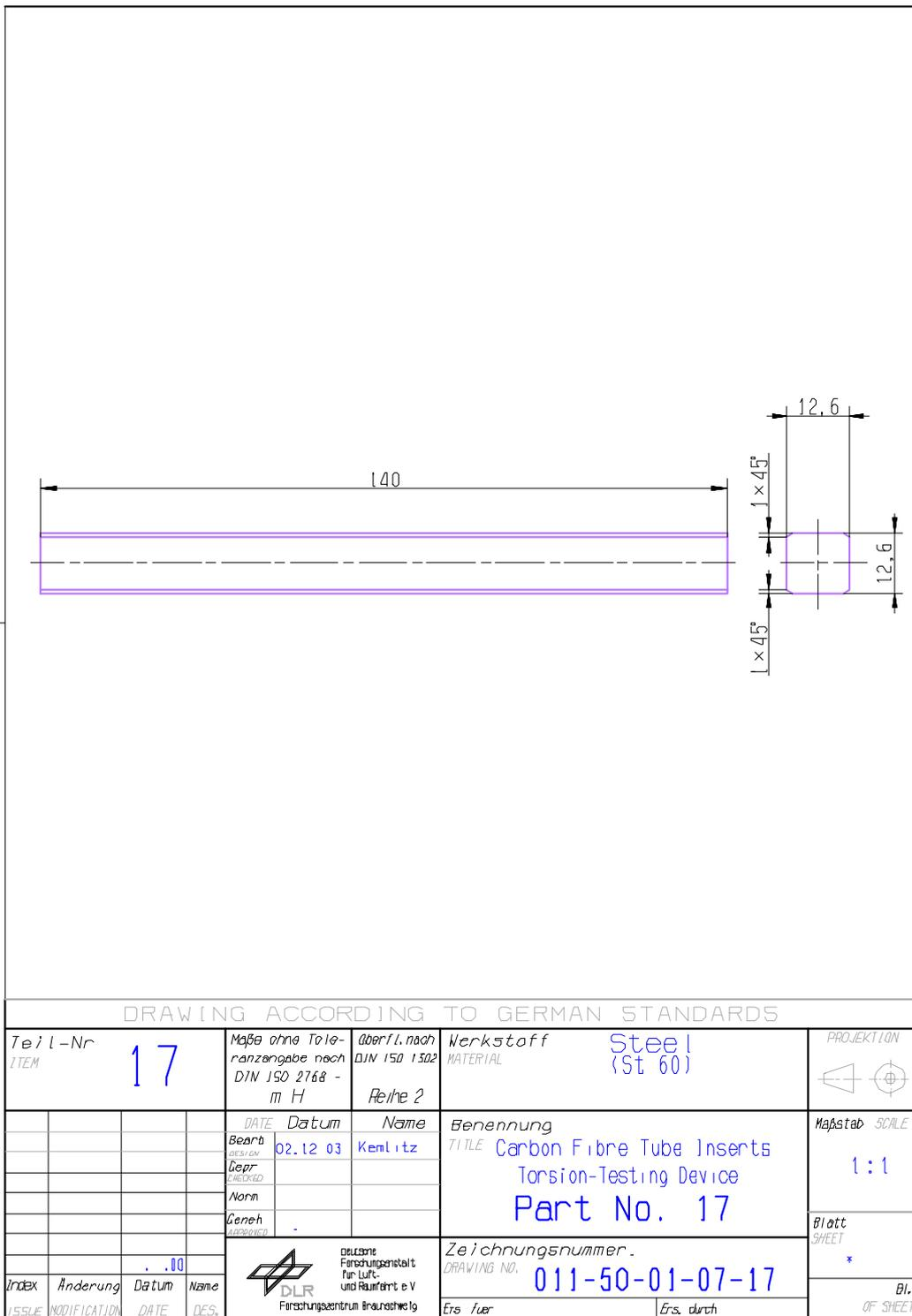
Figure H-48: Test fixture: Torsion – part 17
