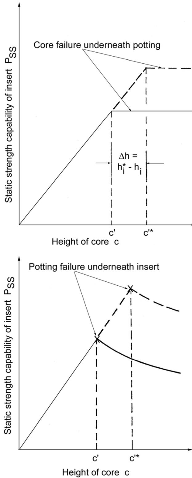
Figure 12-4: Influence of insert height on insert capability
