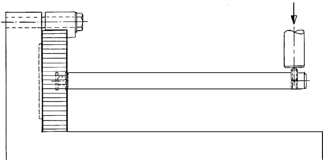
Figure 29-4: Testing: Bending fixture
