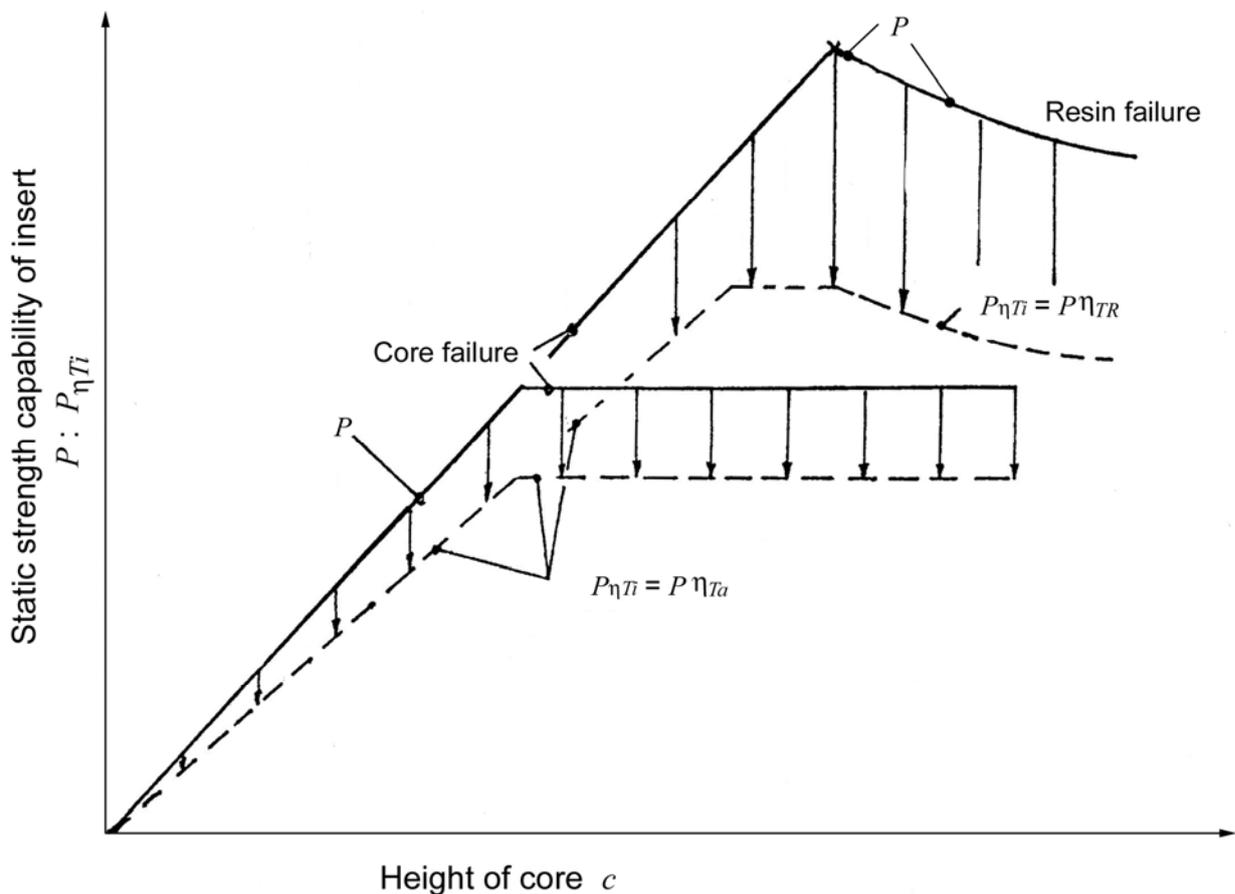
Figure 22-3: Thermal effects: Coefficient of thermal degradation
