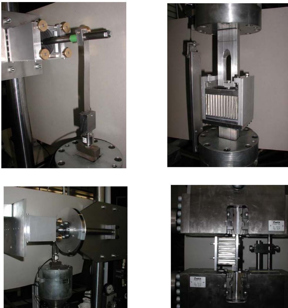
Bending and tension-compression tests (top row)
