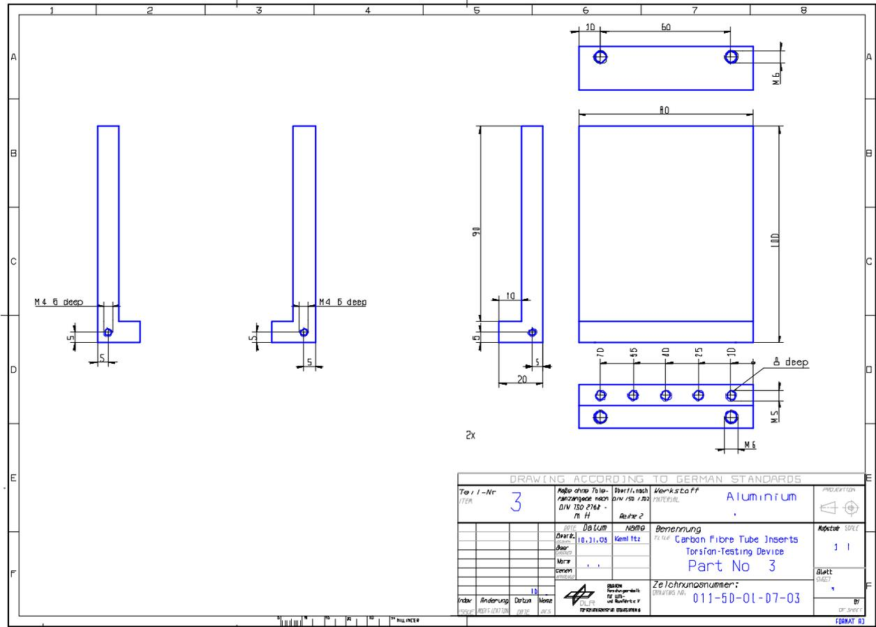
Figure H-34: Test fixture: Torsion – part 3
