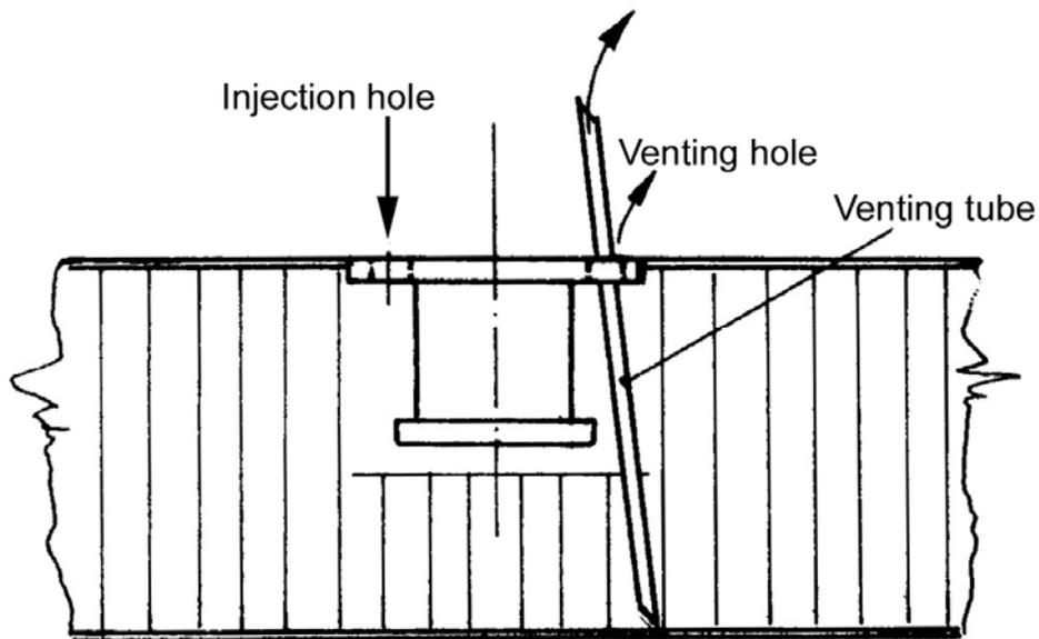
Figure 23-3: Venting of non-perforated core
