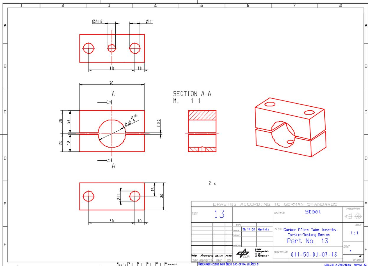
Figure H-44: Test fixture: Torsion – part 13
