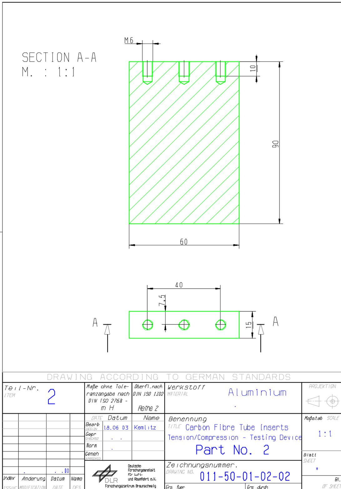
Figure H-3: Test fixture: Tension-compression load – part 2
