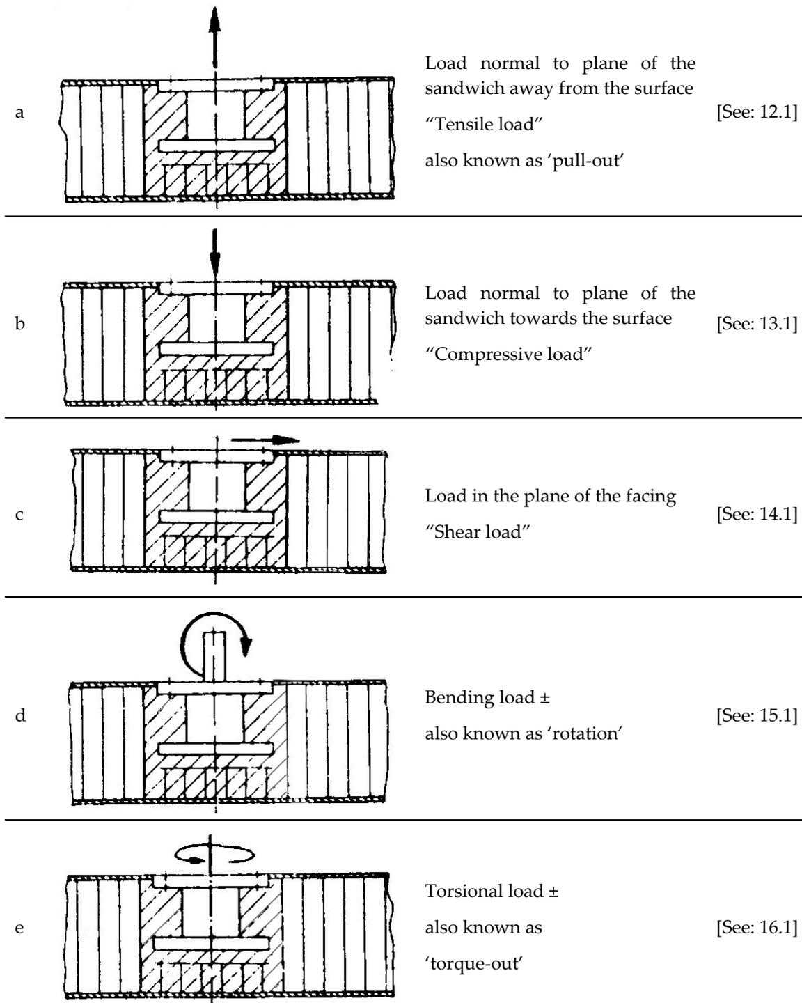
Figure 10-2: Insert load conditions
