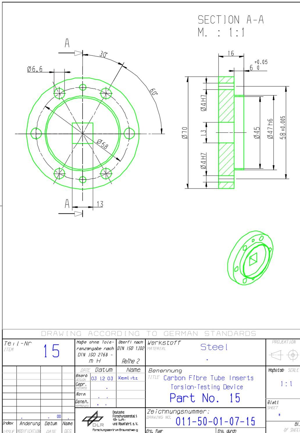
Figure H-46: Test fixture: Torsion – part 15
