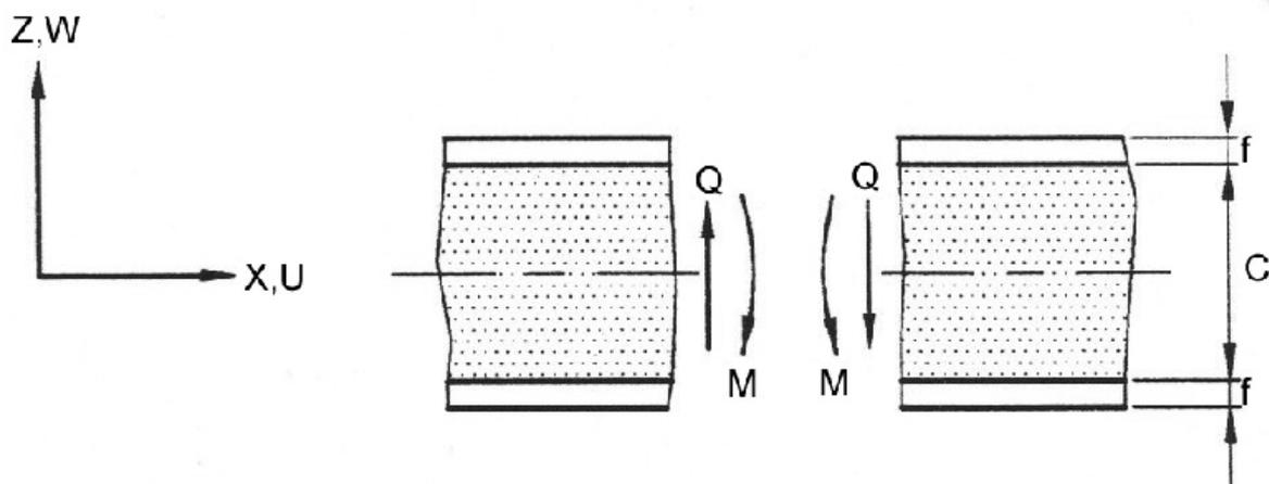
**Figure 8-2: Sign conventions for sandwich beam element**
