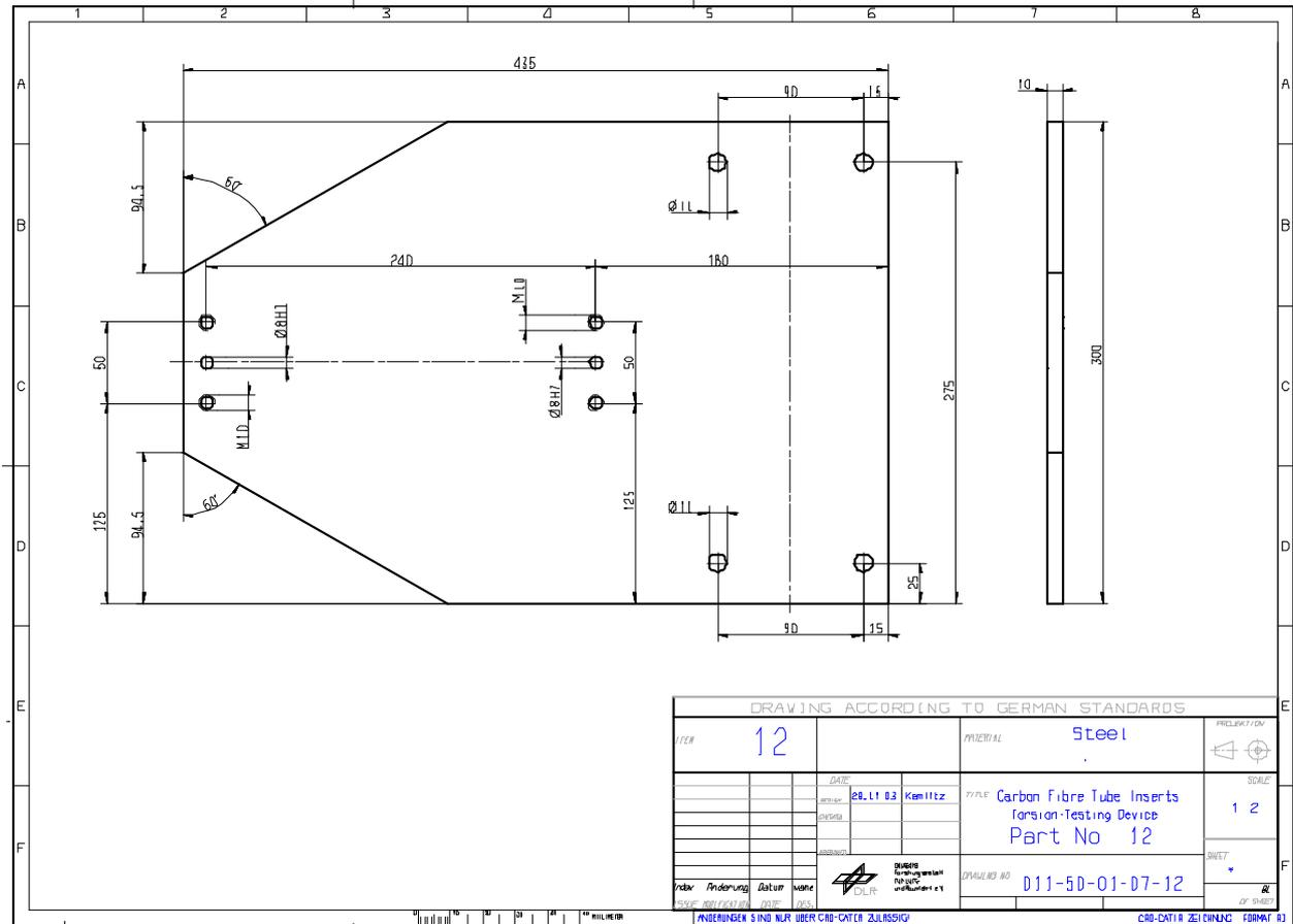
Figure H-43: Test fixture: Torsion – part 12
