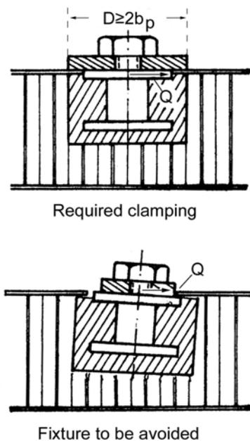
**Figure 14-1: Shear-loaded inserts: Clamping conditions**
