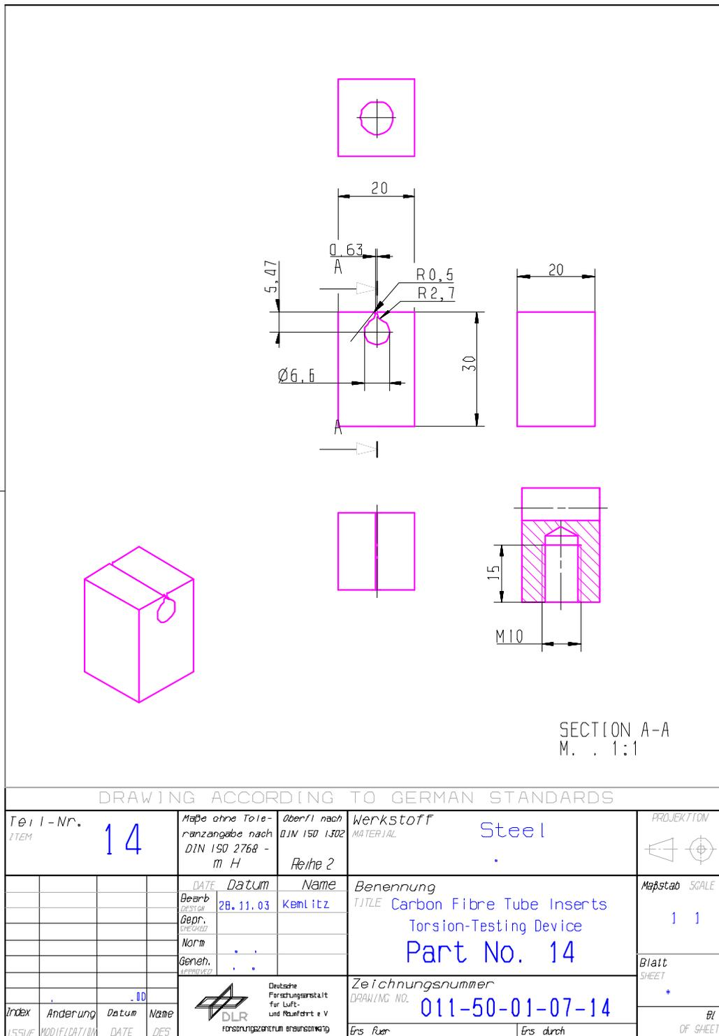
Figure H-45: Test fixture: Torsion – part 14
