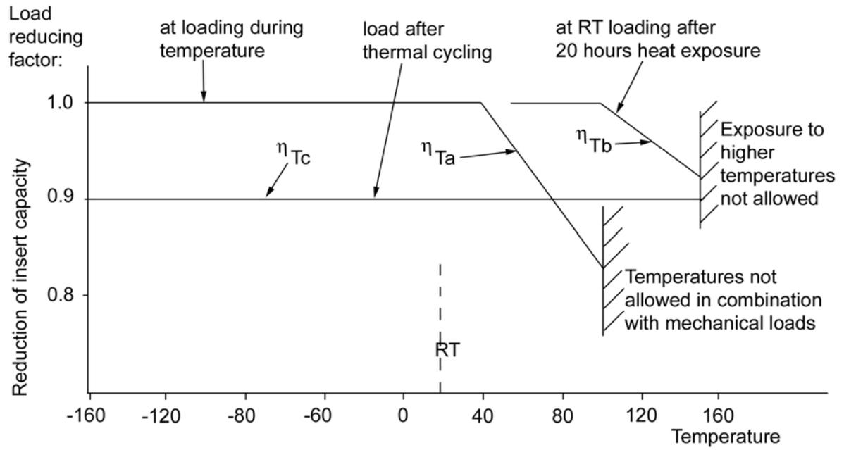
Figure 22-1: Thermal effects: Reduction of insert capability
