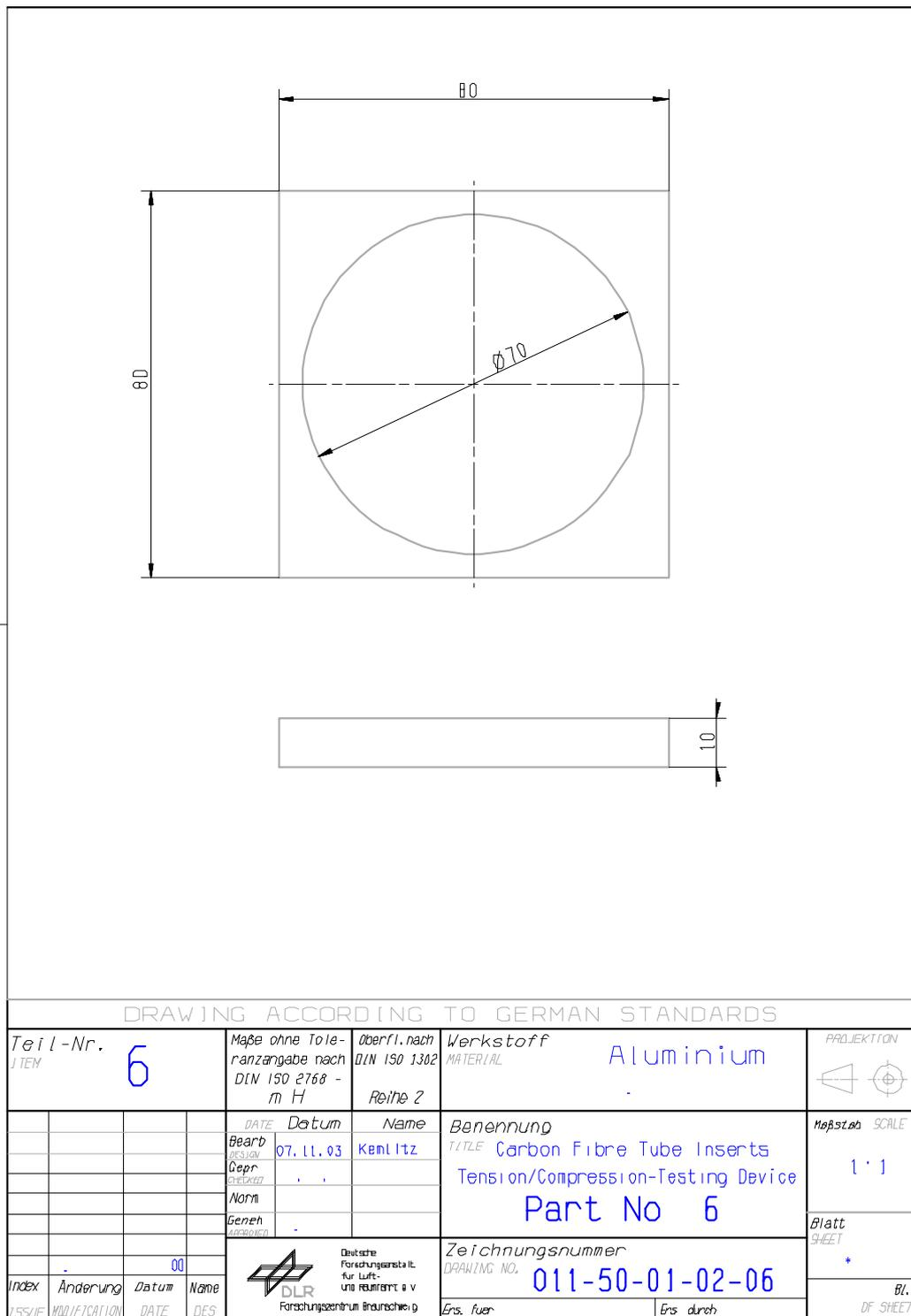
Figure H-7: Test fixture: Tension-compression load – part 6
