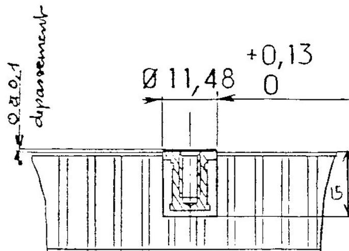
**Figure F-1: Case study: ARIANE 1 equipment bay / ASAP 4 - tensile (pull-out) test method**
