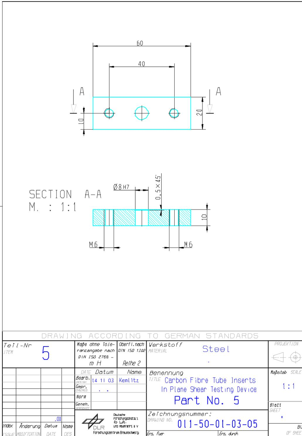
Figure H-14: Test fixture: In-plane shear load – part 5
