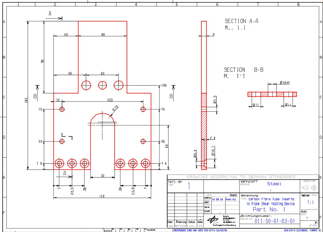
Figure H-10: Test fixture: In-plane shear load – part 1
