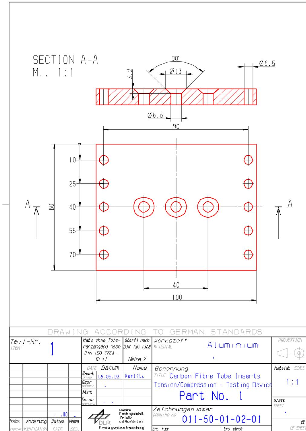
Figure H-2: Test fixture: Tension-compression load – part 1
