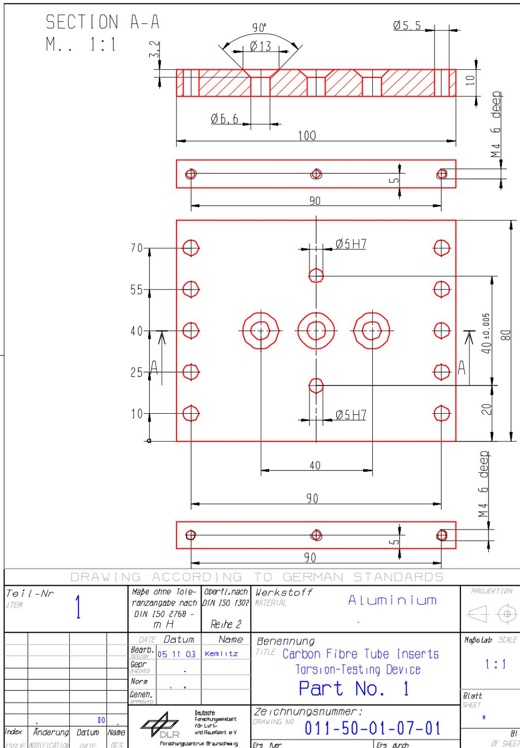
Figure H-32: Test fixture: Torsion – part 1
