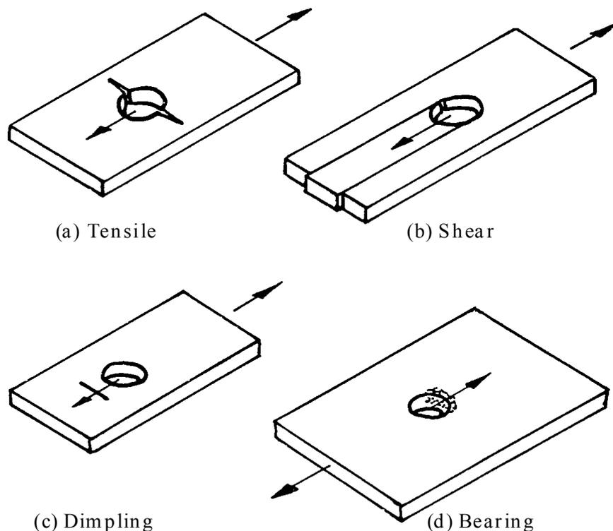
**Figure 10-20: Failure modes: CFRP face sheets**
