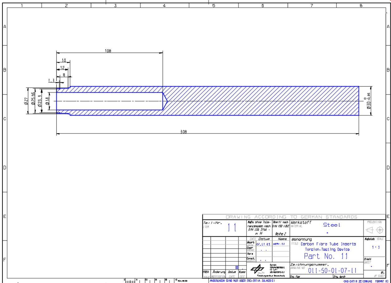
Figure H-42: Test fixture: Torsion – part 11
