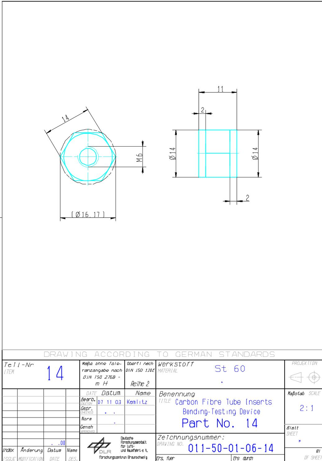
Figure H-30: Test fixture: Bending – part 14
