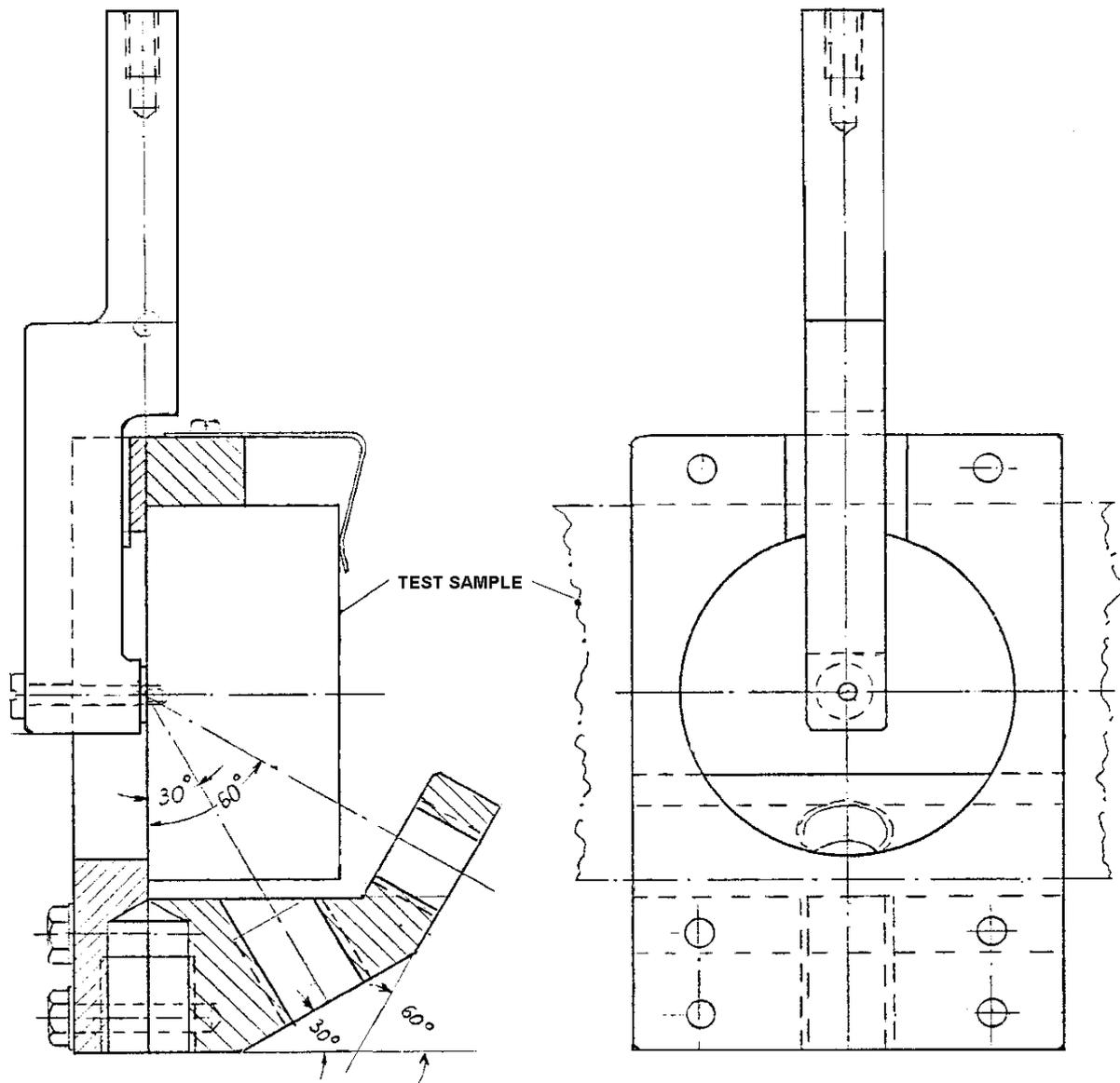
**Figure 29-2: Testing: Insert static in-plane strength fixture**
