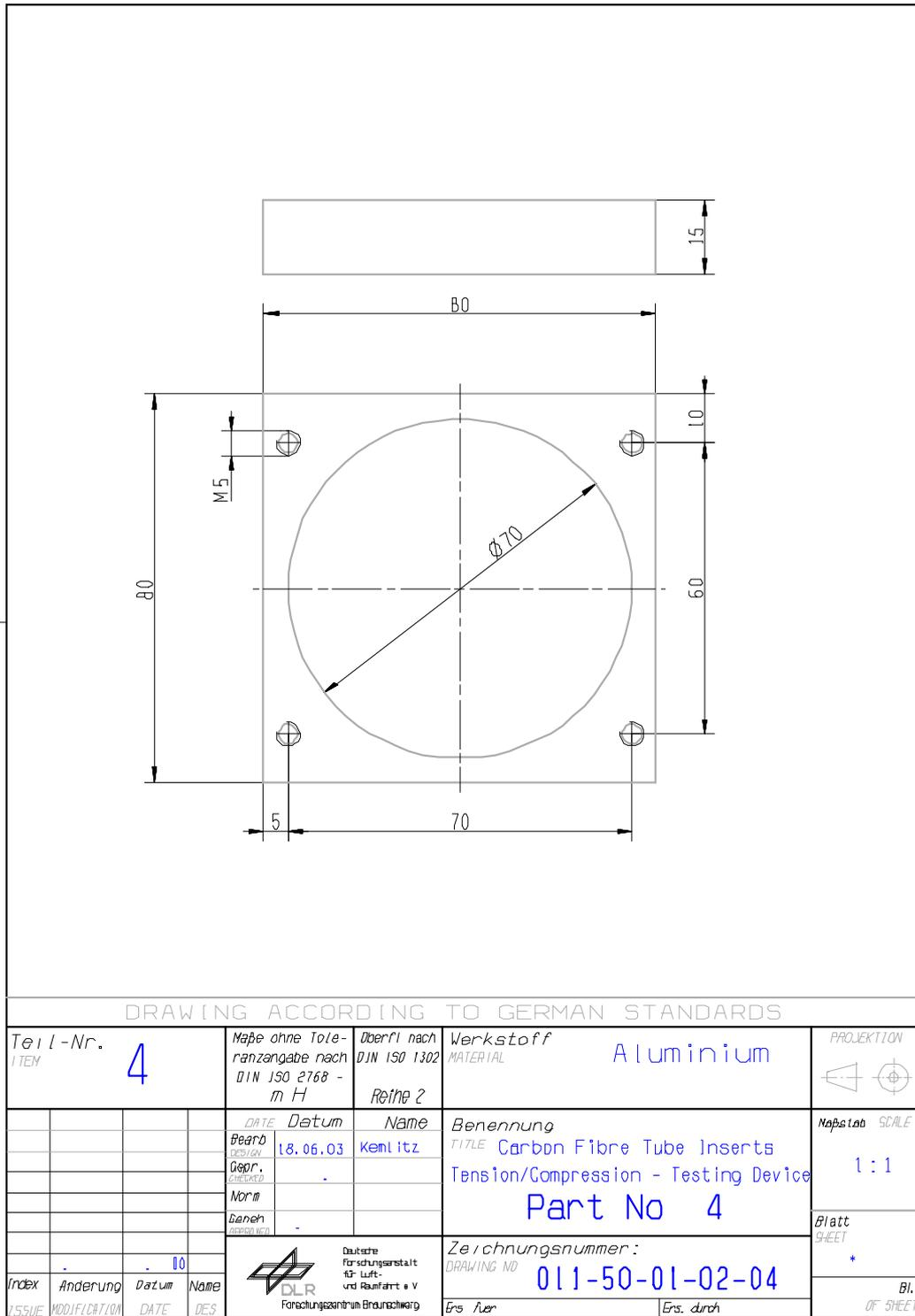
**Figure H-5: Test fixture: Tension-compression load – part 4**
