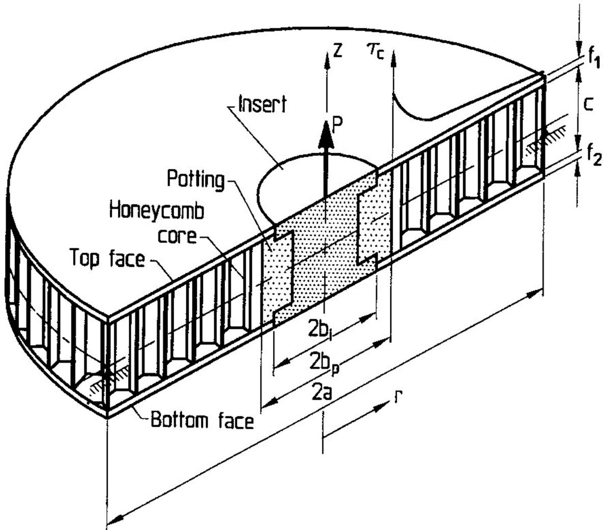
**Figure D-1 Out-of-plane loading: Circular sandwich plate with through-the-thickness insert**
