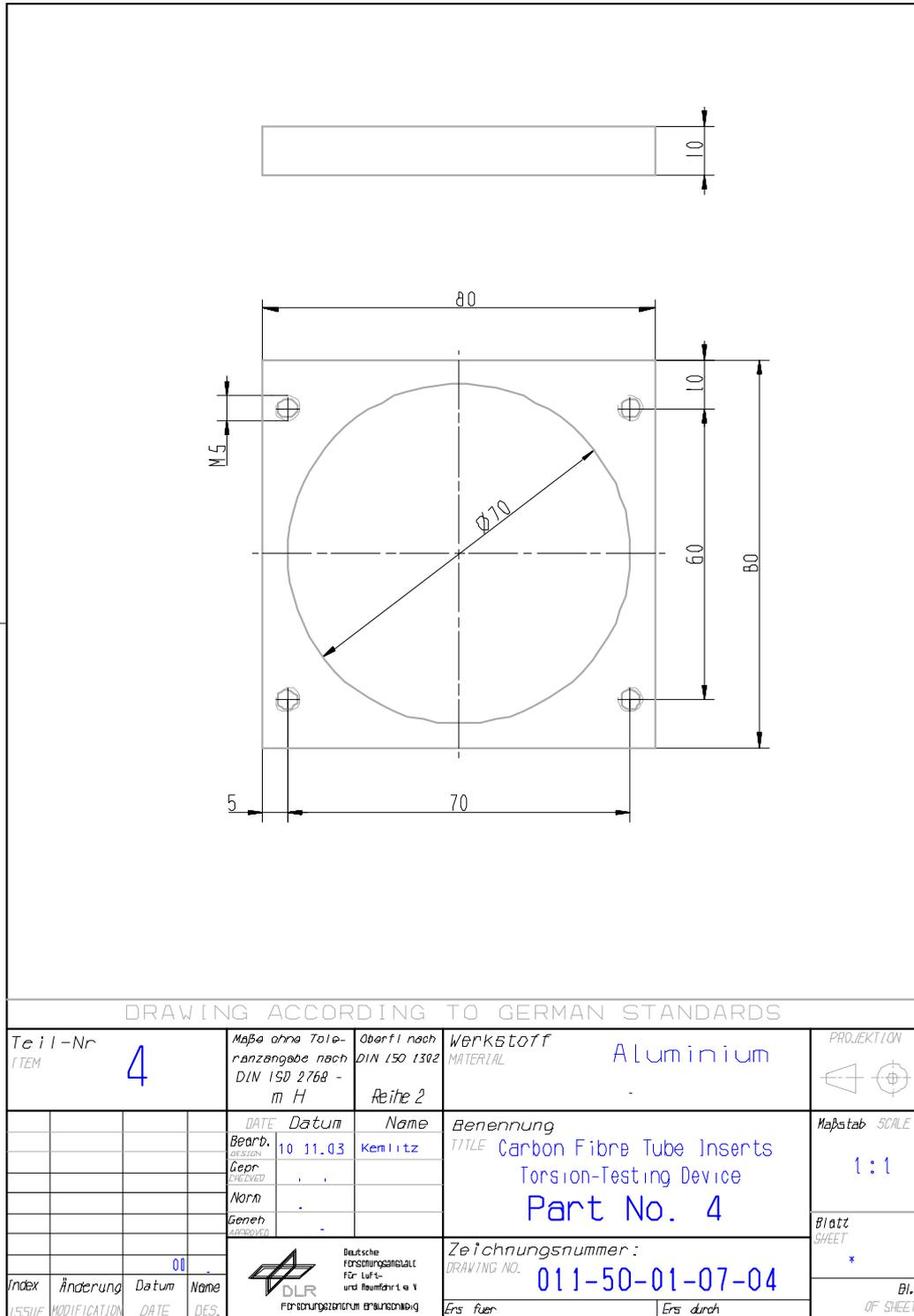
Figure H-35: Test fixture: Torsion – part 4
