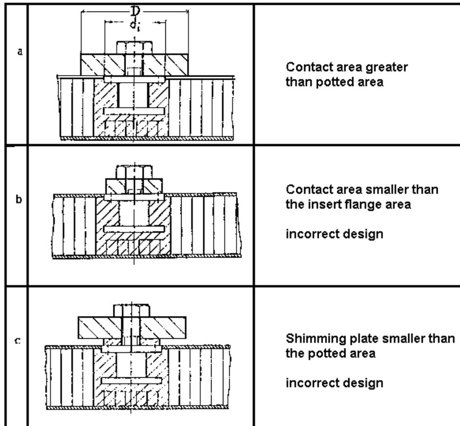
**Figure 10-3: Sandwich panel with metallic face sheets: General design rules**
