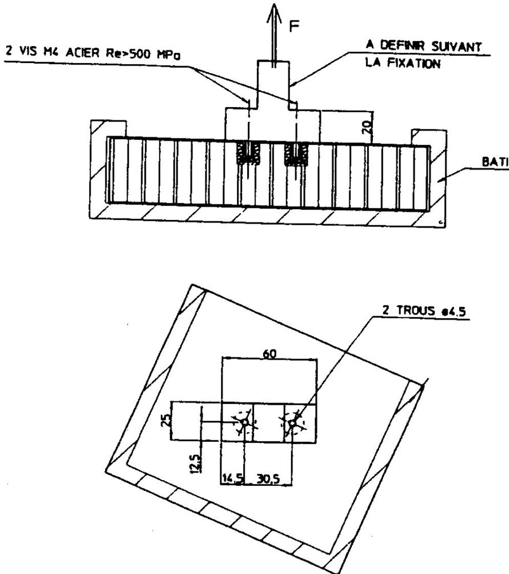
Figure F-9: Case study: ASAP 4 (AR4) - tensile (pull-out) method B
