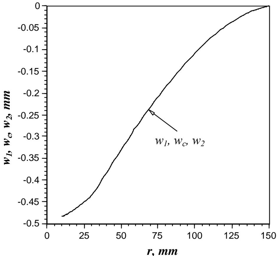
NOTE Out-of-plane displacements (core midsurface):  $w_1, w_2, w_c$ .
