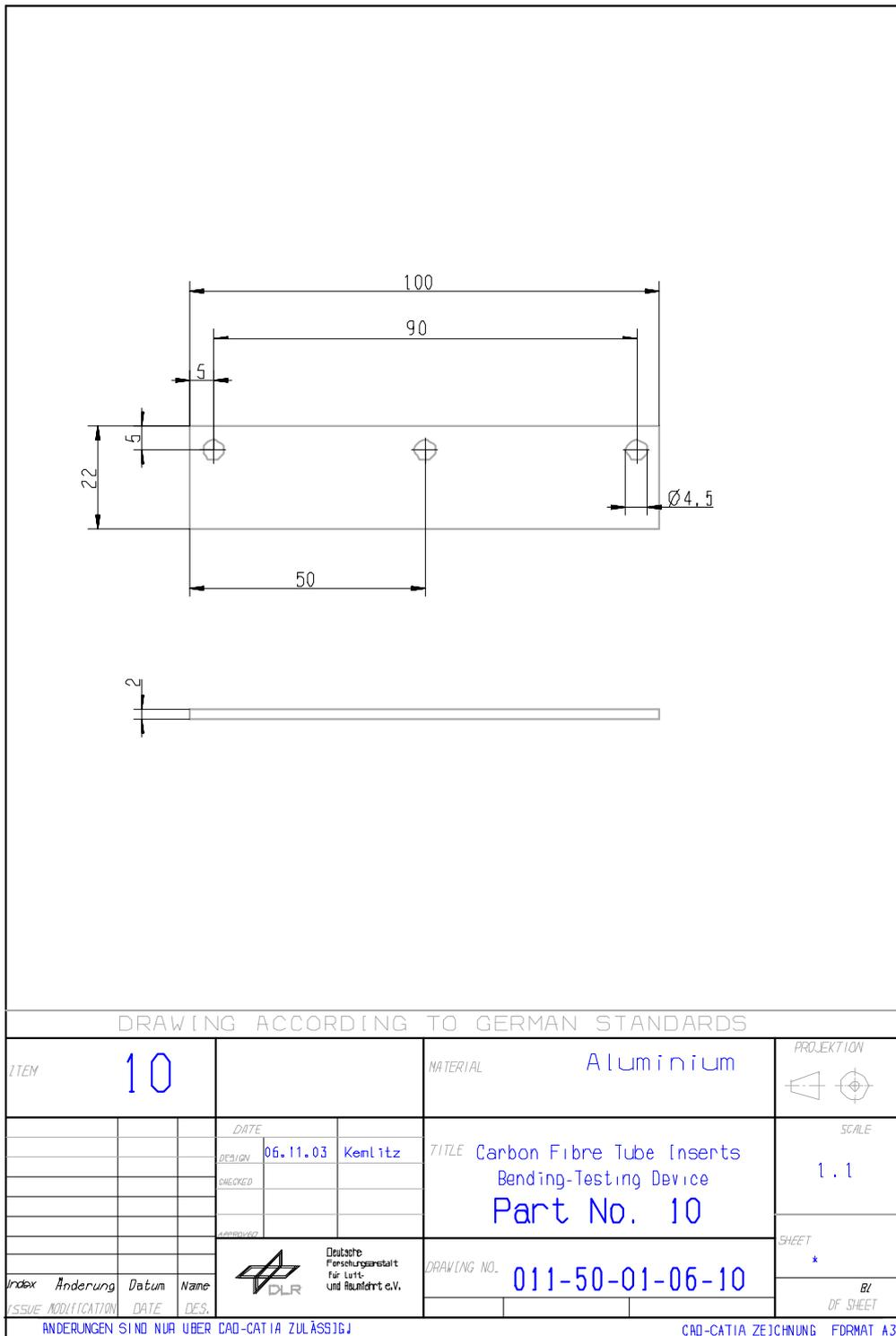
Figure H-28: Test fixture: Bending – part 10
