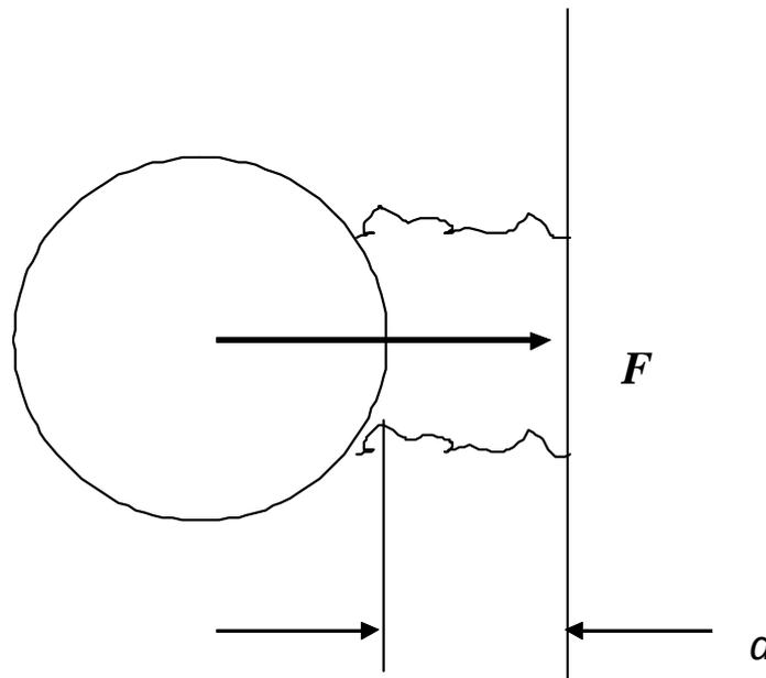
**Figure 10-12: Pre-design: Face sheet shear-out failure mode**
