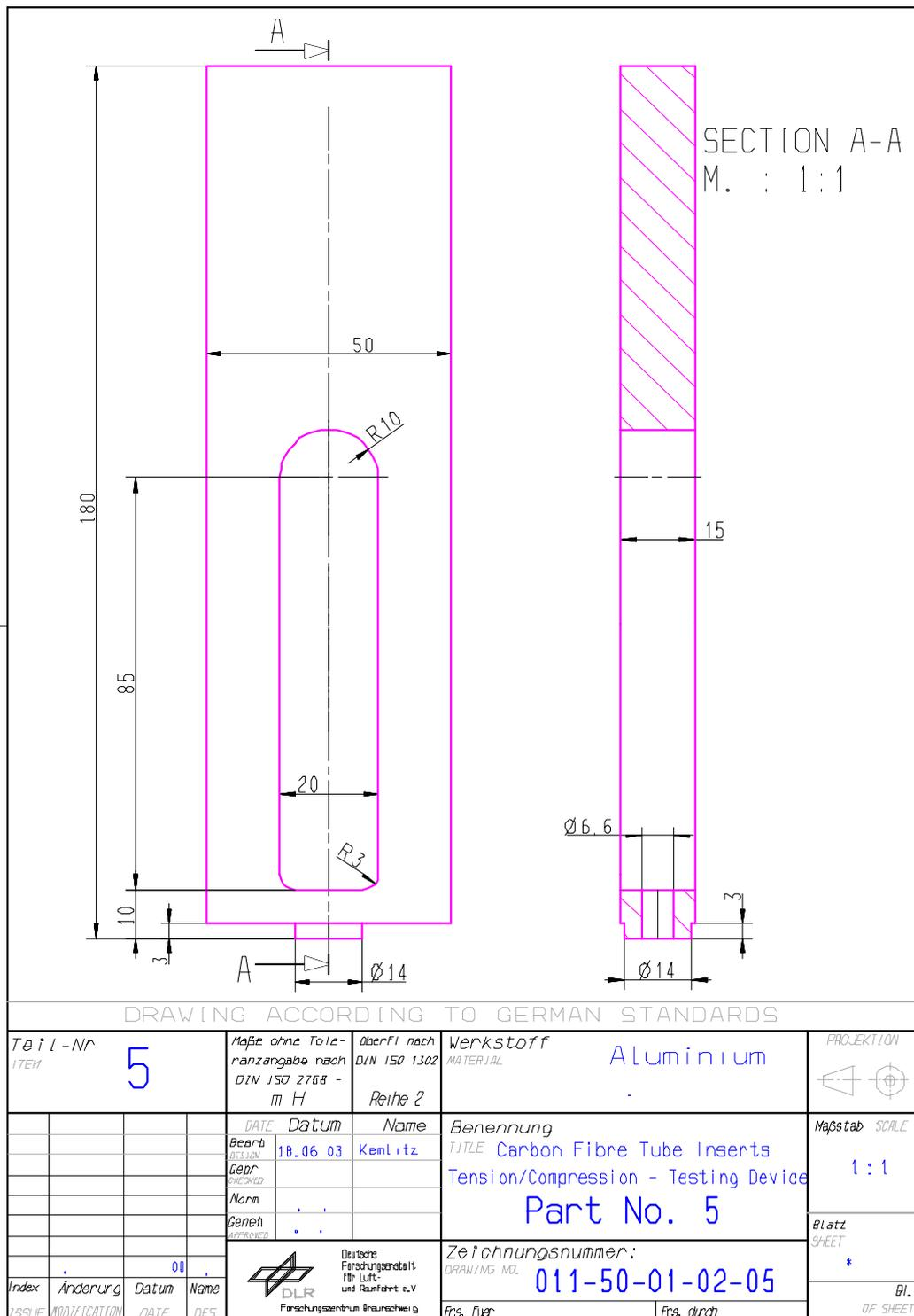
Figure H-6: Test fixture: Tension-compression load – part 5
