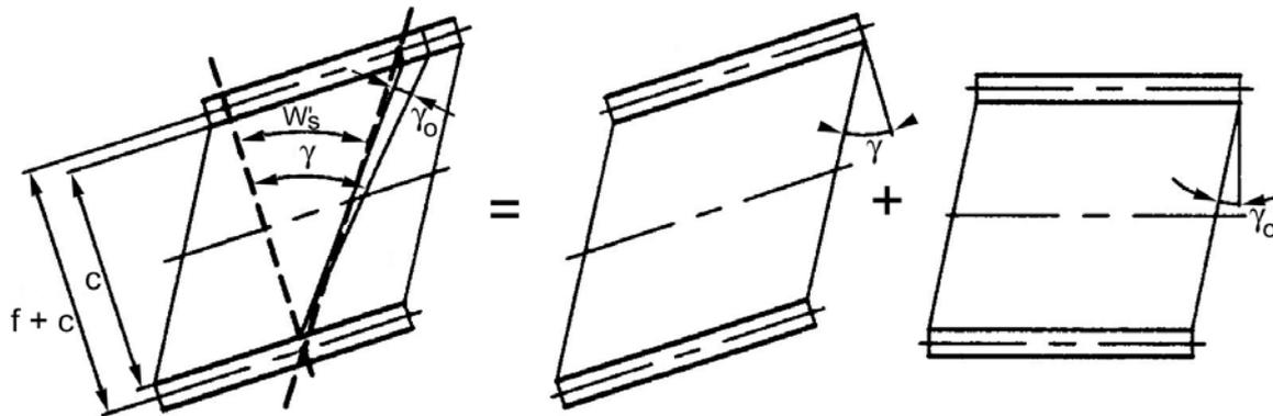
NOTE Shearing deformation of sandwich beam element ( $w'_s \equiv dw_s/dx$ ).
