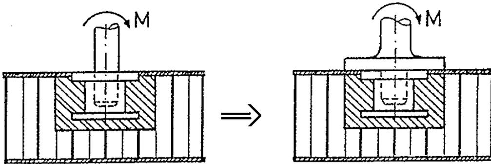
**Figure 15-3: Bending load: Insert footprint on moment loading**
