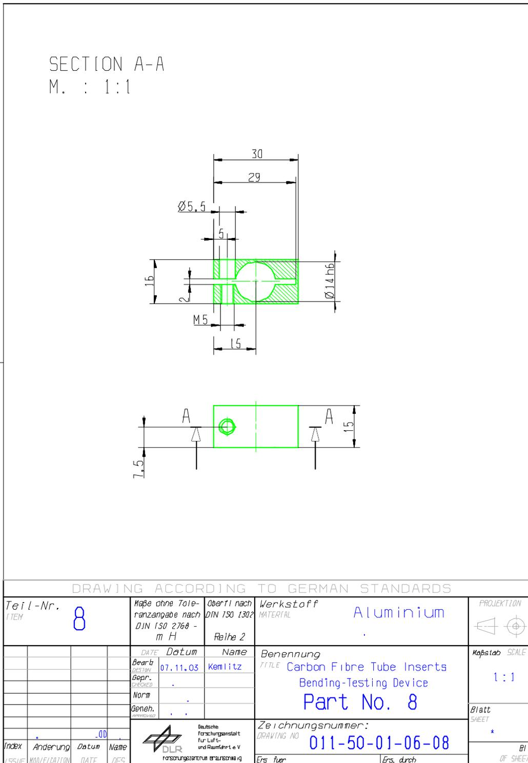
Figure H-26: Test fixture: Bending – part 8
