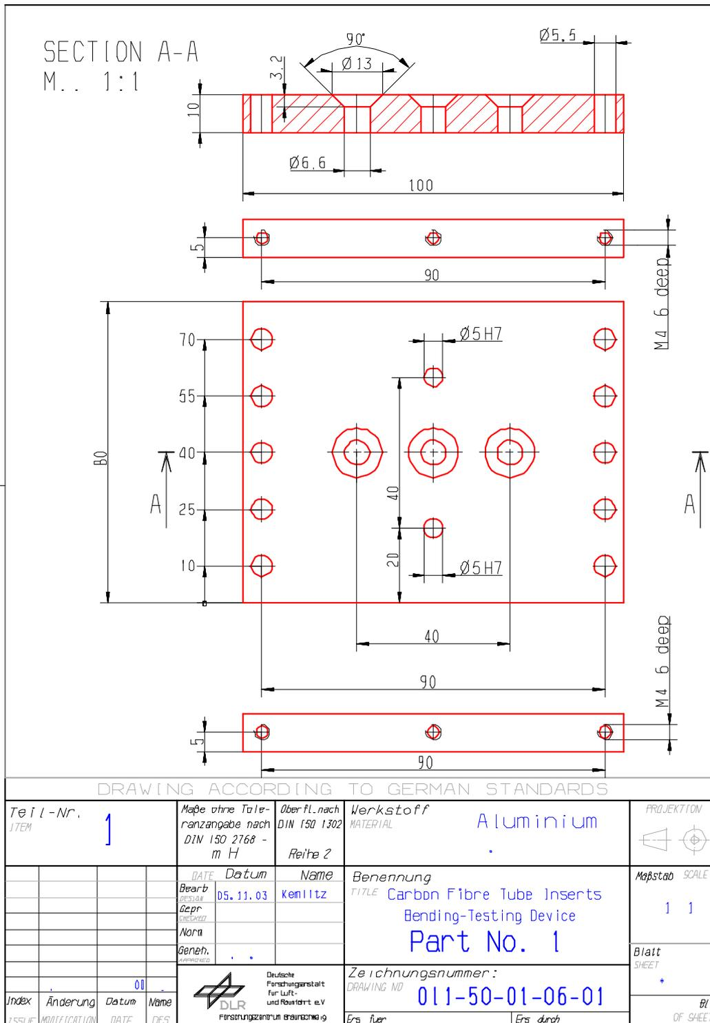
Figure H-19: Test fixture: Bending – part 1
