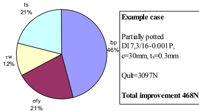
**Figure 14-9: In-plane capability: Contributions of the main components on improved core shear**
