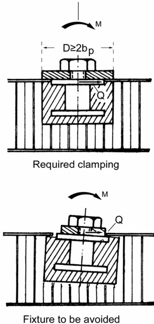
Figure 15-1: Inserts loaded in bending: Clamping conditions
