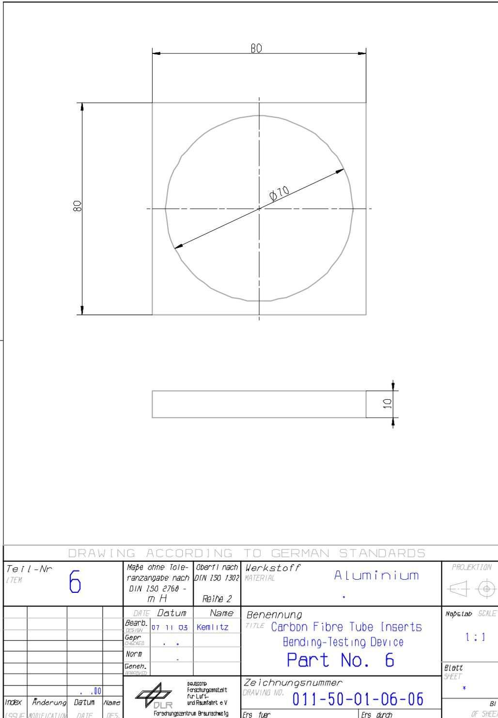
Figure H-24: Test fixture: Bending – part 6
