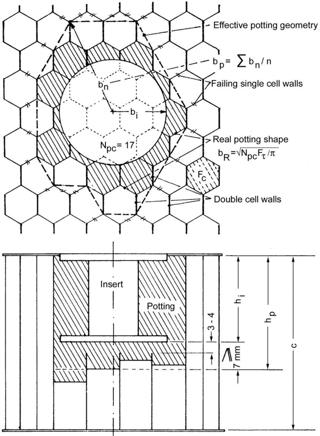
Figure 7-1: Potting geometry
