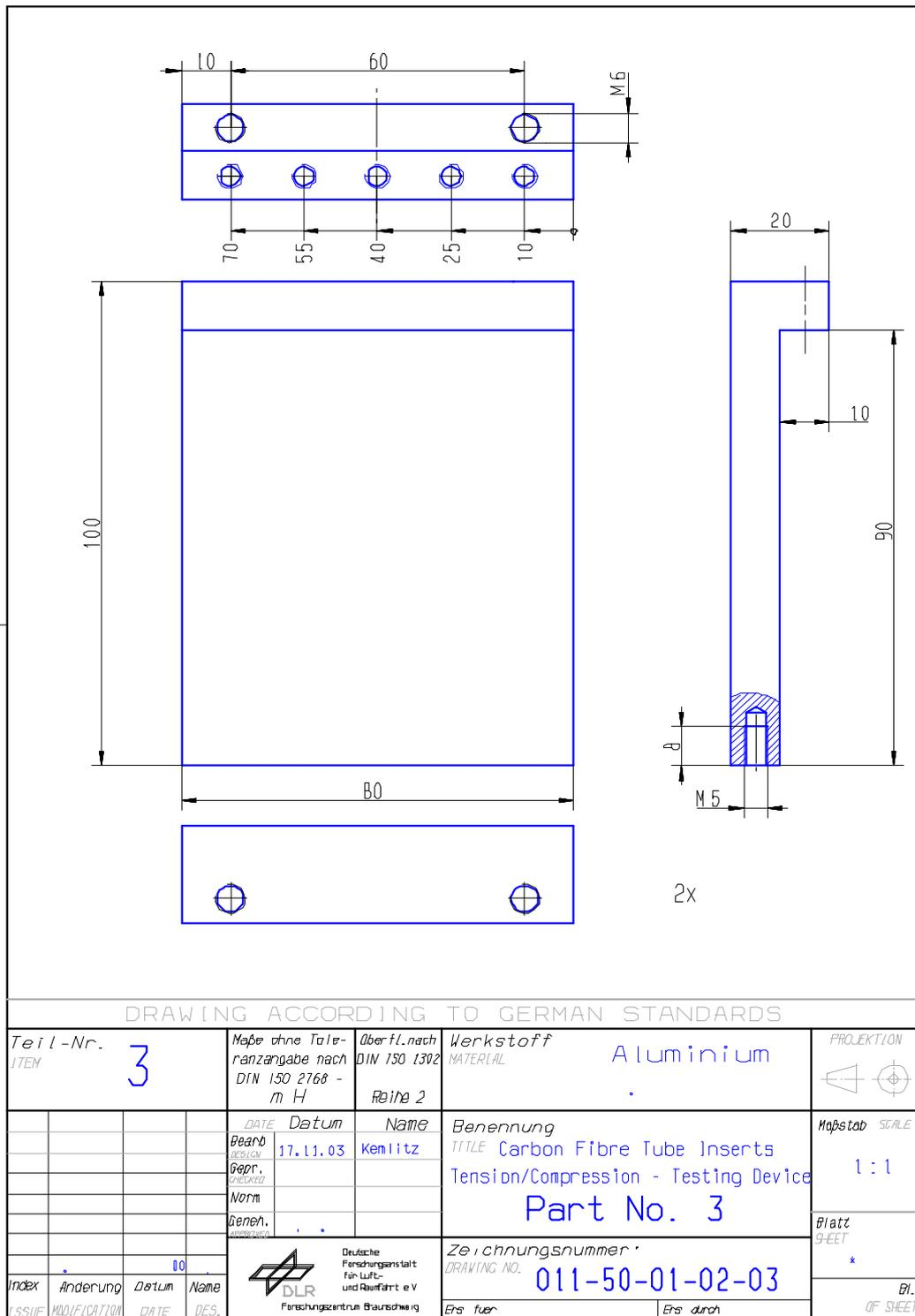
Figure H-4: Test fixture: Tension-compression load – part 3
