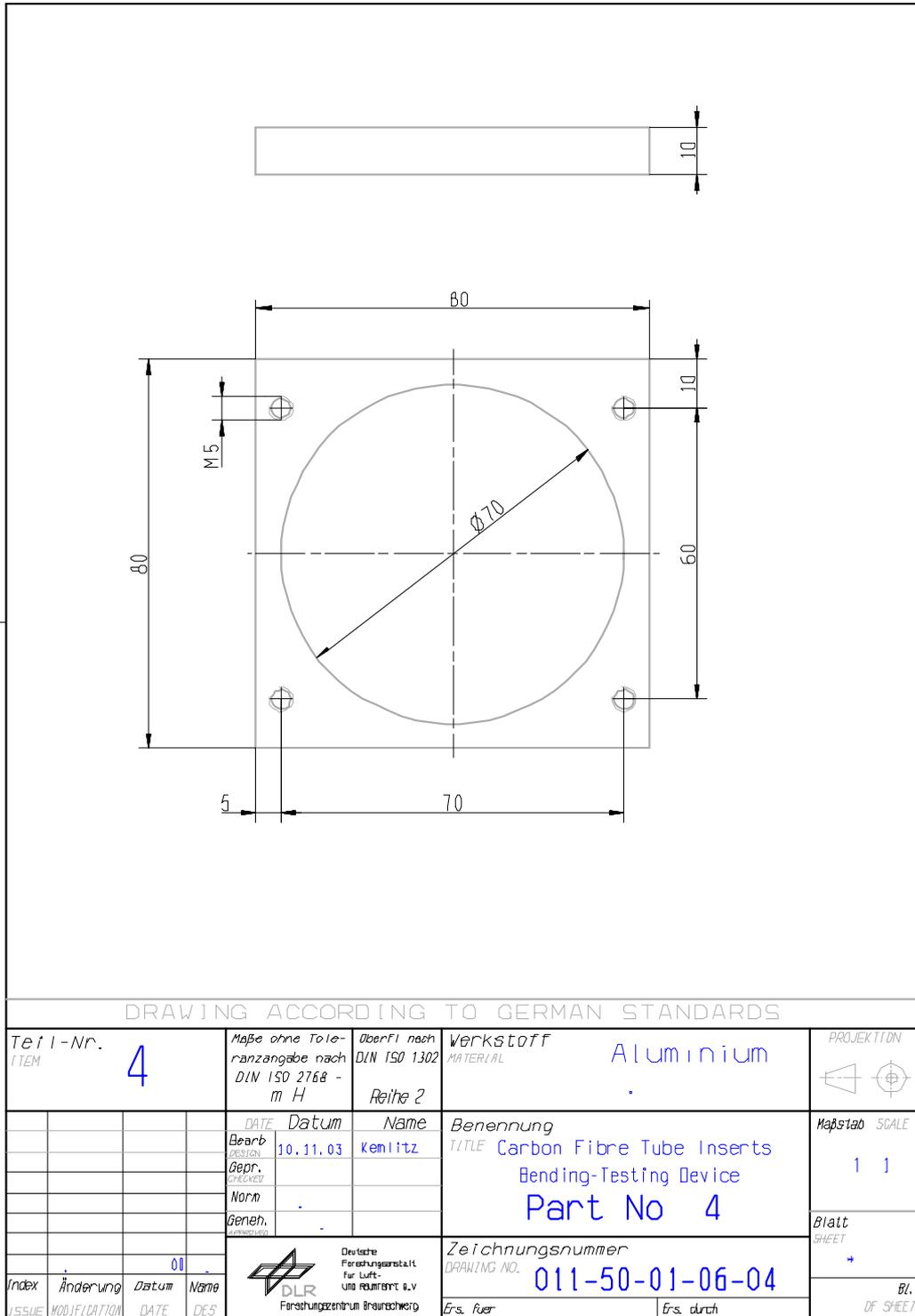
Figure H-22: Test fixture: Bending – part 4
