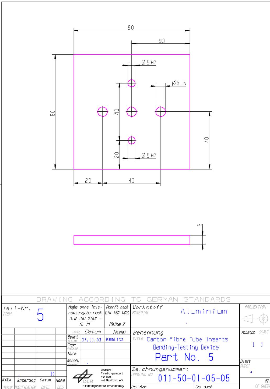
Figure H-23: Test fixture: Bending – part 5
