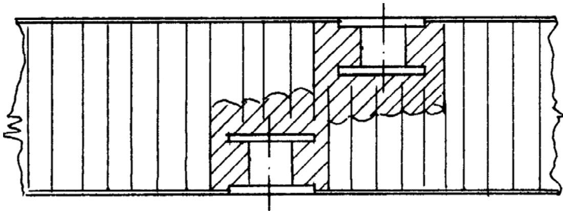
Figure 23-2: Inserts with connected potting mass
