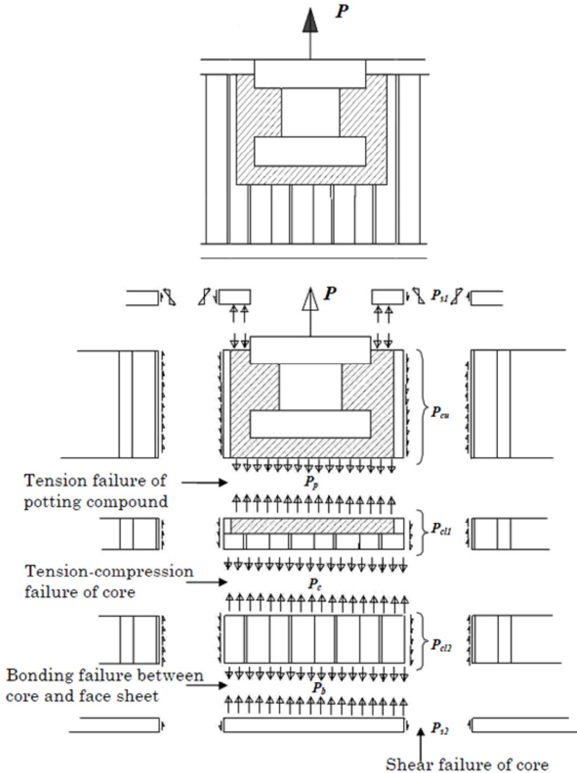
Figure 10-15: Failure modes: Load transfer in out-of-plane case
