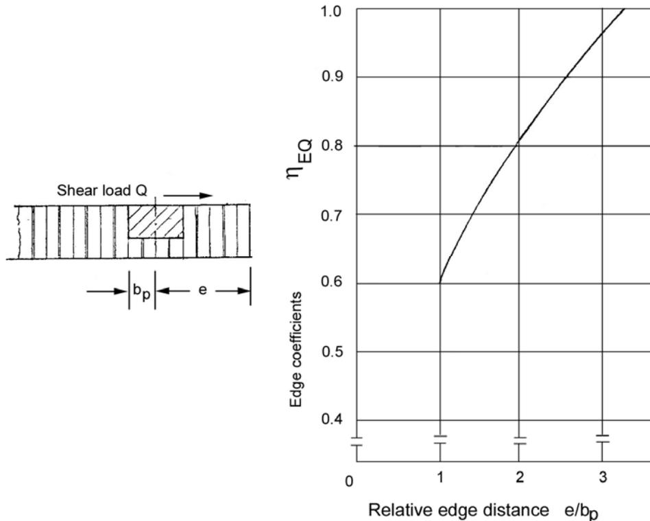
Figure 14-8: Shear strength: Influence of edge distance
