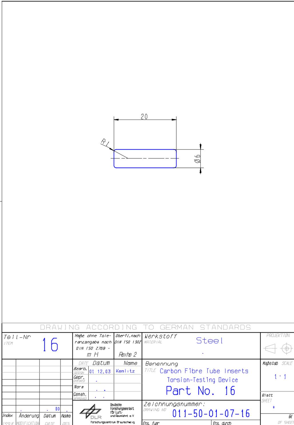
Figure H-47: Test fixture: Torsion – part 16
