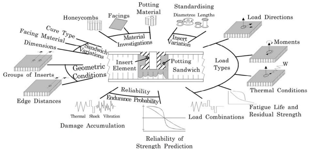
**Figure 9-1: Basic aspects of insert design, analysis and testing**
