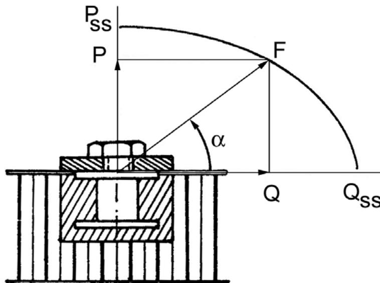
**Figure 17-1: Insert submitted to an inclined load**
