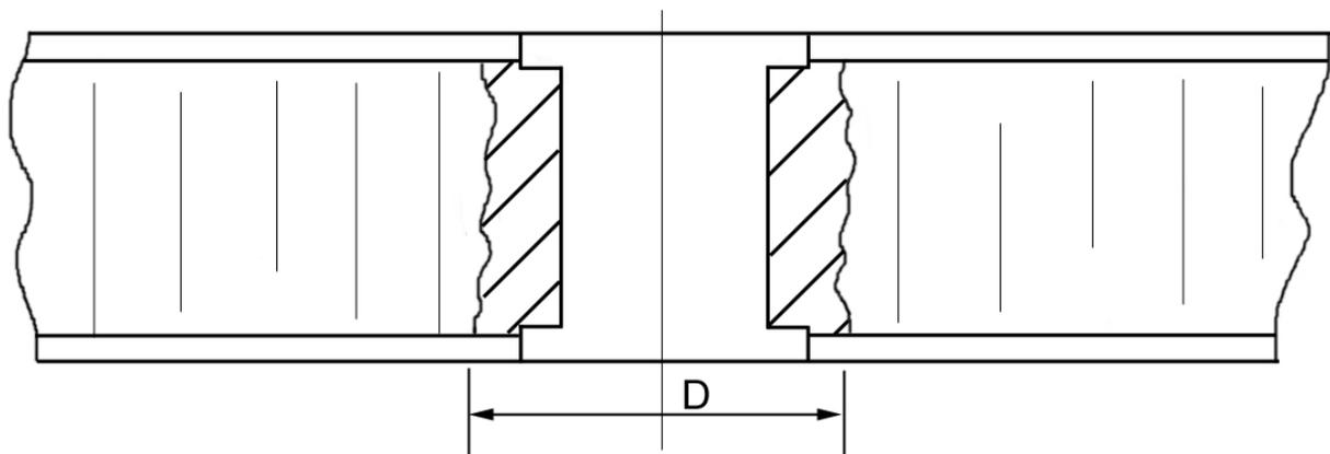
**Figure 10-13: Pre-design: Through-the-thickness insert under transverse force**
