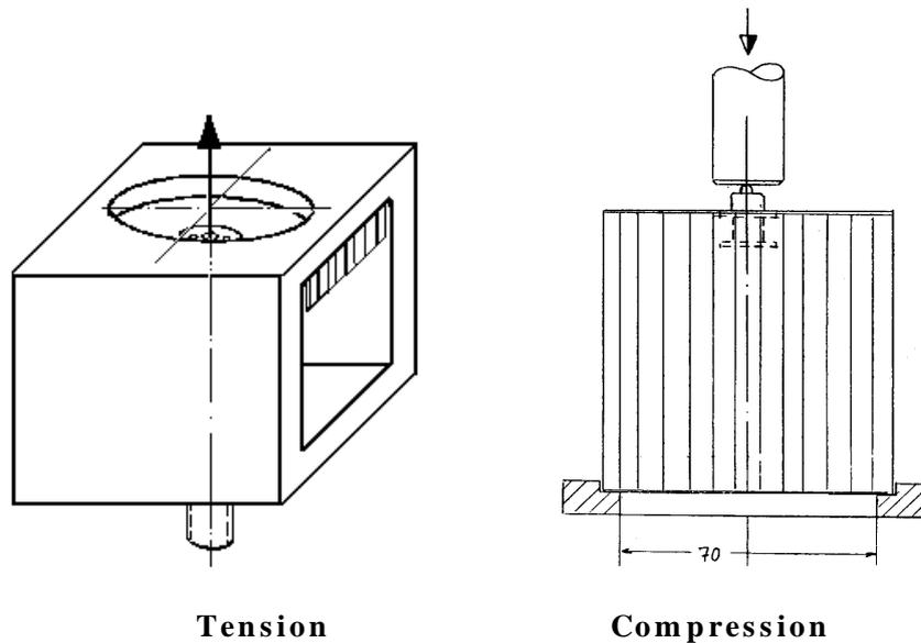
**Figure 29-1: Testing: Insert static out-of-plane strength fixture**
