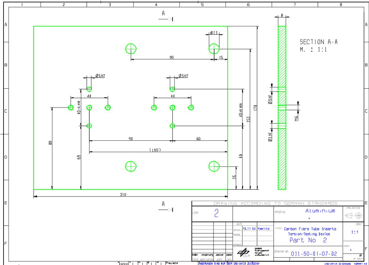
Figure H-33: Test fixture: Torsion – part 2
