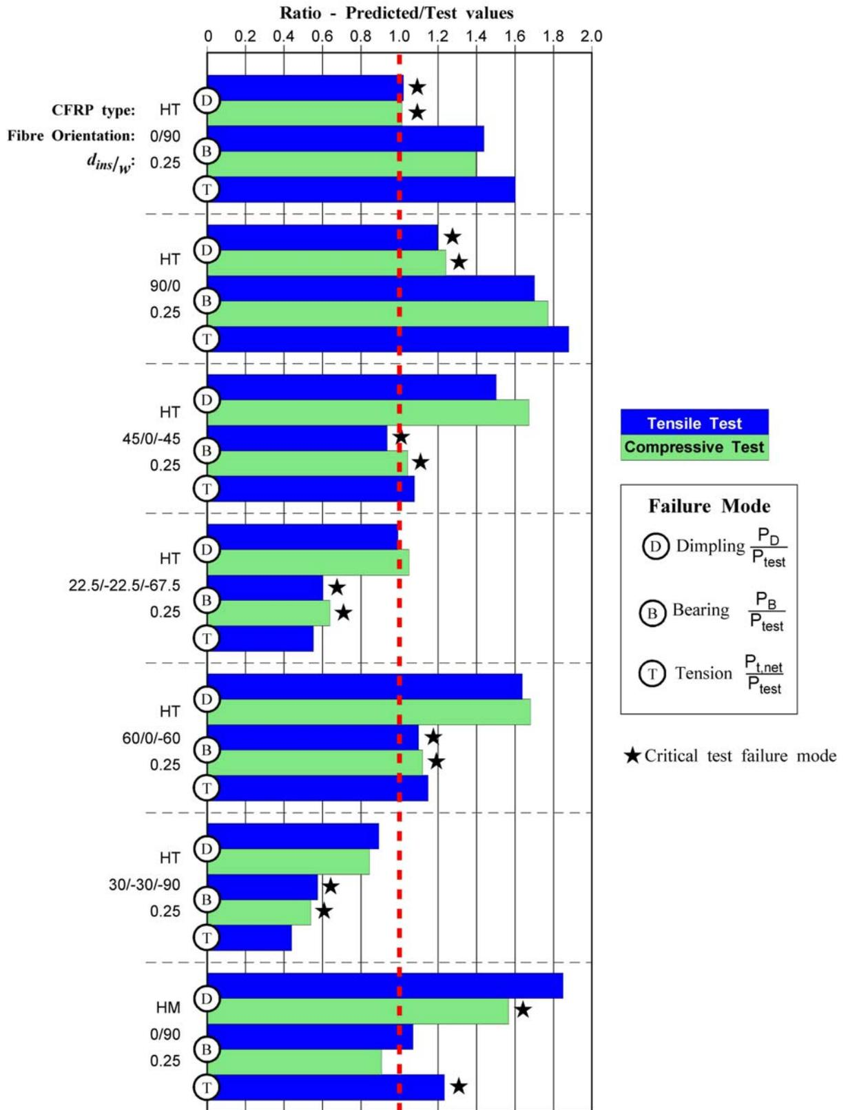
Figure 14-2: Correlation between calculated and tested in-plane capabilities with fibre orientation
