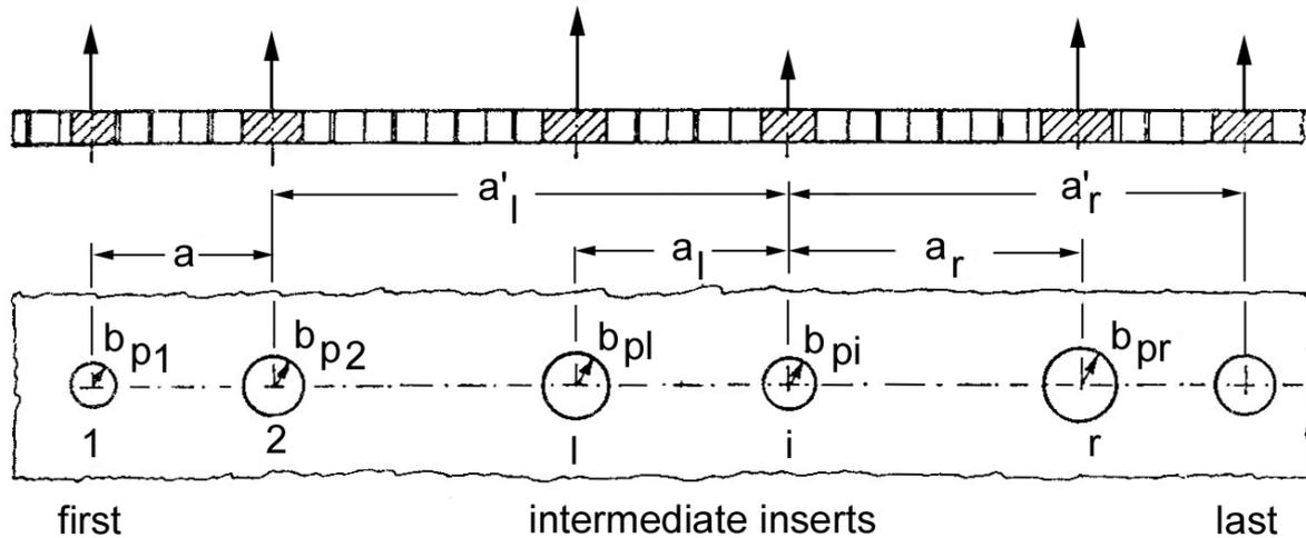
Figure 19-2: Insert groups: Series of inserts loaded in same direction
