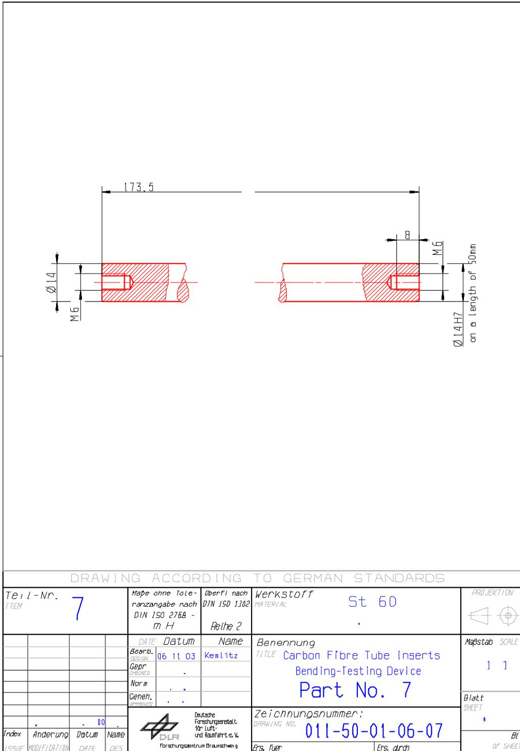
Figure H-25: Test fixture: Bending – part 7
