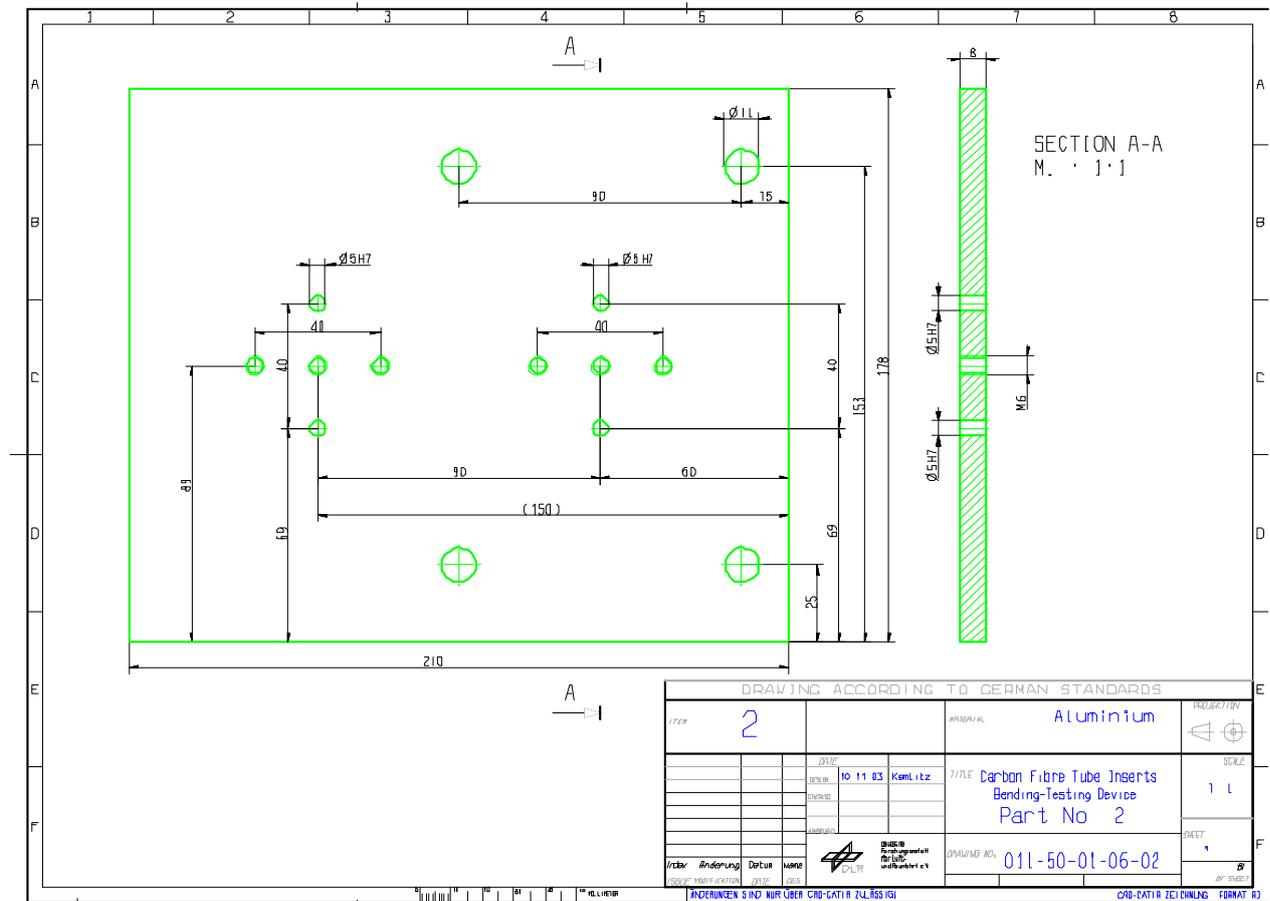
Figure H-20: Test fixture: Bending – part 2
