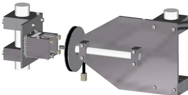
**Figure 27-5: Manufacture control: Torsion test fixture**
