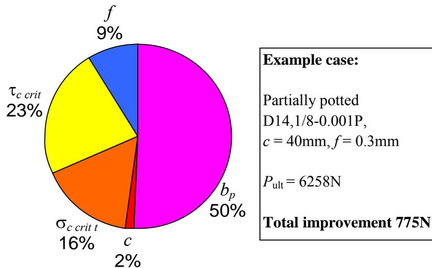
**Figure 12-3: Out-of-plane capability: Contributions of the main components on improved core tension**
