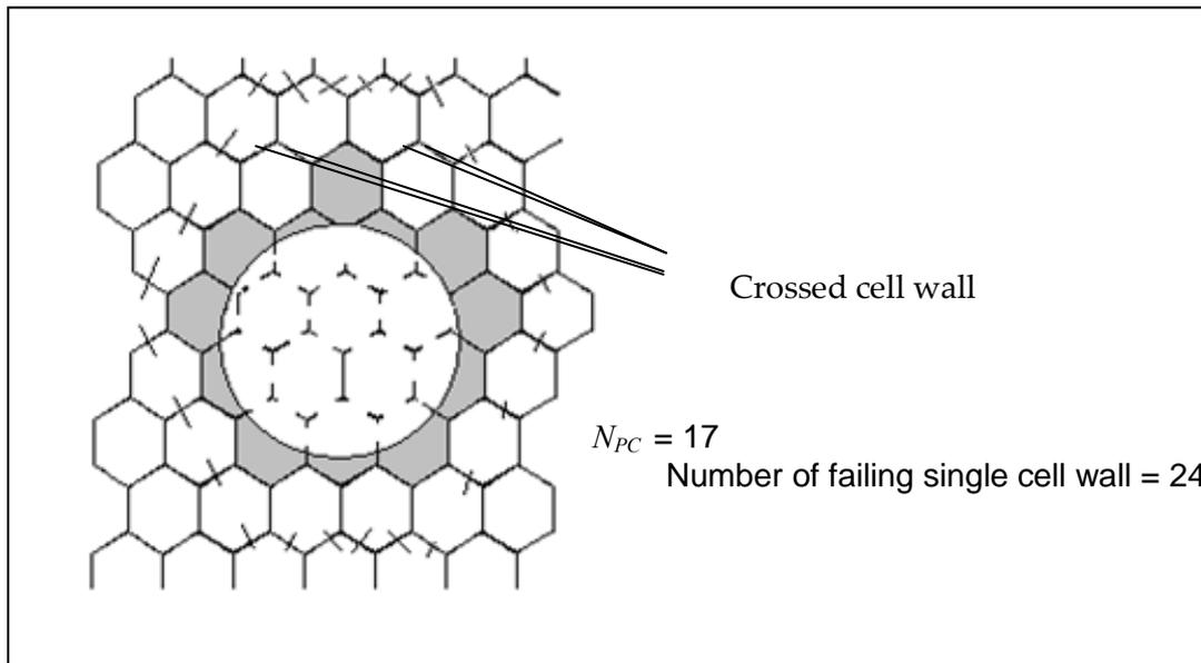
**Figure 10-18: Failure modes: Unsymmetrical potting and crossed cell**
