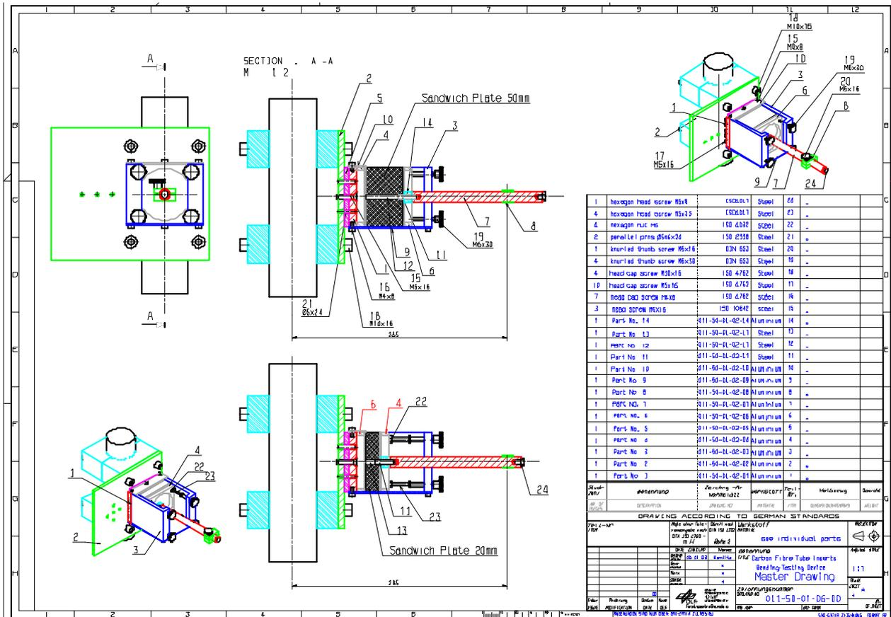
Figure H-18: Test fixture: Bending – master drawing
