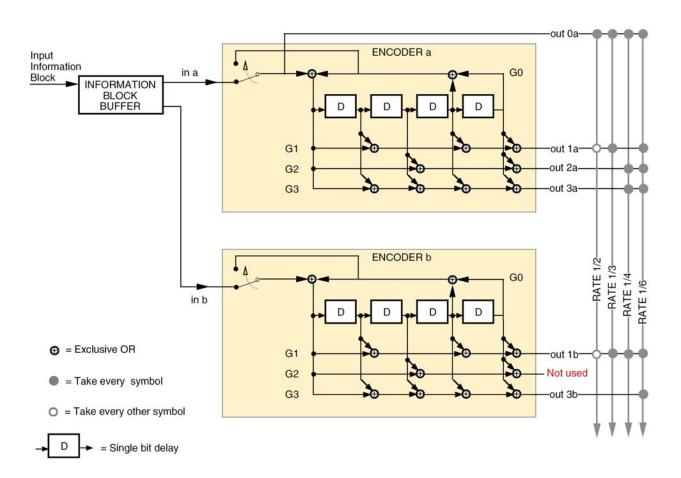
Figure 7-2: Turbo encoder block diagram
