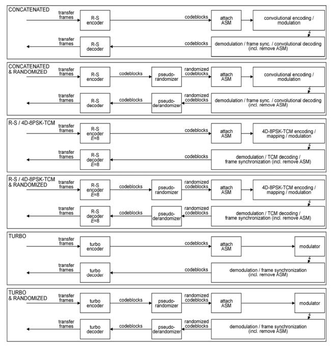
Figure 4-2: Coding, randomization and synchronization (2)
