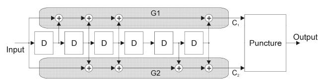
Figure 5-2: Punctured encoder block diagram
