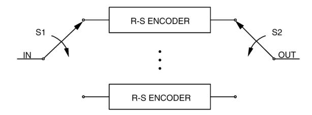
Figure 6-1: Functional representation of R-S interleaving
