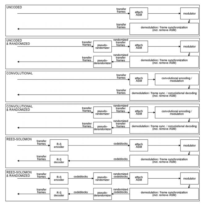
Figure 4-1: Coding, randomization and synchronization (1)
