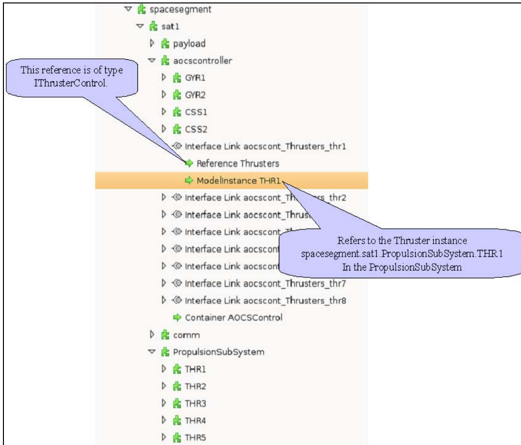
Figure 8-18: Defining Interface-Links From AOCSController to the Thrusters
