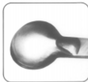
Unacceptable Excessive solder
