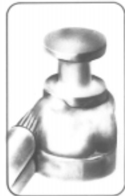
Unacceptable Excessive solder
