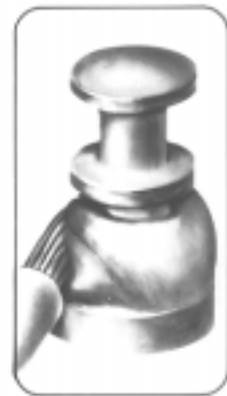
Unacceptable Excessive solder
