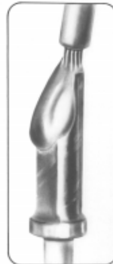
Unacceptable Excessive solder
