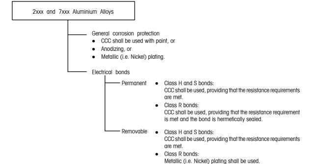
\* Class S bond: resistance less then 1,0  $\Omega$  Class H bond: resistance less then 0,1  $\Omega$  Class R bond: resistance less then 0,0025  $\Omega$
